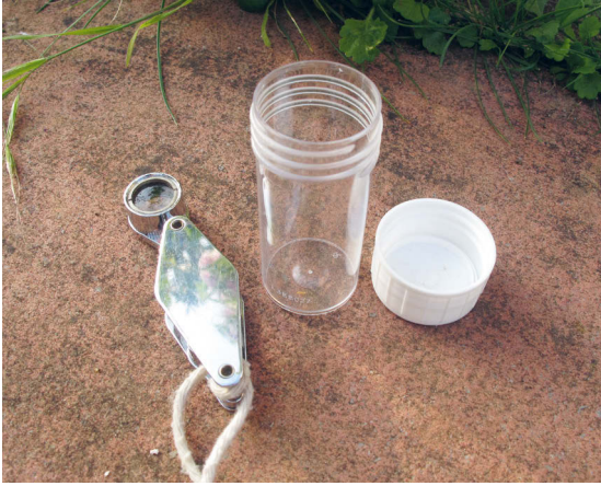
◀ Field survey equipment: x10 hand lens and small collection pot.
