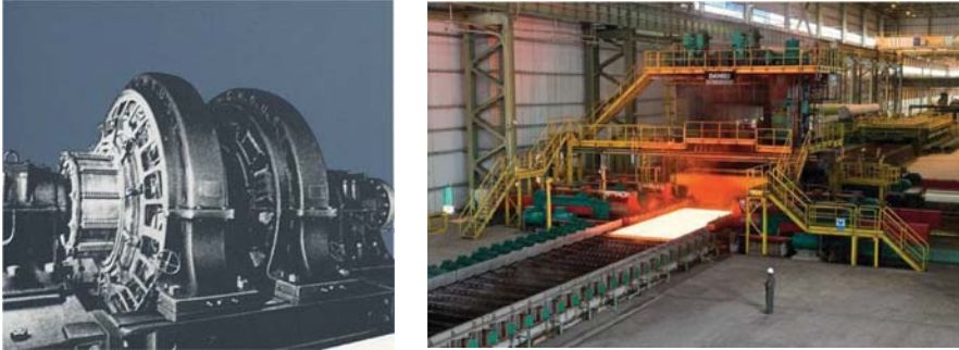
FIGURE 6.1 First rolling mill motor by Westinghouse Company and a rolling mill producing steel slabs by the company Danieli.
