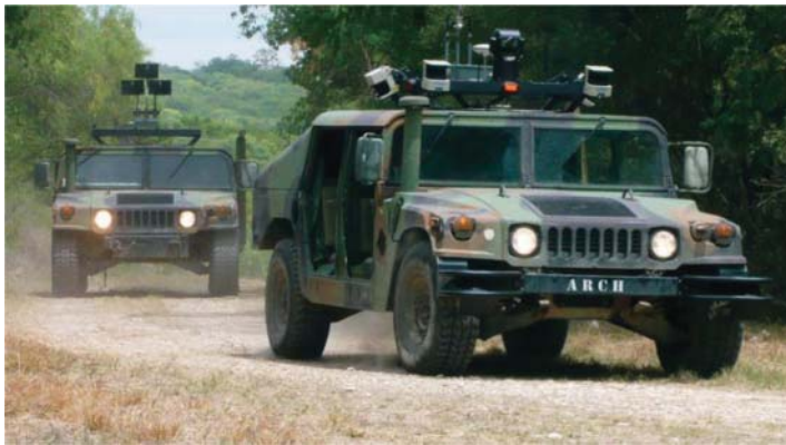
Figure 1.20 The autonomous remote controlled HMMWV, ARCH . Created by students directed by Dr. Alfred Wicks of Virginia Tech and researchers from TORC, www.torc.tech.com .
