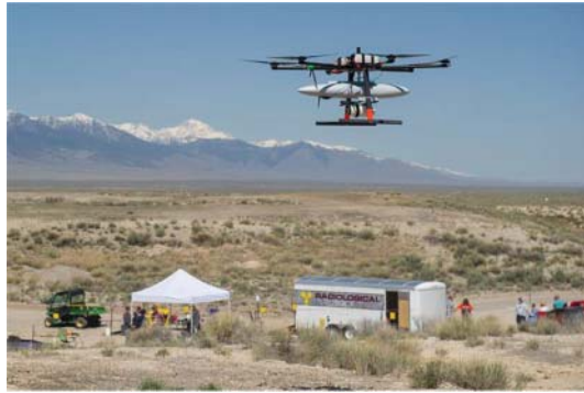
Figure 1.21 Autonomous rotorcraft for radiation sensing. Created by students under the direction of Professor Kevin Kochersberger of Virginia Tech.
