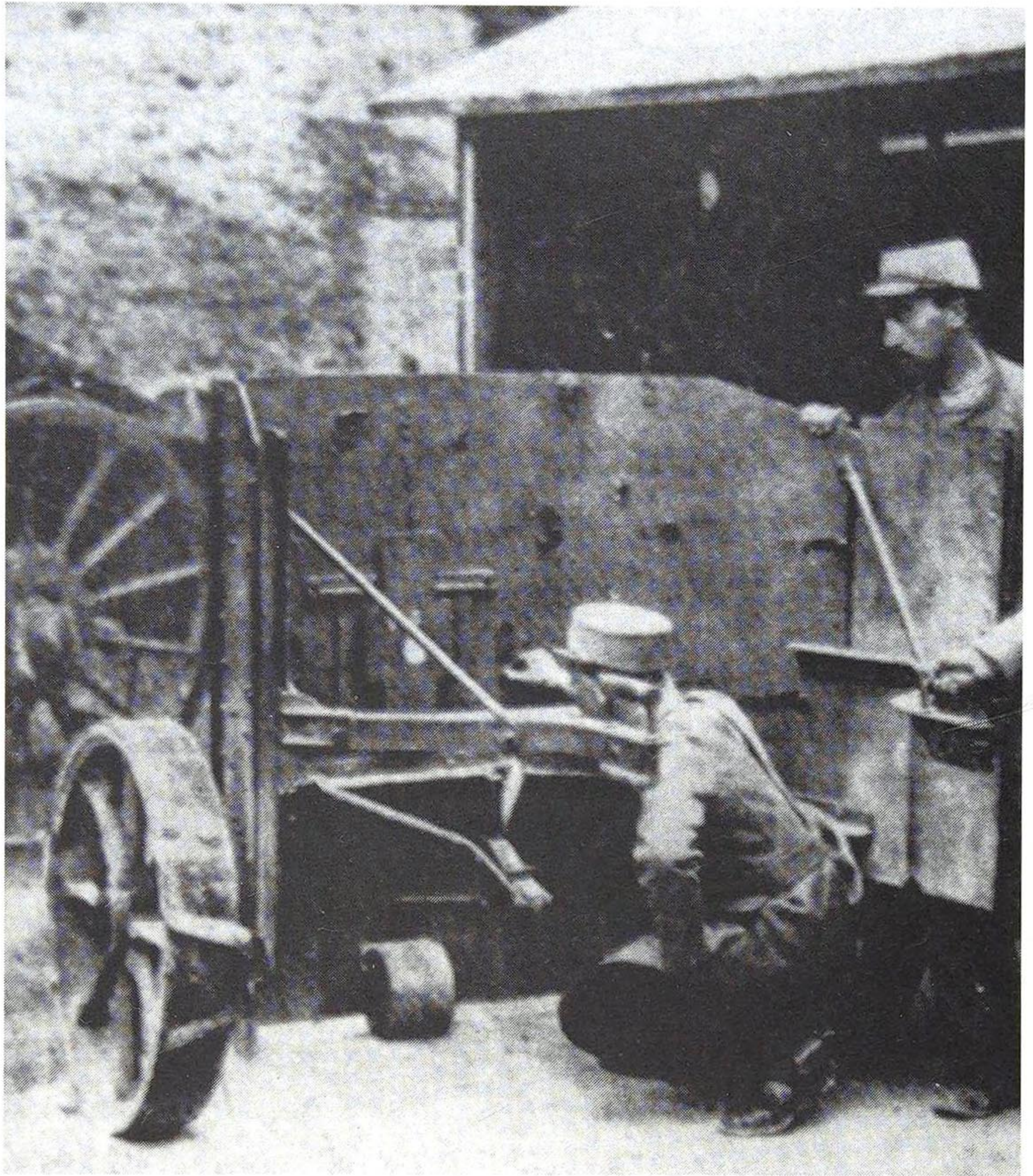
French wheeled shield with side plates, propelled by muscle power. (The Times History of the War)
