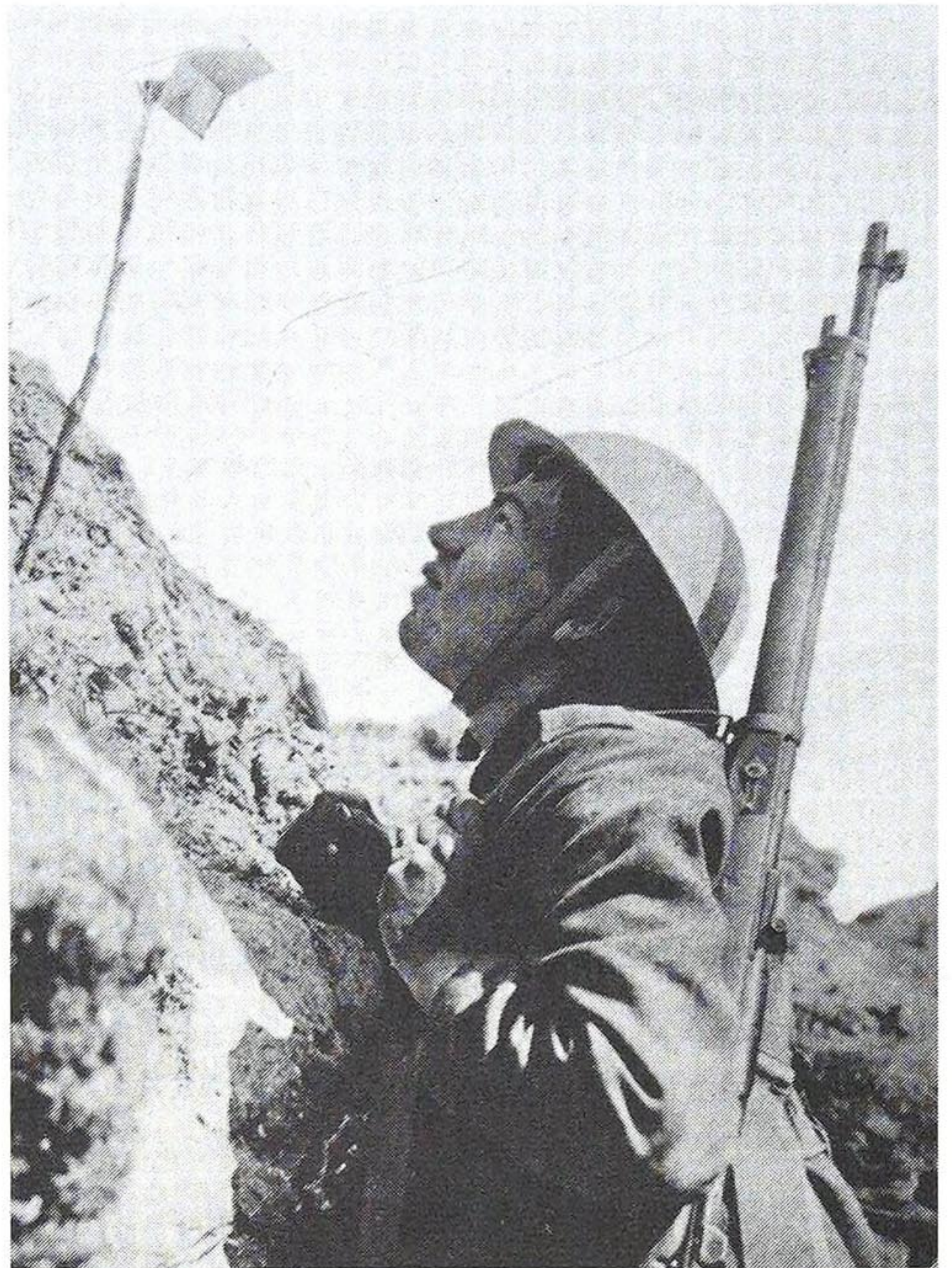
The simplest ‘periscope’ was a single mirror with a shade. This one is attached to a stick stuck into the parados. (The Illustrated War News)
