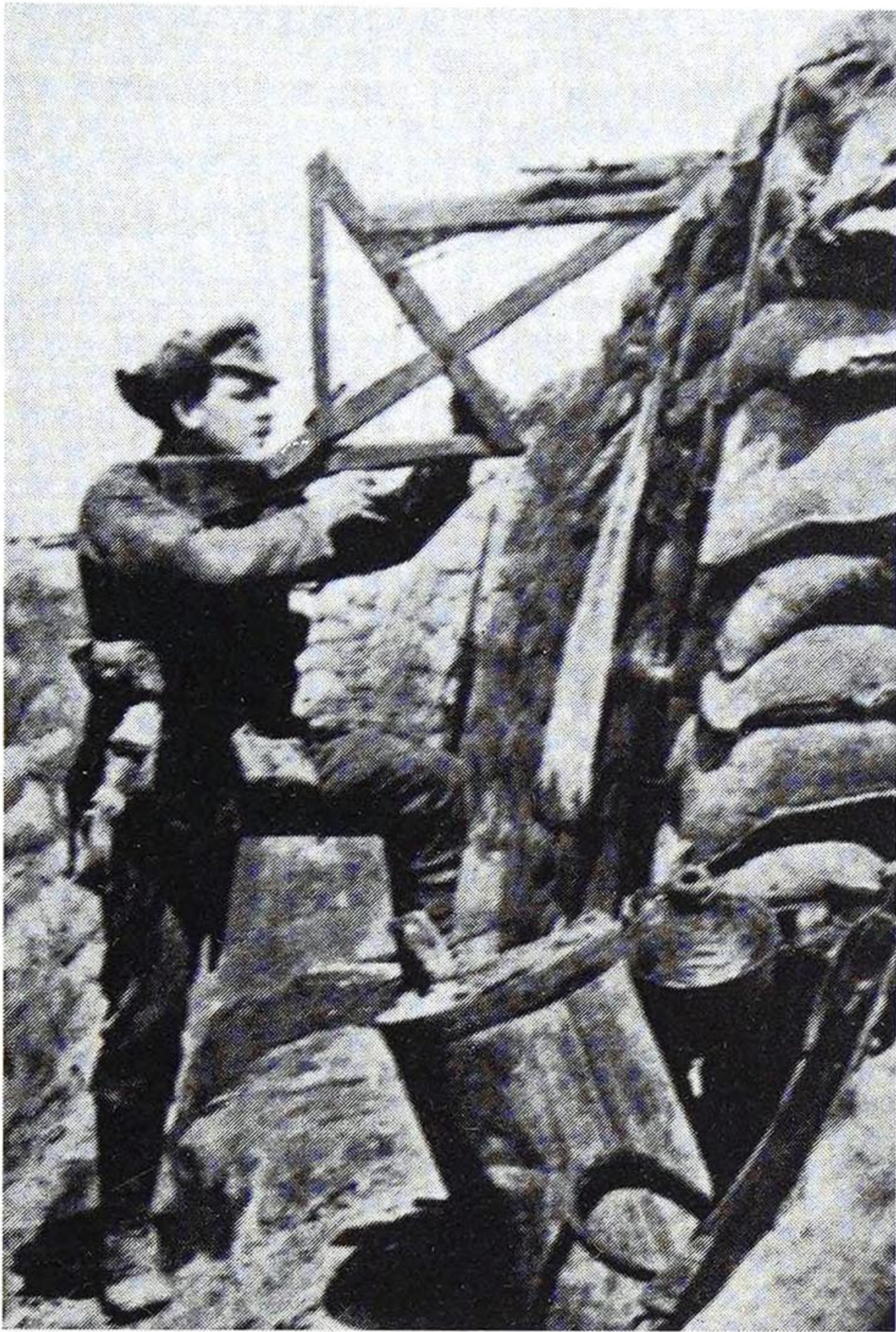
A British sniperscope designed and made by Royal Engineers, 1915. This simple device was made in large numbers throughout the war. Although it has an auxiliary trigger, there is no bolt-operating mechanism. (The Times History of the War)
