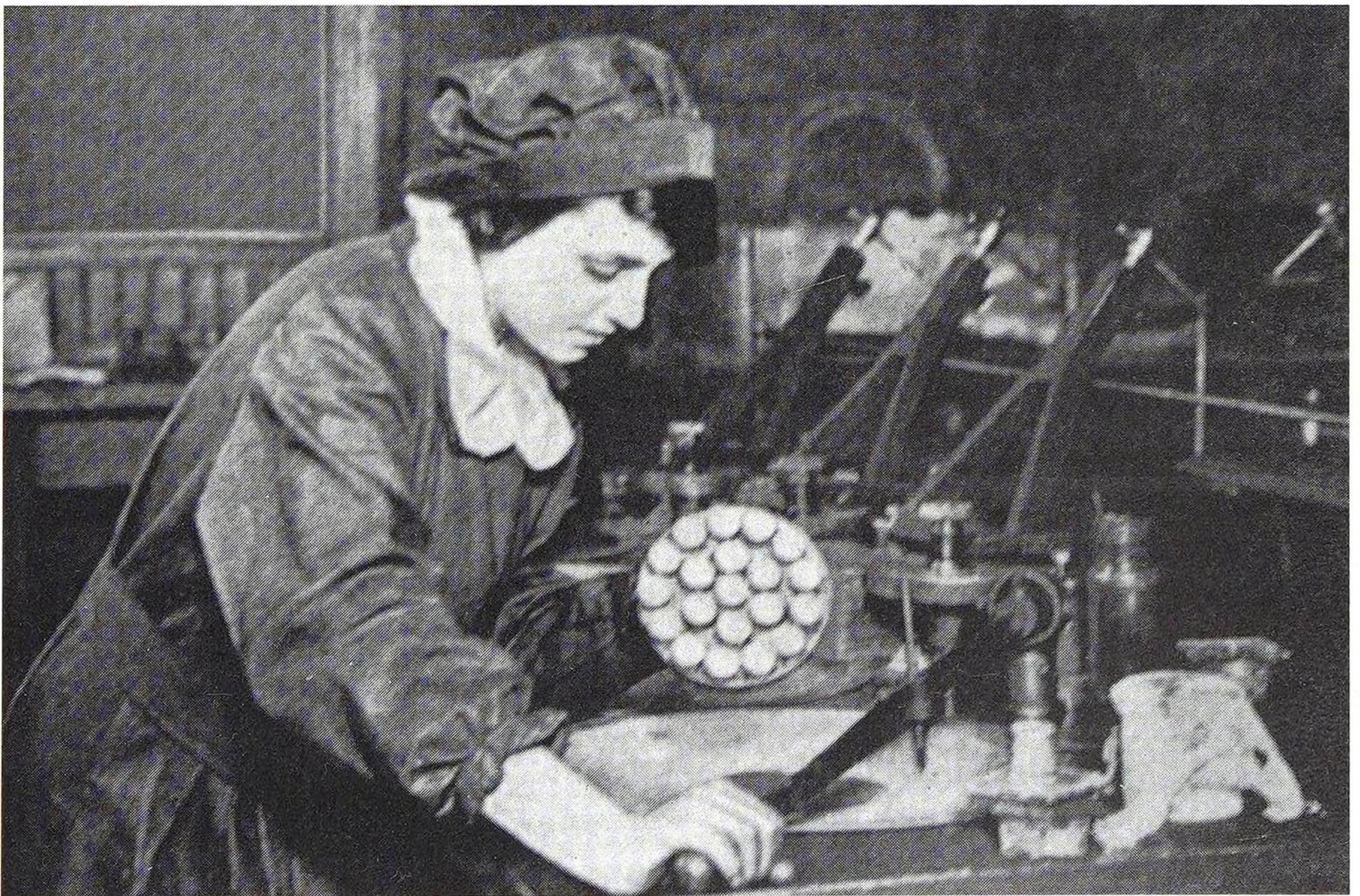
Learning how to make lenses at the Northampton Institute. This worker is polishing twenty lenses. (The Illustrated War News)
