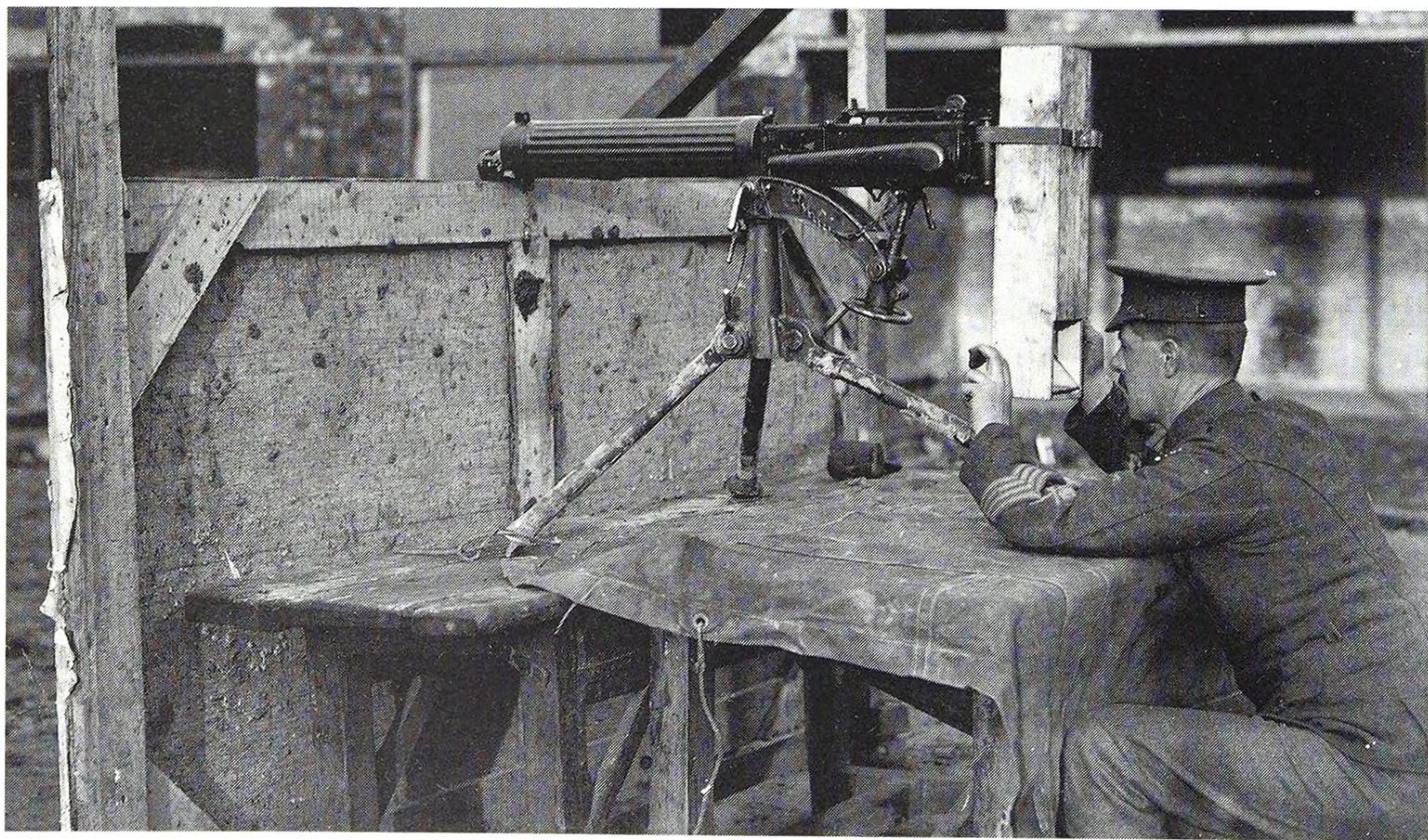
The GHQ-pattern machine-gun hyposcope. A metal band fixes the device to the gun's spade grips. The operator is resting his hands on the auxiliary trigger. (IWM)
