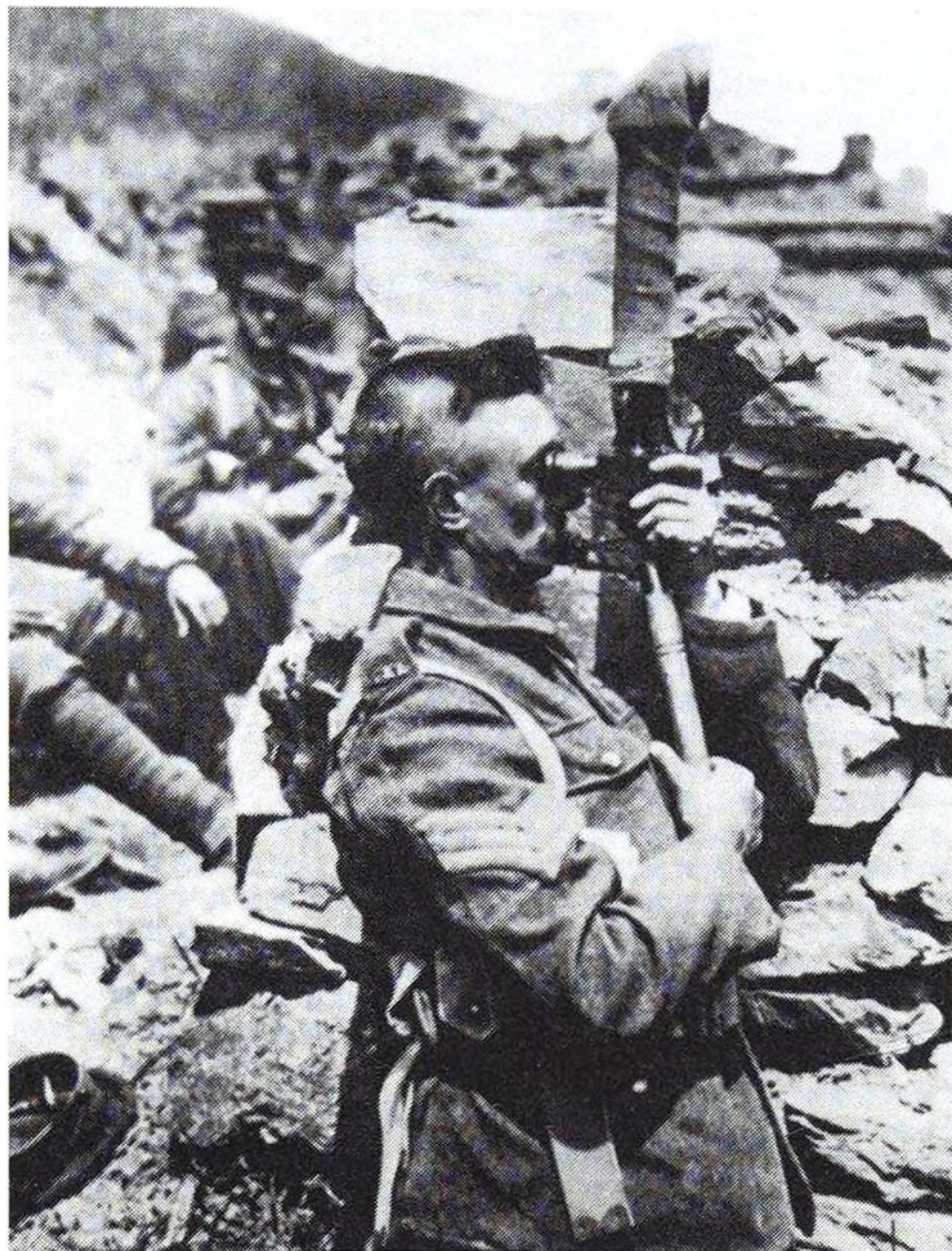
An artillery observer at Salonika in early 1916, using a camouflaged magnifying periscope fitted with a wooden handle, possibly the No. 14. (The Illustrated War News)
