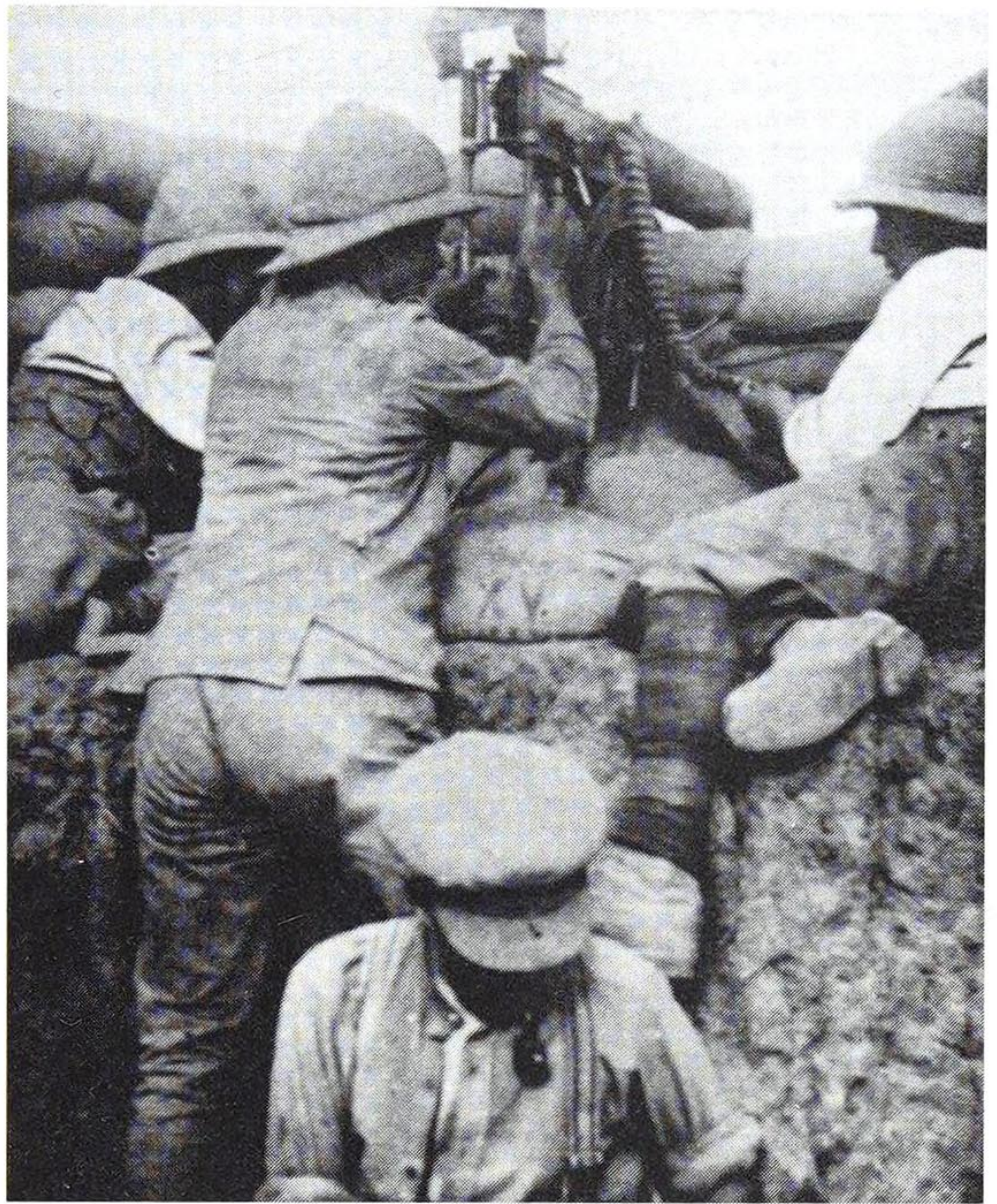
One of William Youlten's machine-gun hyposcopes fitted to a Vickers in the Dardanelles, late 1915. It has two mirrors; the lower mirror is just above the crook of the shooter's right arm. The gun's trigger is operated by an auxiliary depressed with the thumb. (The Illustrated War News)
