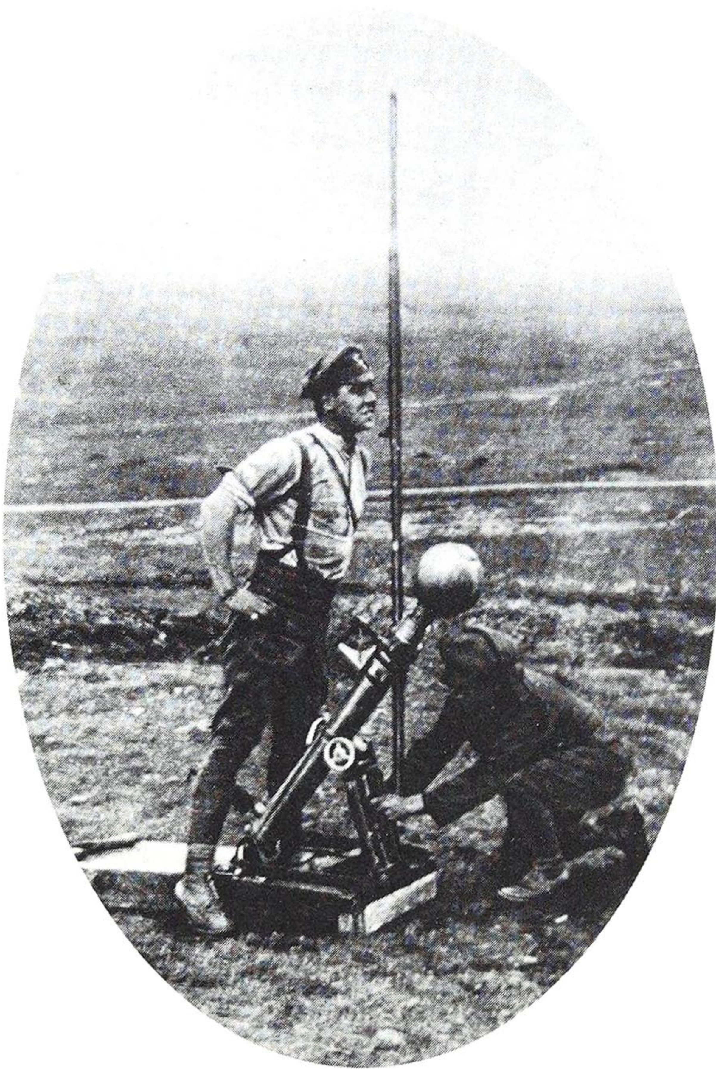
The 2 in toffee-apple mortar fitted with the No. 4 Mk II periscope. (The Illustrated War News)
