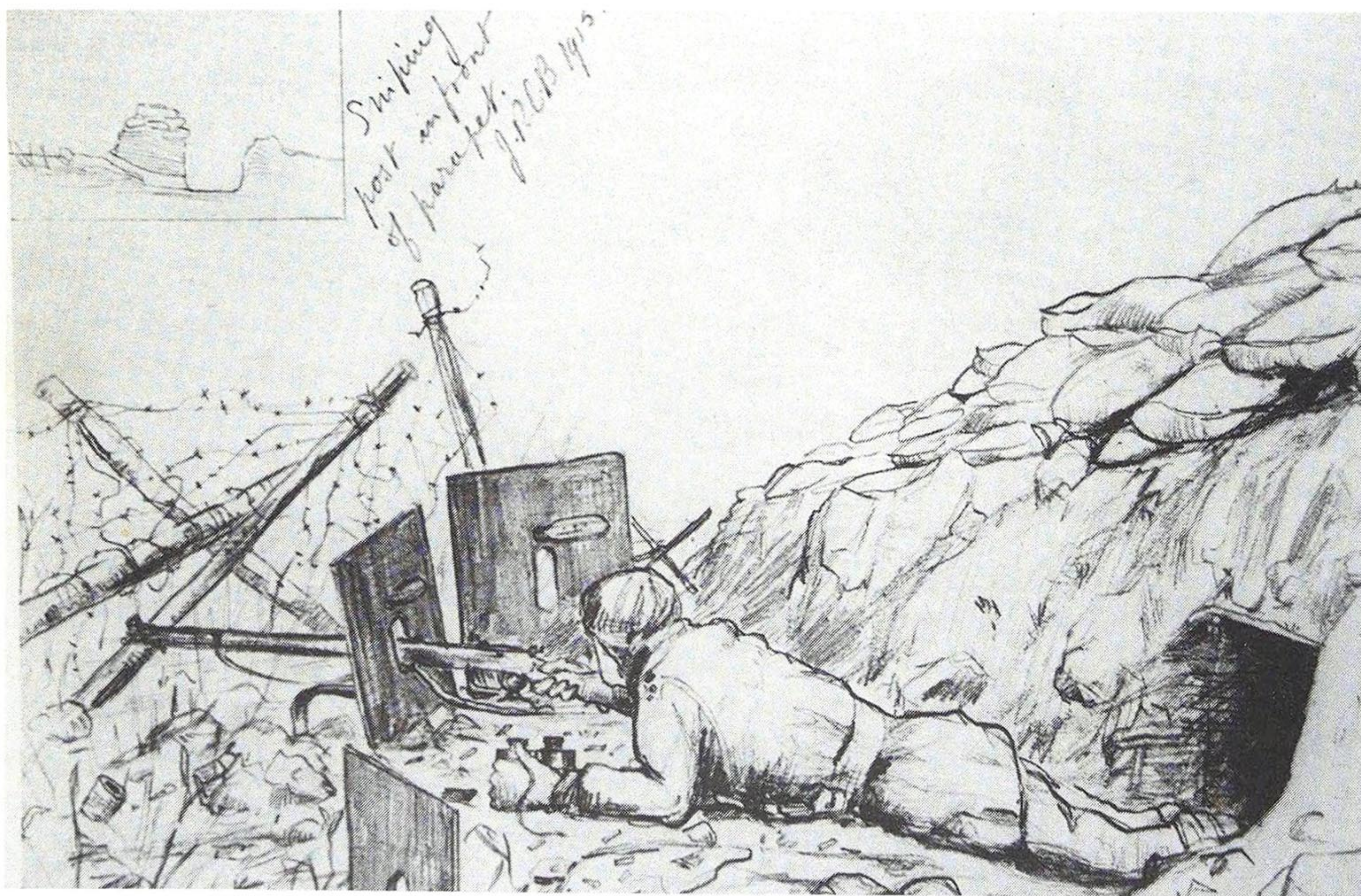
Sketch of British sniper in 1915 with three sniping plates set up in front of the parapet, each of which has a shuttered loophole; note that the shutter is on the inner face. Note also the supporting leg on the front of the central shield. (The Illustrated War News)
