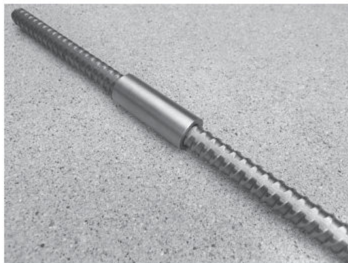
Picture of #7 GR75 Dywidag THREADBAR (R) reinforcing bar including a couple for transferring tension loads.
