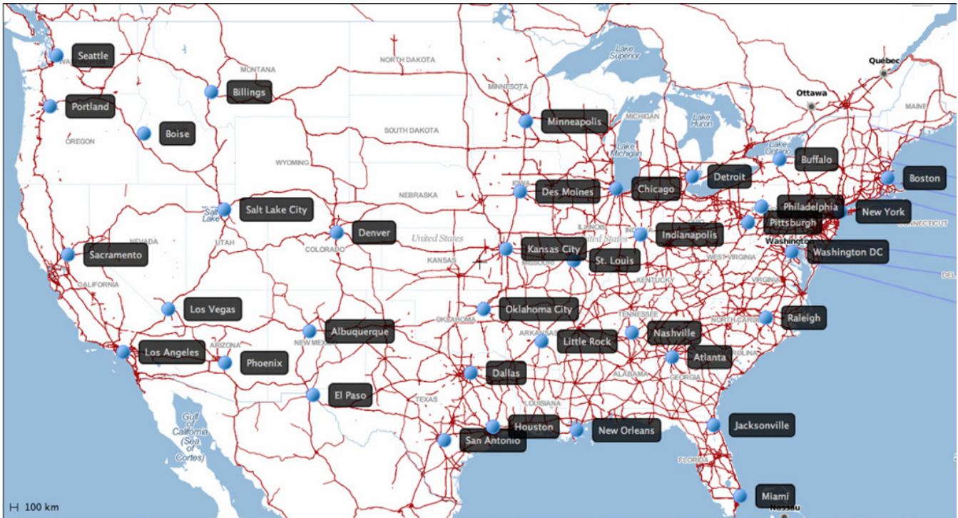
FIGURE 5.4 Major carrier hotels within the United States form the backbone of telephony and Internet service.
