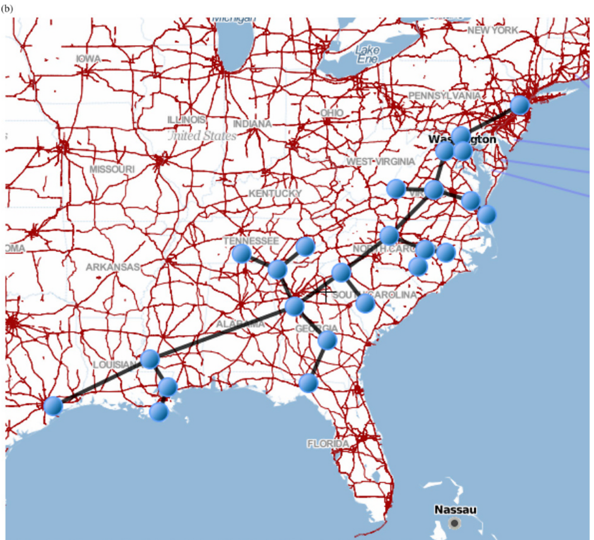
FIGURE 12.7 Refined petroleum products flow from the Gulf of Mexico oil field and LOOP terminal to refineries along the Gulf Coast and then to consumers in the Northeast by way of the Colonial pipeline and storage network. (a) Gulf of Mexico network of oil fields and refineries. LOOP is circled. (b) Colonial pipeline connecting refineries to markets in the Northeast. http://www.shellpipeline.com/cd_maps/SPL403_D_gc_crude_f.pdf .
