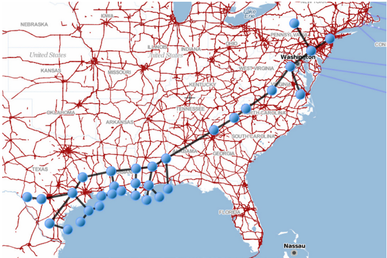
FIGURE 12.14 The 10,600-mile Transco Pipeline carries liquid natural gas (LNG) from fields along the Gulf of Mexico and ports along the East Coast to markets in the Northeast.
