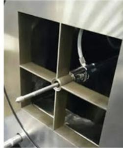
(c) Diaphragm rupture device
