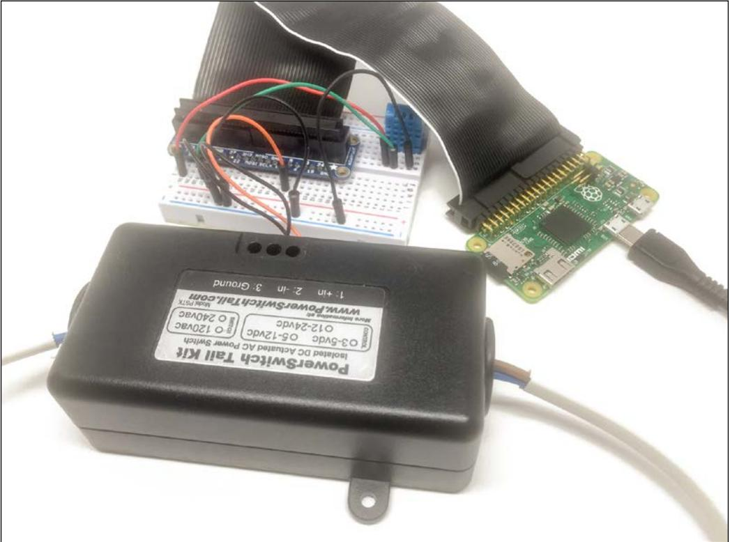
Finally, plug the heater into the PowerSwitch Tail and connect the PowerSwitch Tail to the mains electricity.
