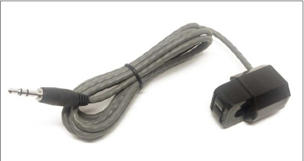
The advantage of this sensor is that you don't need to cut anything to measure the current flowing in the device. To use this sensor, and convert the current it measures to a voltage we can measure, you'll also need a 10-Ohm resistor.
