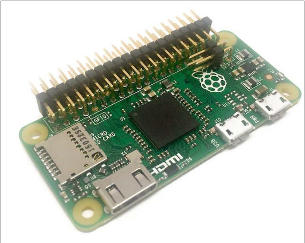
In the center of the board, you will find the same **System-on-a-Chip (SoC)** as the original Raspberry Pi board, with a 1-GHz single-core processor, 512 MB of RAM, and a graphical processing unit.
