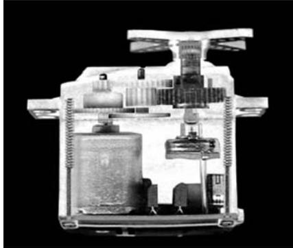
**FIGURE 7.1** Inner view of a standard R/C servo motor.
