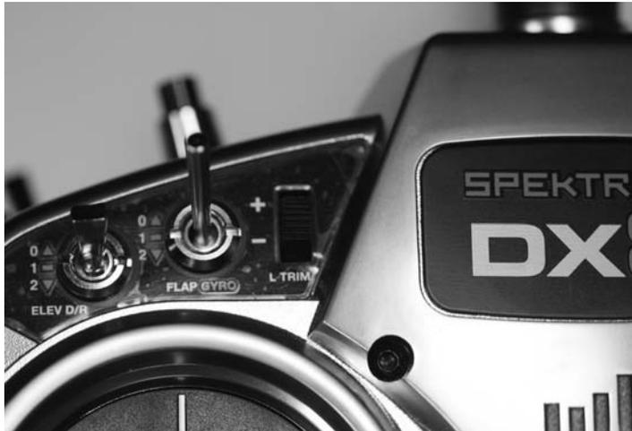
FIGURE 7.19 DX-8 Aux-1 (Flap) switch.
