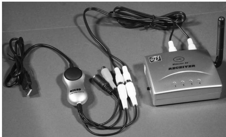
**FIGURE 9.23** RC310 receiver and an EzCap USB video-capture module.
