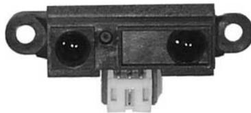
**FIGURE 11.22** Sharp GP2D12 IR range sensor.
