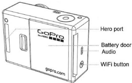
FIGURE 9.3 Diagram of a Hero 3 camera back.
