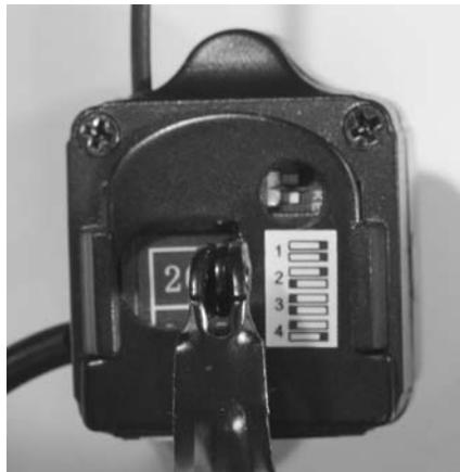
**FIGURE 9.24** RC310 camera frequency selection switches.
