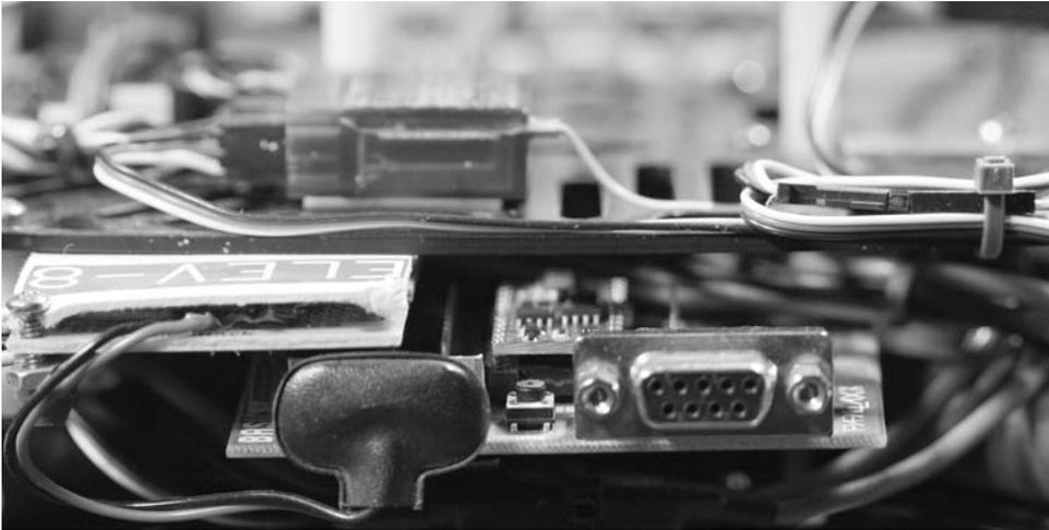
**FIGURE 7.18** Early version of an Elev-8 LED-lighting controller.
