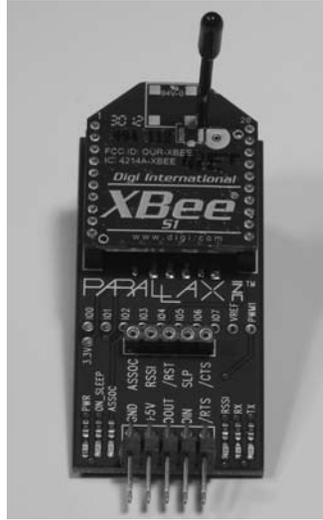
**FIGURE 8.15** Parallax XBee SIP Adapter.
