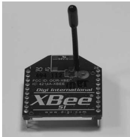
**FIGURE 8.14** XBee Series 1 transceiver.
