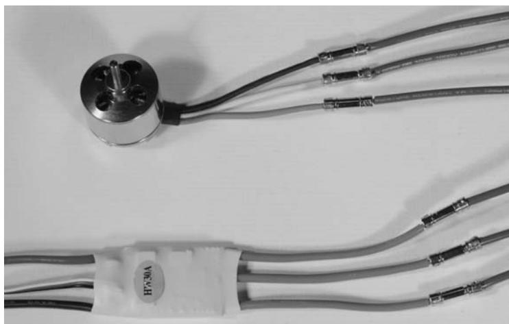
**FIGURE 3.19** Wire extensions connected to an ESC and motor.
