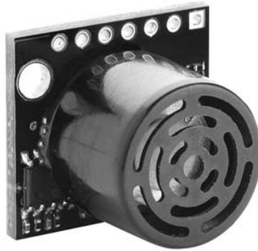
**FIGURE 11.20** The MaxBotix HRLV-Max Sonar® – EZ1™, model MB1013.
