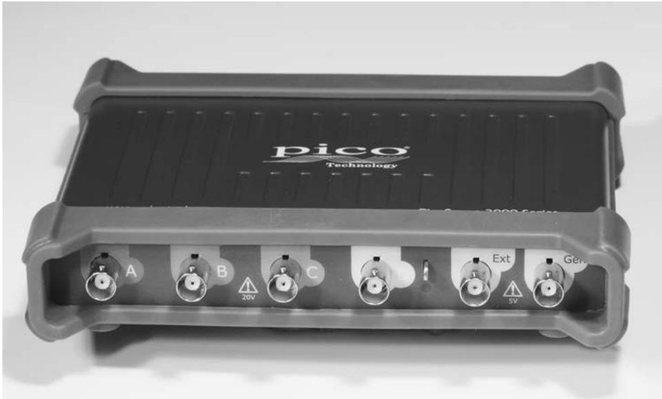
**FIGURE 4.17** Picoscope Model 3406B USB oscilloscope.
