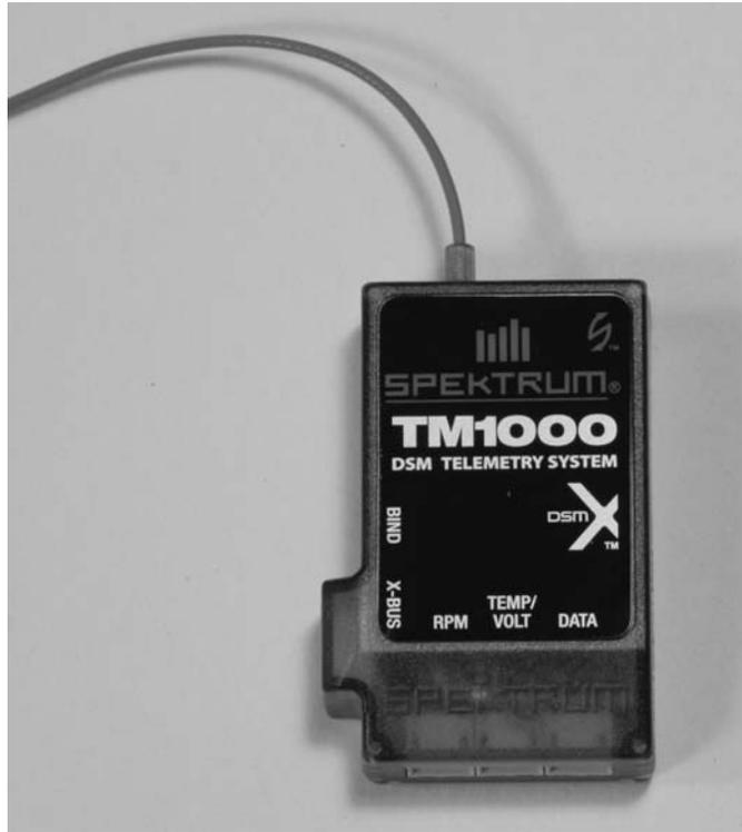
**FIGURE 3.13** Spektrum 1000 telemetry transmitter.
