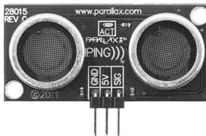
FIGURE 11.14 Parallax Ping sensor.
