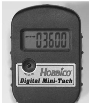
**FIGURE 5.20** Optical tachometer.
