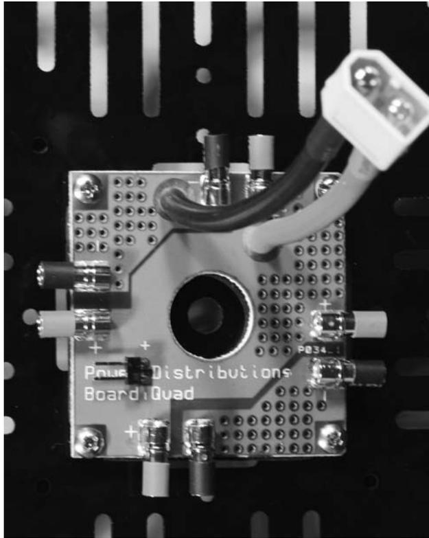
**FIGURE 3.26** The installed quad power-distribution board.
