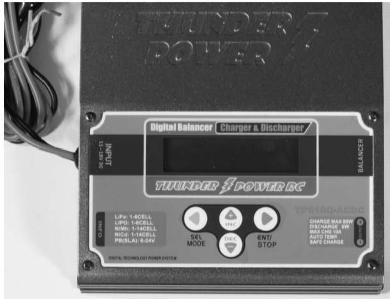
**FIGURE 3.10** Automatic LiPo battery charger.
