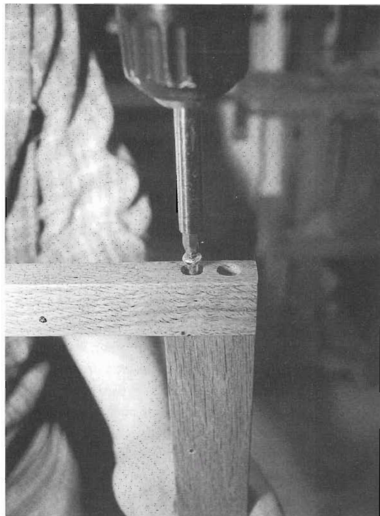
Fig. 1-21 The face frame can be butt joined using the same PCB screws.
