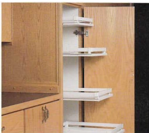
Pull-out shelves are a combination of shelves and drawers. Instead of searching through a stack of pots and pans in your lower cabinets, just slide out the shelf and pick what you need. Build your own using drawer slides.
