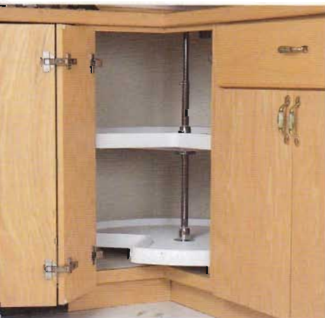
Utilize wasted corner space by installing a lazy susan. In upper cabinets, use a regular corner cabinet with 170° full-overlay hinges.
