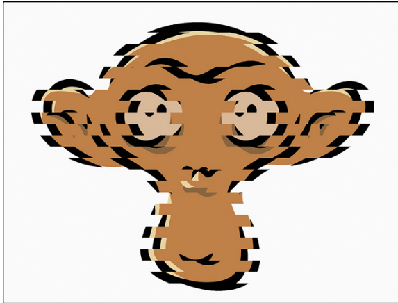
FIGURE 19-2: An interlaced frame is assembled by interleaving neighboring frames in captured footage.
