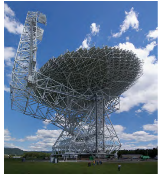
Figure 7.1. A telescope’s resolving power is related to its aperture and the wavelength of light to which it is attuned. A radio telescope, which observes very long wavelength light, must have a very large aperture to resolve details.
