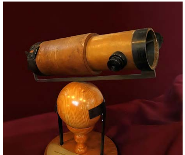
Figure 4.6. A replica of Newton’s reflecting telescope. A curved mirror is placed on the opposite (left) end as the opening where the light enters. This mirror then directs the light up to a flat mirror near the opening, which redirects it to a focus through a hole, drilled in the side of the telescope tube. An eyepiece can then be placed there to observe the image.
