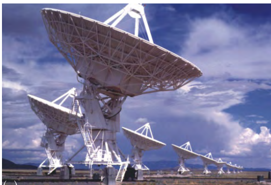
Figure 7.7. Light signals from multiple telescopes can be combined through interferometry to increase the resolution of the image, as is done at the Very Large Array (left) and the Very Large Telescope Interferometer (right). VLT image courtesy of NRAO/AUI. VLT image courtesy of ESO/H.H.Heyer.
