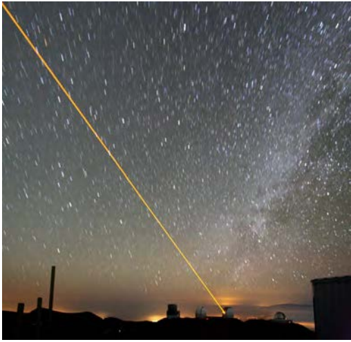
Figure 7.8. By using artificial stars created by lasers, astronomers can measure the atmosphere's effects on an image and subtract it out in a process called adaptive optics. Many of today's modern telescopes, like the two Keck telescopes and the Subaru telescope shown here, are outfitted with these systems to provide images with remarkably high resolution.
