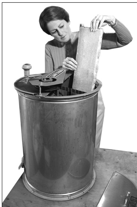
FIGURE 17-7: Place the uncapped frame vertically in the extractor.
