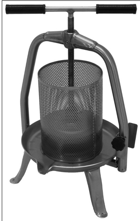
FIGURE 17-9: This is one style of honey press that is used for extracting honey from Top Bar hives.
