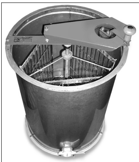
FIGURE 16-1: This hand-crank, stainless-steel extractor extracts up to six shallow frames at a time.
