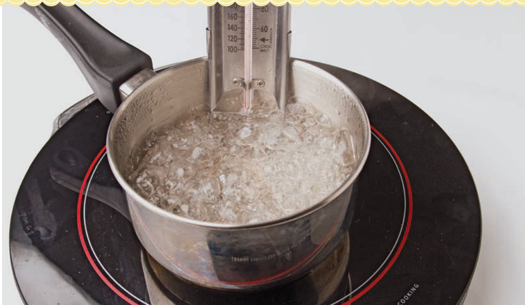
Testing a thermometer in boiling water
