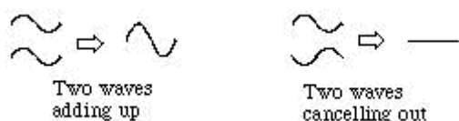
Figure 5: Unlike two particles, two interfering waves can either add up or cancel out.
