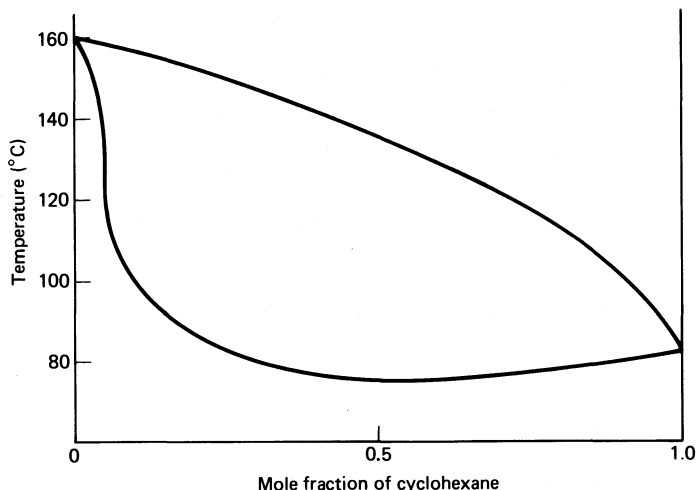
Fig. 146 Other deviant behavior (but no azeotropes) in the furfural-cyclohexane system.
