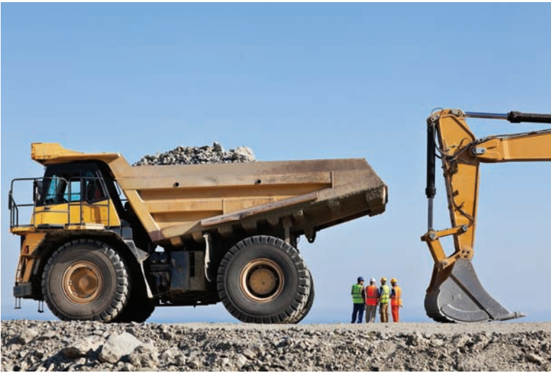
Fig. 2-9 An off-highway truck used for moving earth. Note its size in comparison with the worker. © Martin Barraud/Getty Images
