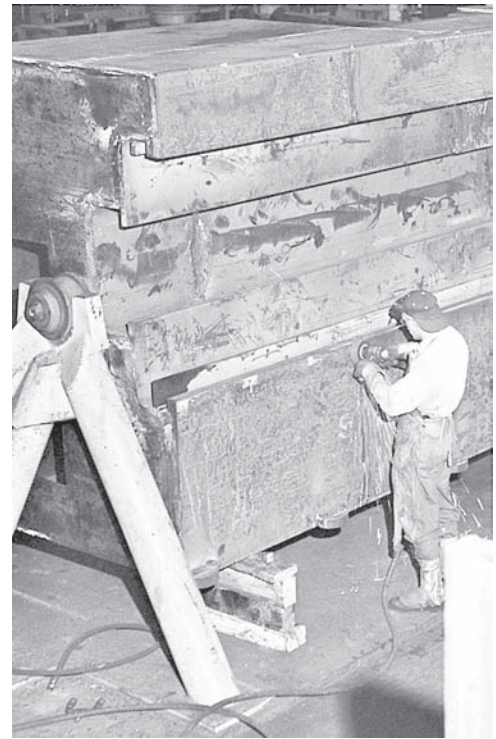
Fig. 2-15 A mechanic grinding welds on the bed of the profiler shown in Fig. 2-13. © MAG IAS, LLC
