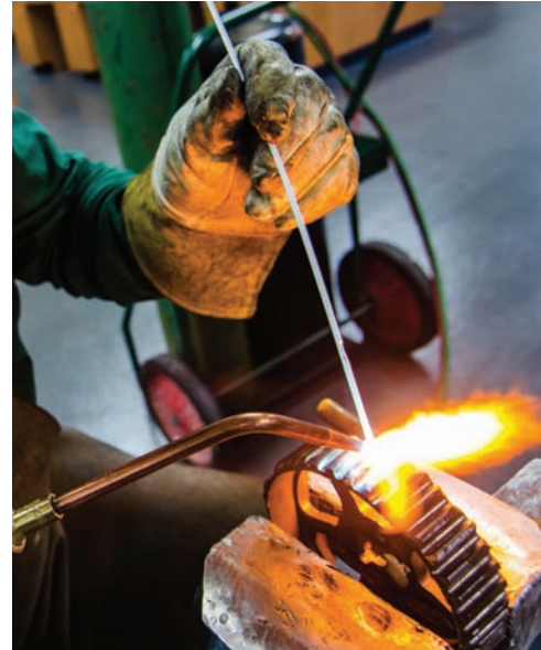
Fig. 9-2 Building up a gear tooth with bronze in a series of layers, each of which is about \frac{1}{16} -inch thick. A flux coated brazing rod is being used. Location: Northeast Wisconsin Technical College © McGraw-Hill Education/Mark A. Dierker, photographer
