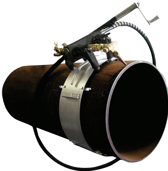
Fig. 16-86 Band-type cutting and beveling machine cuts out-of-round pipe. © Mathey Dearman
