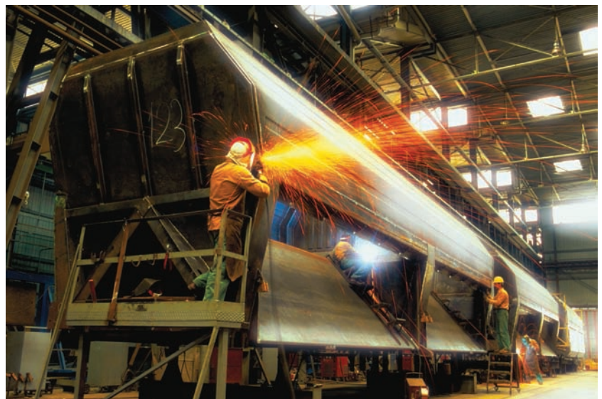
Fig. 2-13 Several rail cars in various stages of completion. Note the size of this fabrication area. Air carbon arc gouging is being used, as well as many of the typical arc welding processes like GMAW and FCAW. © Alberto Incrocchi/Riser/Getty Images
