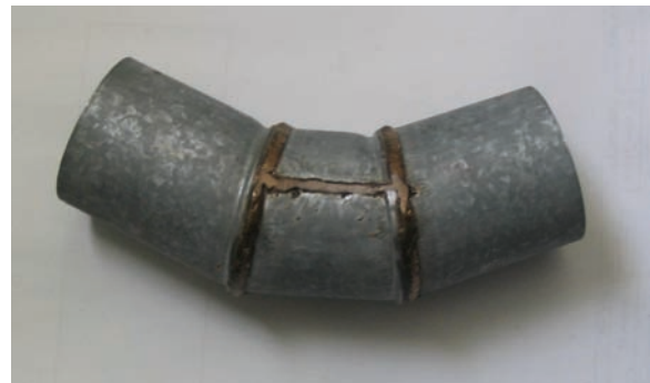
Fig. 21-15 Silicon bronze applied to a 22-gauge galvanized steel pipe elbow using the GMAW-B process. © Wisconsin Wire Work
