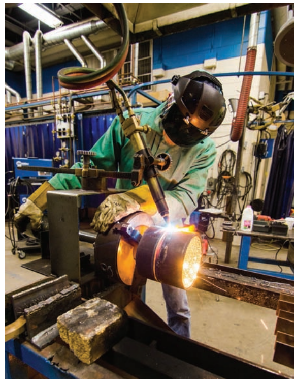
Fig. 7-12 A welding student is beveling pipe with a shop-built beveling machine. Location: Northeast Wisconsin Technical College © McGraw-Hill Education/Mark A. Dierker, photographer
