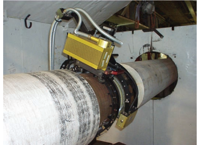
Fig. 16-44 Real-time radiographic inspection of pipeline welds. Digital X-ray technology has advanced to becoming truly real time and in high resolution. Utilizing advanced X-ray detector technology and pipeline-specific software, the inspection process has become a replacement for conventional RT. A typical pipeline crawler is used inside the pipeline, but externally the film is replaced by an RTR scanning mechanism that runs on a typical band. © Shaw Pipeline Services
