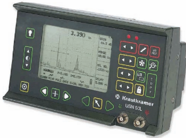
Fig. 28-43 Portable ultrasonic weld flaw detector with built-in trigonometric flaw location calculations with curvature correction and AWS D1.1 weld rating calculations. It combines a phased array imaging device and a conventional flaw detector into one instrument, with a phased array probe that allows significantly increased confidence in inspection data. Compared with traditional thickness gauge and flaw detector inspection, it offers greater probability of detection as well as faster and more reliable scanning. (left) © Agfa Corporation; (right) © General Electric Company
