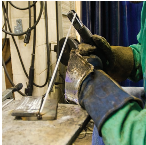
Fig. 13-33 Welding lap joints in the flat position. The electrode and electrode holder are positioned as instructed in Fig. 13-32. Location: Northeast Wisconsin Technical College © McGraw-Hill Education/Mark A. Dierker, photographer
