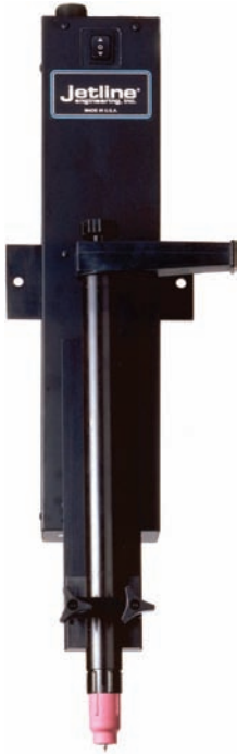
Fig. 27-8 Automatic voltage control drive unit. It features a stepper motor driving a precision lead screw to provide the motion. It is filtered against high frequency and has minimal play and backlash. Manual up and down jog buttons are provided on the side of the unit. © ITW Jetline - Cyclomatic
