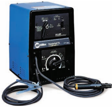
Fig. 11-16 A simple SMAW welding machine with mechanical control of the welding output. This hand lever permits continuous control of current. © Miller Electric Mfg. Co.
