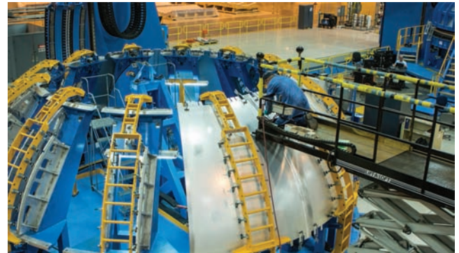
Fig. 2-3 Welded jigs and fixtures are used with various welding processes. In this case they are being used for a friction stir weld on an orange peel section of an end cap for a large aluminum fuel storage vessel. NASA
