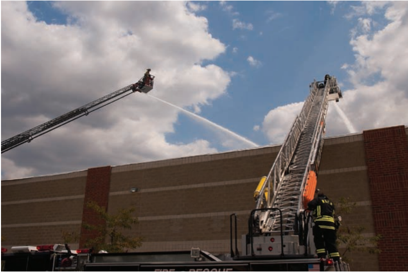
Fig. 2-7 Note the two water cannons being used to fight this fire. One is also equipped with a basket the fire fighters can use to rescue people. Light-weight aluminum is extensively used and welded to accommodate this type of service. © McGraw-Hill Education/Mark A. Dierker, photographer
