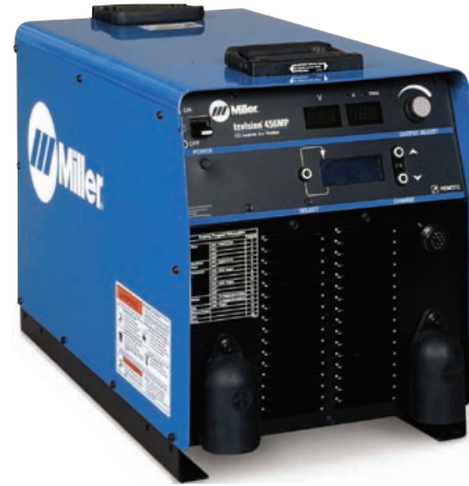
Fig. 11-18 A 450 amp d.c. inverter power source. This machine is equipped with a micro processor to control the various process output capability. © Miller Electric Mfg. Co.
