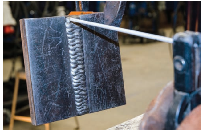
Fig. 13-72 Welding beads in the vertical position, travel up. The electrode and electrode holder are positioned as instructed in Fig. 13-70. Location: Northeast Wisconsin Technical College © McGraw-Hill Education/Mark A. Dierker, photographer
