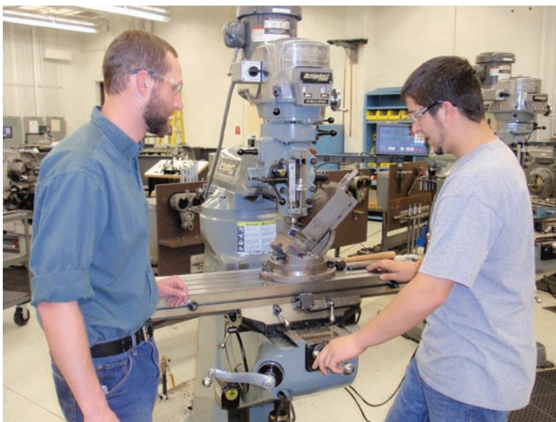
Fig. 26-72 Instructor observing student using a vertical milling machine. Gloves are not used around machine tool operations where they could get caught up in the moving equipment. © Renee Bohnart
