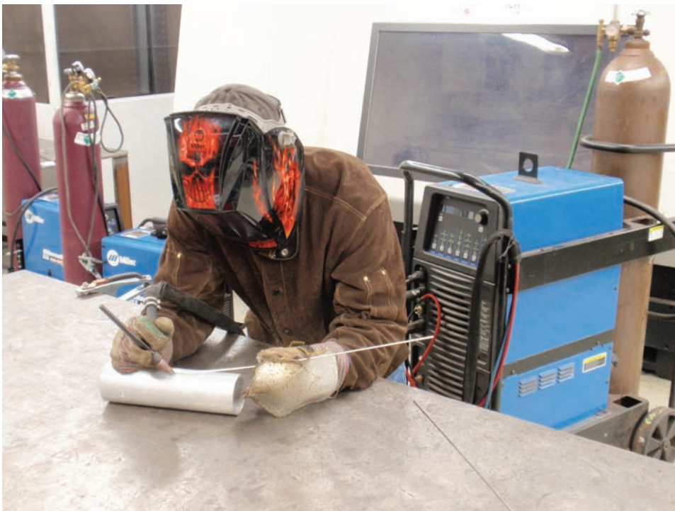
Fig. 20-2 Welding on aluminum pipe, in the 1G pipe rotated position. The welding machine is a 300-ampere a.c.-d.c. enhanced square wave GTAW power source. © Renee Bohnart
