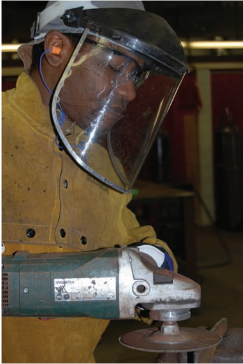
Fig. 26-57 A welding student using an electric side grinder. This type tool is very helpful for dressing weld profiles, removing weld defects or in this case joint preparation. Note the ear plugs, gloves, and double eye protection. © Renee Bohnart
