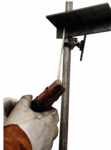
Fig. 15-7 Electrode and electrode holder positioned as instructed in Fig. 15-6. Note how the joint is held by the jig. © Edward R. Bohnart
