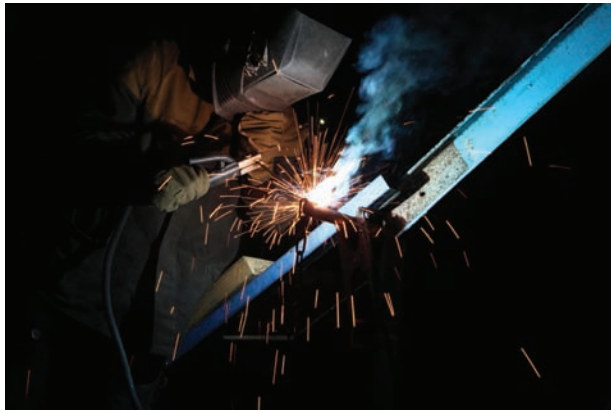
Fig. 13-1 A young welder who has completed training is welding a steel fabrication on the job with the shielded metal arc welding process. © VPC Travel Photo/Alamy Stock Photo
