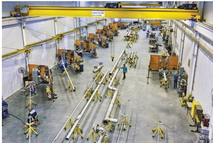
Fig. 26-20 A well-organized bay setup for welding stainless steel pipe. It is critical when working with certain alloys like stainless steel to segregate them so cross contamination does not take place. Note each work cell with its own positioner and overhead crane for material handling operations. © Team Industries, Inc.
