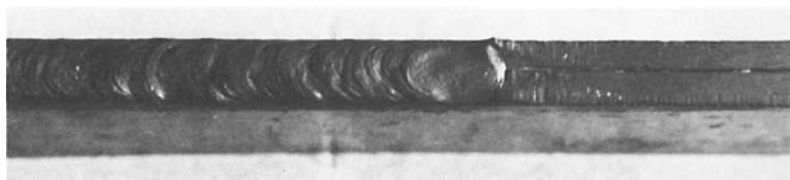
Fig. 13-29 Typical appearance of an edge joint welded in the flat position with DCEN or a.c. shielded arc electrodes.
