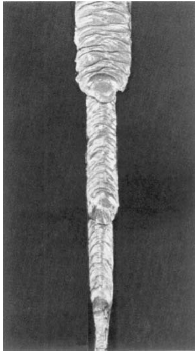
Fig. 14-63 Typical appearance of a multipass single V-groove weld on a butt joint with a backing bar in the vertical (3G) position, travel down, with DCEP or a.c. shielded metal arc cellulose coated electrodes.
