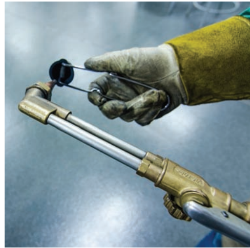
Fig. 7-26 Lighting the cutting torch with a friction lighter. Location: Northeast Wisconsin Technical College © McGraw-Hill Education/Mark A. Dierker, photographer
