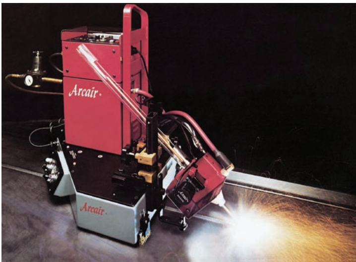
Fig. 17-15 Air carbon arc torch and carriage for mechanized operation. The current is d.c. electrode positive polarity, variable voltage. Electrode sizes are 5/16 through 5/8 inches. © Thermadyne Industries, Inc.
