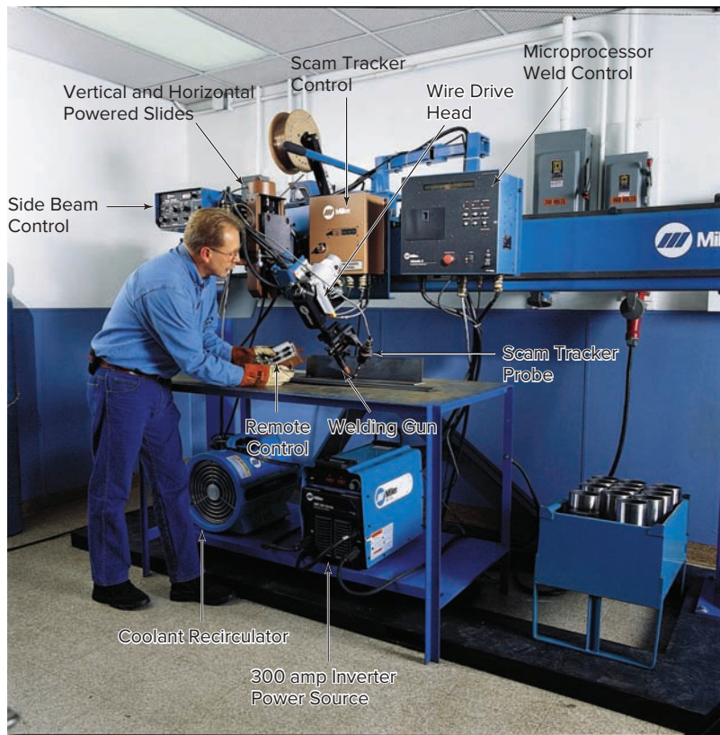
Fig. 27-6 Side beam carriage setup for GMAW with seam tracker and microprocessor weld control. It is using a tactile probe seam tracking system. © Miller Electric Mfg. Co.
