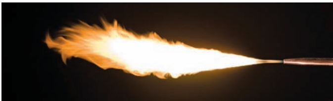
Fig. 8-8 Atmospheric burning of acetylene. Open the acetylene valve until the smoke disappears. © David A. Tietz/Editorial Image, LLC
