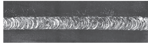
Fig. 8-36 A fillet weld in a T-joint welded in the horizontal position. Stock is \frac{1}{8} -inch plate. A no. 4 tip and \frac{1}{8} -inch mild steel filler rod were used. The flame was neutral.
