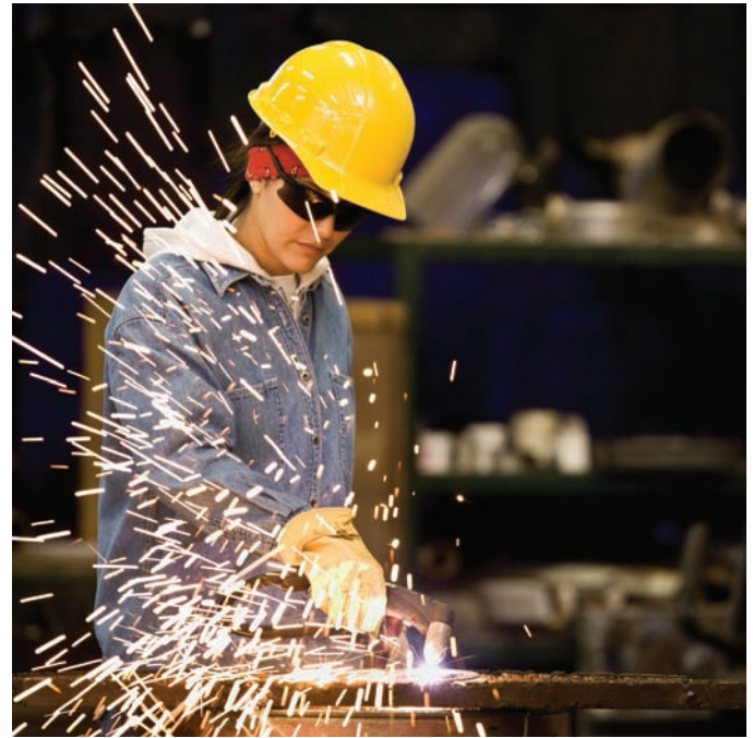
Fig. 1-5 Welding is generally considered a nontraditional occupation for women. However, it can be a very lucrative and in-demand skill for those women choosing this career path. A procedure is being used setting up a plasma arc gouging operation.
