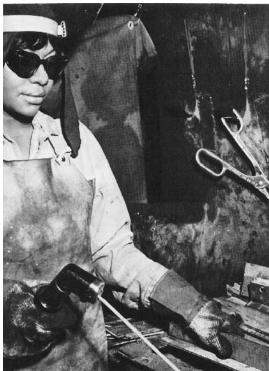
Fig. 13-54 A woman welding truss braces in industry. This job is similar to the practice jobs on T-joints.
