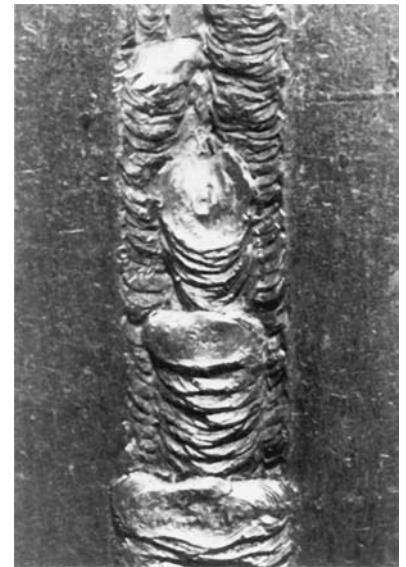
Fig. 15-63 Joint for the fillet weld soundness test welded in the vertical position, travel up (3F). Note the sequence of weld beads and the appearance.
