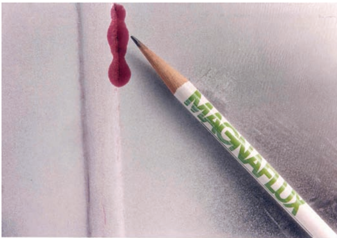
Fig. 28-41B Spotcheck® of a welded joint. © Magnaflux
