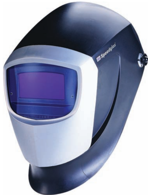
Fig. 32-8 This Speedglas® helmet equipped with an auto-darkening lens is lightweight and very flexible and so is appropriate for the welder to use when getting into hard to reach areas. It also has side windows to provide a peripheral view since the helmet can be used in the down mode for most work like grinding, cleaning, and inspection of welds. It has good neck protection and is designed to deflect the welding fumes around the helmet to keep the welder's breathing zone cleaner. © Hornell, Inc. Speedglas®
