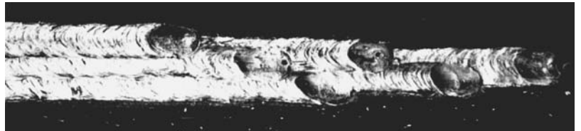
Fig. 13-90 Typical appearance of a multipass fillet weld done with the stringer bead technique in a T-joint welded in the horizontal position with DCEN or a.c. shielded arc electrodes.
