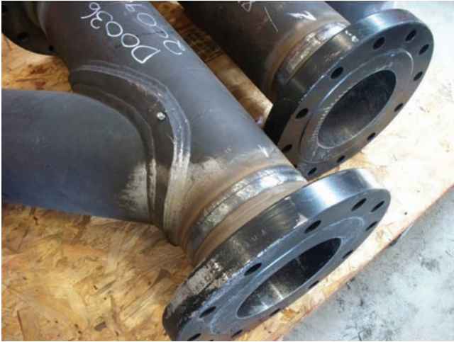
Fig. 16-77 A 45° lateral in 8 inch diameter pipe schedule 80 pipe with a weld ring for reinforcement plus the attached flange. © Piping Systems, Inc.
