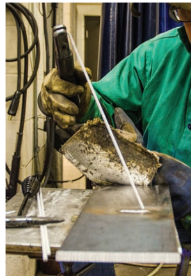
Fig. 13-8 Position of the electrode and electrode holder when striking the arc. Location: Northeast Wisconsin Technical College © McGraw-Hill Education/Mark A. Dierker, photographer
