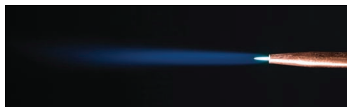
Fig. 8-4 Neutral welding flame does not have an excess of oxygen or acetylene. It is used for welding steel and cast iron. Its temperature is approximately 6,300°F. © David A. Tietz/Editorial Image, LLC
