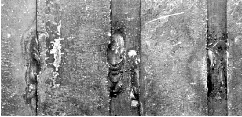
Fig. 14-14 Backing bar applied to the back side of a V-groove butt joint.
