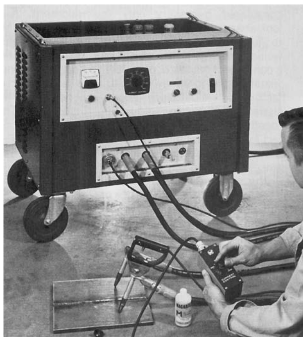
Fig. 28-30 Remote control used with a magnetic particle test unit. Welds can be inspected for incomplete penetration and fusion, slag inclusions, crater cracks, and porosity. © Magnaflux
