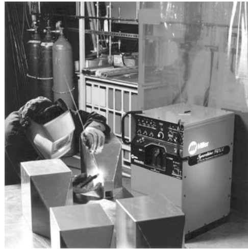
Fig. 18-35 This machine is recommended for pipe welding and other precision-type welding. It can be used for manual or automatic welding and for gas tungsten arc or shielded arc welding. It has a single output from 3 to 400 amperes. © Miller Electric Mfg. Co.
