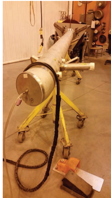
Fig. 18-40 Remote hand control unit with contactor control used with the machine shown in Fig. 18-30. © Miller Electric Mfg. Co.
