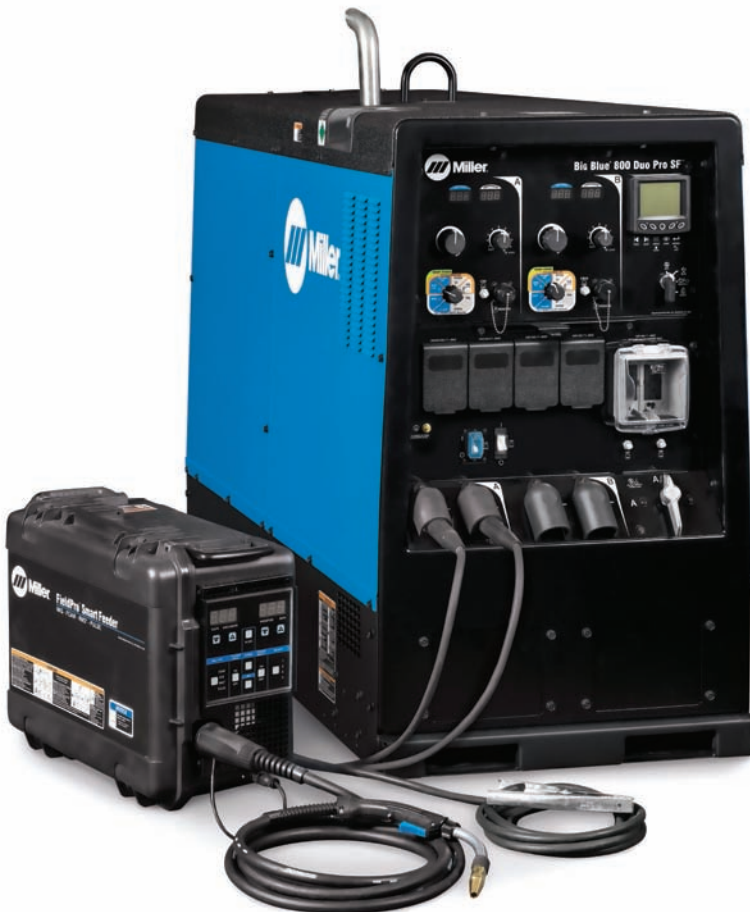
Fig. 23-7 Constant voltage/constant current family of d.c. welding machines. These are industrial rated machines at 100 percent duty cycle. Output ratings from 300 through 1,000 amperes are available to meet demanding needs. All the major processes like FCAW, SAW, GMAW, SMAW, and GTAW are capable with this type of equipment. These machines are capable of running ArcReach™ which allows control of the power source with the displayed remote control connected at the wire-feeder. © Miller Electric Mfg. Co.
