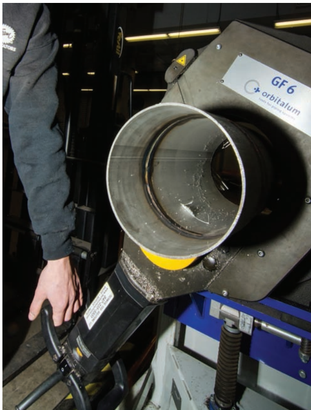
Fig. 16-90 A power saw for cutting various diameters and wall thicknesses of pipe. This is 8 inch schedule 5 stainless-steel pipe. Location: UA Local 400 © McGraw-Hill Education/Mark A. Dierker, photographer
