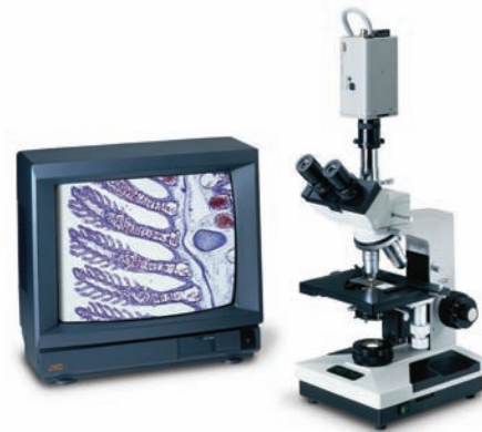
Fig. 28-92 This system consists of color cameras, monitors, power supply, and interconnection cables. Systems such as this greatly aid accuracy and efficiency by presenting larger images that reduce eye fatigue. The images can be captured and stored on film, video tape, and digitally. © Prior Scientific
