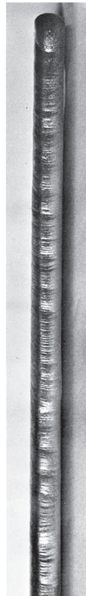
Fig. 8-27 An edge joint welded in the vertical-up position. It is made in \frac{1}{8} -inch steel plate. A no. 3 tip and a \frac{3}{32} -inch filler rod were used. The flame was neutral.
