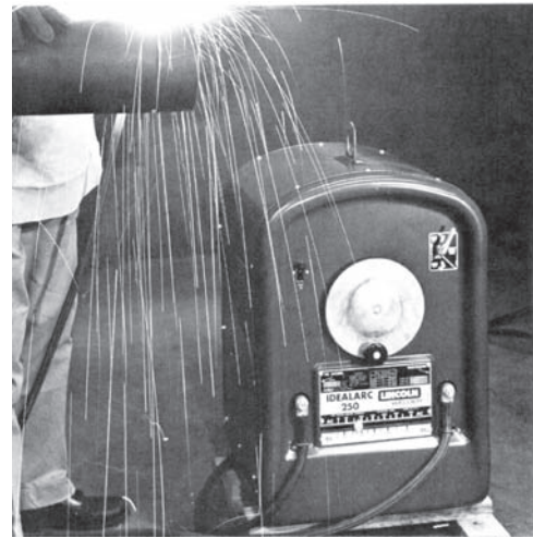
Fig. 11-15 A Lincoln a.c.-d.c. transformer-rectifier welding machine. In this model, which has a 300-ampere capacity, a hand-wheel permits continuous control of current. The a.c.-d.c. current selector is at the top right. A direct-reading current indicator is at the bottom of the machine. © Lincoln Electric
