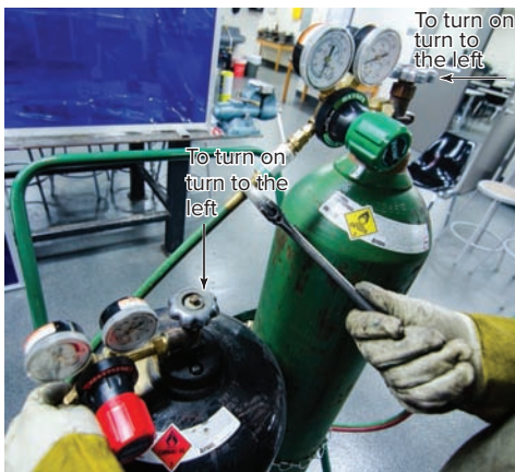
Fig. 7-23 Attaching the oxygen hose to the oxygen regulator. Location: Northeast Wisconsin Technical College © McGraw-Hill Education/Mark A. Dierker, photographer
