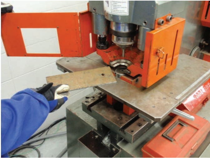
Fig. 26-78 Iron Worker used to punch a hole in a steel plate. Note the punch and die. The safety door is open to show interior components. © Renee Bohnart
