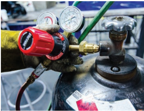
Fig. 7-22 Attaching a fuel regulator to a fuel cylinder. Note the gauge on the left is for the low pressure fuel gas for the torch. In this case acetylene is being used and red lines at 50 p.s.i. The gauge on the right is for the high pressure in the fuel gas cylinder. Location: Northeast Wisconsin Technical College © McGraw-Hill Education/Mark A. Dierker, photographer
