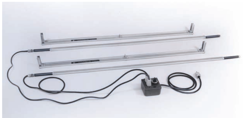
Fig. 31-5 Heat bars for bending and forming plastic. Handles materials up to ½ inch thick. Combination of variable temperature plus two heating surfaces results in adaptability to a wide range of materials, sizes, and thicknesses. © Laramy Products Co., Inc.
