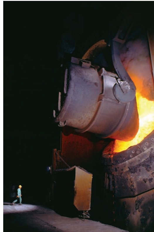
Fig. 3-16 Charging hot metal into a 150-ton basic oxygen furnace. © H. Mark Weidman Photography/Alamy Stock Photo
