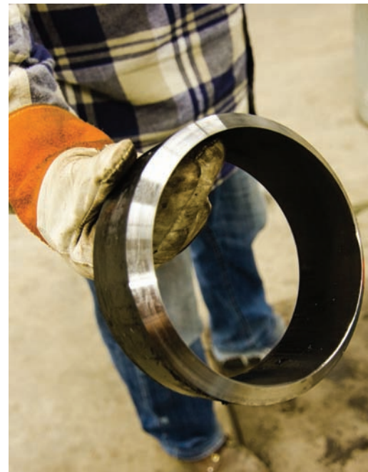
Fig. 4-6 For code quality work on CJP groove welds the appropriate end preparation must be provided. As indicated on this machine cut pipe nipple practice pipe. A typical bevel angle of 37\frac{1}{2}^\circ is used to produce a 75^\circ groove angle for butt joints. The root face will need to be applied. Location: UA Local 400 © McGraw-Hill Education/Mark A. Dierker, photographer
