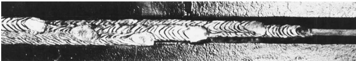
Fig. 14-22 Joint construction and typical appearance of a multipass single V-groove weld in a butt joint welded in the horizontal (2G) position with DCEP or a.c. shielded metal arc coated electrodes.
