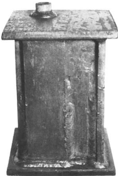
Fig. 15-65 One side of the pressure vessel test unit: a corner joint, lap joint, and T-joints are visible. Welds include both fillet and groove welds.
