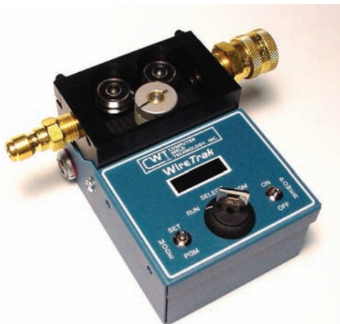
Fig. 27-12 This wire-feed speed sensor uses optical encoder technology to transmit information to the weld monitor. This, coupled with the amperage sensor, can be used to detect electrode extension. These data can be supplied to the motion control device and electrode extension can be accurately maintained. Weld volume, profile, deposition rates, as well as other issues may require accurate control and monitoring of wire-feed speed. © Computer Weld Tech., Inc.
