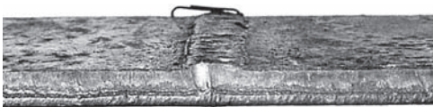
Fig. 3-44 Single V-groove butt joint that shows no distortion but may be high in stresses.
