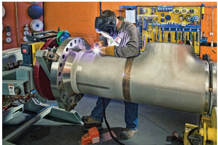
Fig. 26-9 A welding positioner teamed with a manual TIG weld being made on a flange to large bore heavy wall stainless steel pipe. The all welded positioner and the three jaw gripper is designed specifically for pipe welding shops. Note the two wireless foot pedals to control weld output and rotational speed. Also the well-organized tool rack. © Team Industries, Inc.
