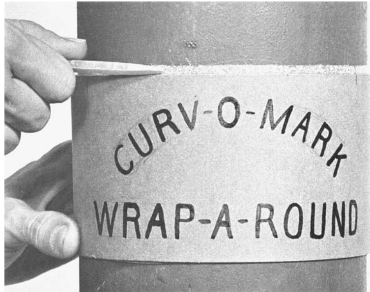
Fig. 16-99 Wrap-A-Round® for marking off square pipe ends.
