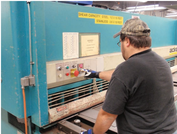
Fig. 26-47 A welding student is using a squaring shear with digital control over width of cut. Steel plate up to 10 feet wide and \frac{1}{2} inch thick can be sheared on this machine. © Renee Bohnart
