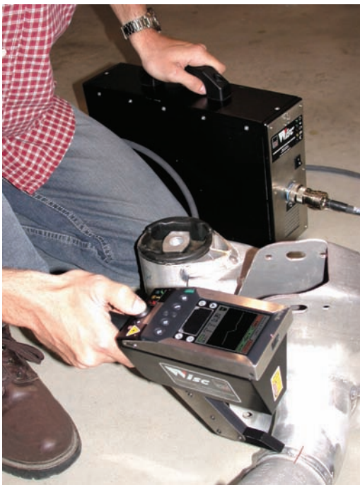
Fig. 28-116 Handheld laser scanner welding inspection system. Requires control and the gun that is shown. © Servo-Robot Corp.
