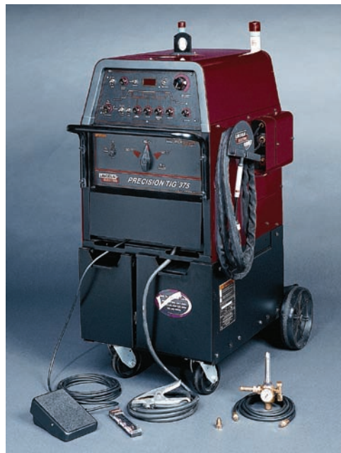
Fig. 18-37 A 375-ampere a.c.-d.c., constant current transformer with solid-state controls and square wave output. This machine can be used for a.c.-d.c. TIG and a.c.-d.c. stick electrode welding. Note the accessories and the cart with built-in water cooler. © Lincoln Electric
