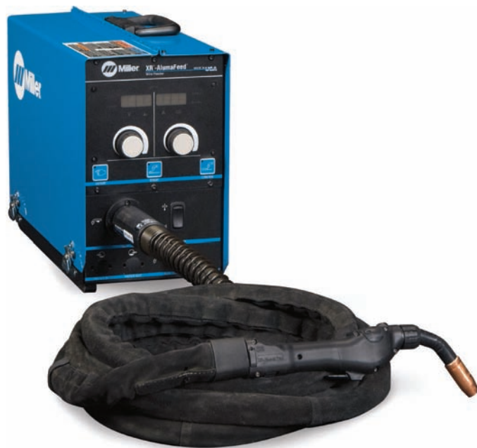
Fig. 21-40 This push-pull wire-feed system is designed specifically for aluminum MIG welding. There is a pull drive motor in the gooseneck gun, while the control and wire spool housing has a push motor. Guns are available from the spool supply housing of 15, 25, and 35 feet for maximum reach. The maximum allowable spool diameter is 12 inches. This water-cooled version is rated at 400 amperes at 100 percent duty cycle. It has an electrode wire diameter capacity of 0.030 to 0.047 inch with a wire-feed speed range of 70 to 875 inches per minute. Note the gun trigger and wire-feed speed control located in the base of the gun handle. © Miller Electric Mfg. Co.
