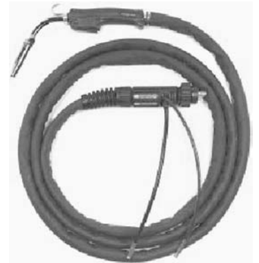
Fig. 21-49 A water-cooled gun rated at 450 amperes with carbon dioxide shielding and 400 amperes with argon or argon mixed gases at 100 percent duty cycle. © Lincoln Electric
