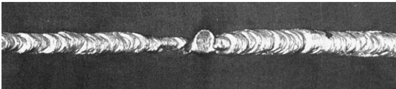
Fig. 15-4 Penetration and fusion through the back side of a V-groove butt joint. Note the spot in the center of the bead where there is a break in the penetration. This can be caused by failure to burn through a tack or a poor tie-in on a restart.
