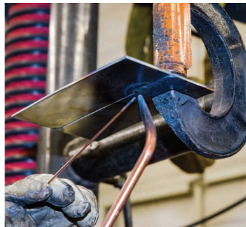
Fig. 8-39 Welding a butt joint in the overhead position, using the backhand welding technique. Location: Northeast Wisconsin Technical College © McGraw-Hill Education/Mark A. Dierker, photographer
