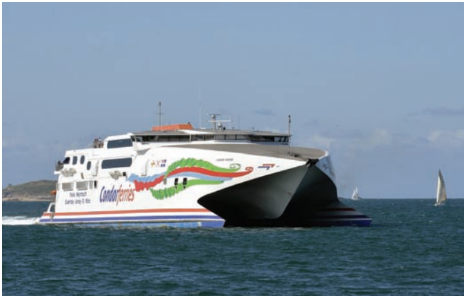
Fig. 2-27 This Tri-Hull 319-foot long high speed ferry can carry 760 passengers and 200 vehicles at speeds of 40 knots or 46 mph. With 38,000 HP from four diesel engines. Made from lightweight aluminum, the boat was fabricated using the pulsed gas metal arc welding process. © Miguel Medina/AFP/Getty Images
