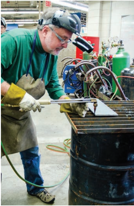
Fig. 7-33 Position while cutting over an appropriate area. Location: Northeast Wisconsin Technical College © McGraw-Hill Education/Mark A. Dierker, photographer
