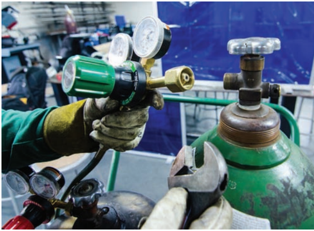
Fig. 7-21 Attaching an oxygen regulator to an oxygen cylinder. One gauge is for the high pressure in the oxygen cylinder while the other is for the working pressure in the torch. Location: Northeast Wisconsin Technical College © McGraw-Hill Education/Mark A. Dierker, photographer
