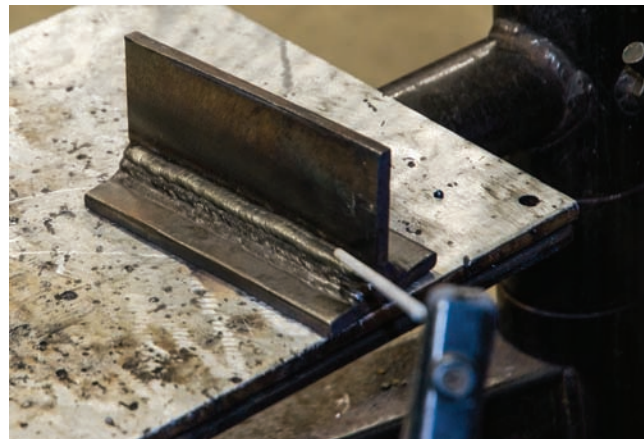
Fig. 13-84 Welding a T-joint in the horizontal position. The electrode and electrode holder are positioned as instructed in Fig. 13-83. Location: Northeast Wisconsin Technical College © McGraw-Hill Education/Mark A. Dierker, photographer
