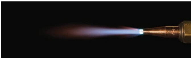
Fig. 7-30 Oxidizing cutting flame. It is an excess oxygen flame used only for rough work. It reduces preheat time. © David A. Tietz/Editorial Image, LLC
