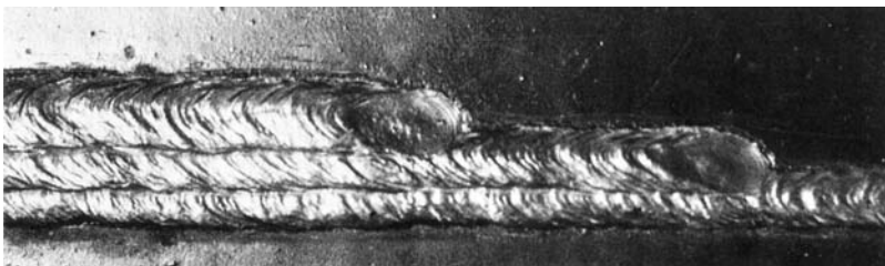
Fig. 13-43 Typical appearance of stringer beads welded in the horizontal position with DCEP or a.c. shielded arc electrodes.
