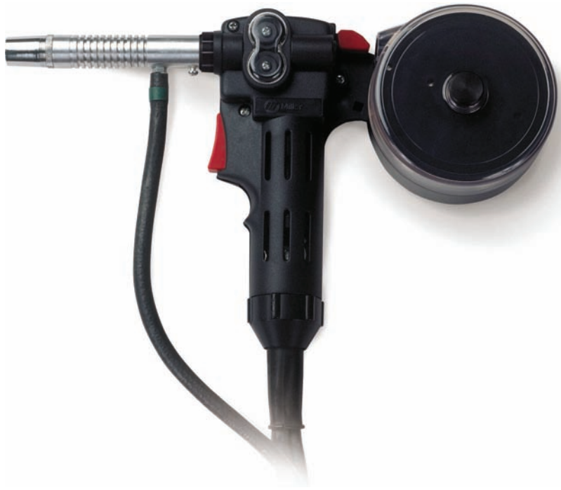
Fig. 21-43 This spool gun provides reach and accessibility. The gun contains the wire and the drive motor system. Since the wire is pushed only a few inches, smooth feeding of difficult-to-feed wire like aluminum is easily accomplished. Ideal for light industrial applications, the gun is rated for 150 amperes at 60 percent duty cycle and has a 20-foot weld control/cable. The electrode wire diameter capacity is 0.023 to 0.035 inches for aluminum, steel, and stainless steel, with wire-feed speeds of from 115 to 715 inches per minute. The maximum spool size capacity is 4 inches. © Miller Electric Mfg. Co.
