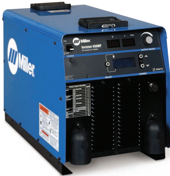
Fig. 21-31 A 450-ampere d.c. inverter power source. This machine has the capability to output c.v.-c.c., so it is multiprocess capable. It is designed specifically for the GMAW-P process for all position welding on thick and thin materials without spatter. It has a built-in microprocessor that allows both manual as well as synergic (adaptive or non-adaptive) control of the pulse output. It is also capable of running all modes of metal transfer as well as FCAW, GTAW, and SMAW processes. SAW and CAC-A up to its output capability are also recommended. © Miller Electric Mfg. Co.
