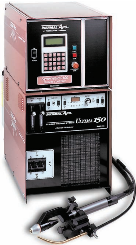
Fig. 18-62 A plasma welding unit. Note control on top of power source and automatic torch with wire delivery system. © Thermadyne Industries, Inc.
