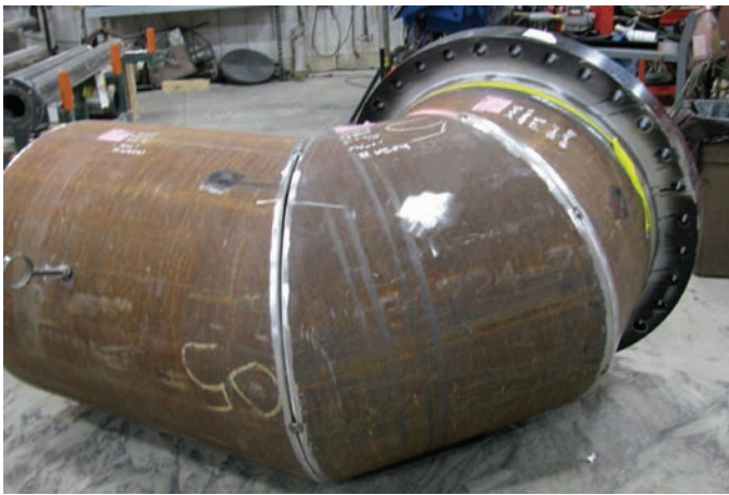
Fig. 16-27 A steel 90° three-segment elbow with flange, tacked and ready to be loaded into a welding positioner for final welding. © Piping Systems, Inc.
