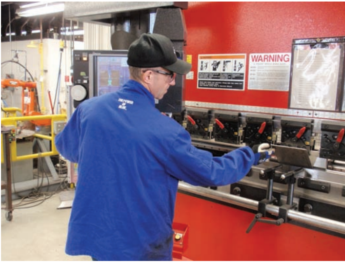
Fig. 26-39 An instructor demonstrating the use of a power press brake prior to welding. Note the proper hand position, as the part is bending in the upward direction. © Renee Bohnart
