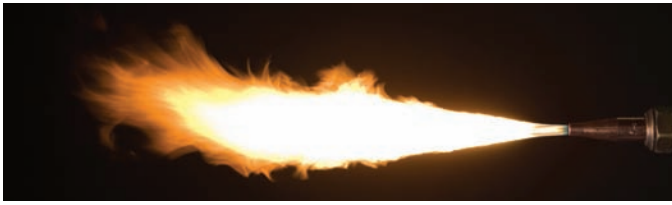
Fig. 7-27 Atmospheric burning of acetylene. Open acetylene valve until smoking of the flame disappears. © David A. Tietz/Editorial Image, LLC
