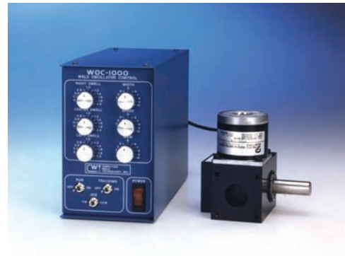
Fig. 27-4 A pendulum-type weld oscillator and control system. The \frac{5}{8} -inch diameter shaft is for attachment of gun or torch mounting assembly. This WOC-1000™ system features Thru-Arc™ tracking technology that allows automatic torch centering and width control. © Computer Weld Tech., Inc.
