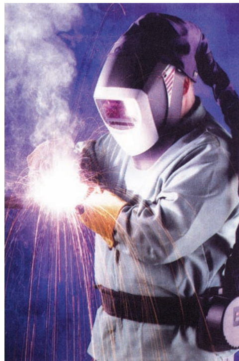
Fig. 32-6 A helmet equipped with an auto-darkening lens and a forced air respirator. Note the welder's good head position in relation to the fume plume and the other personal protection equipment (PPE), such as gloves and welder's jacket being effectively used. The helmet can remain in the down position for weld cleaning, inspection, and grinding. This protects the face and keeps the respirator in a proper position. © American Welding Society, Welding Science and Technology, Vol 1 of Welding Handbook, 9th ed., Fig 17.5, p.723
