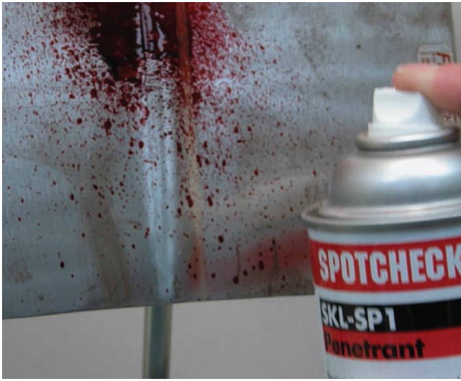
Fig. 28-41A Applying Spotcheck®. © Magnaflux
