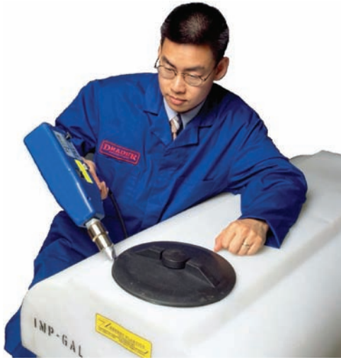
Fig. 31-8 Welder using an injection welding machine to attach an access cover on a plastic tank. © Drader Manufacturing
