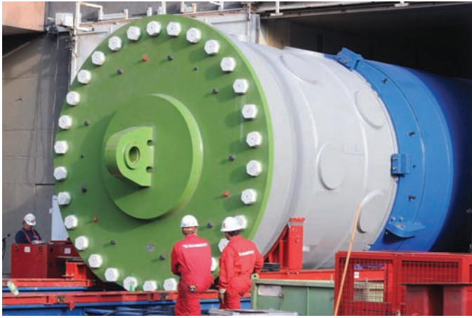
Fig. 2-16 This large reactor for a nuclear power plant is designed to withstand high pressure and high temperatures. Wall thicknesses are typically over several inches thick and welding plays a critical role in their manufacture. Note the large lifting eyes. Large crawler cranes can lift this type mega ton load into position in one lift. © Frank Hormann/AP Images
