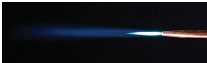
Fig. 8-6 Carburizing welding flame commonly used for welding white metal, stainless steel, hard facing, some forms of pipe welding, and soldering and brazing. © David A. Tietz/Editorial Image, LLC
