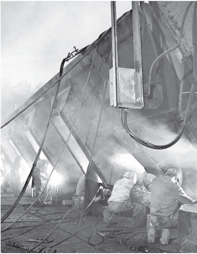
Fig. 2-24 A crew of 23 arc welders supply their own light for the photographer as they apply 100 feet of weld in a matter of minutes to the underframe of a Center Flow dry bulk commodities railroad car, with a capacity of 5,250 cubic feet. © ACF Industries
