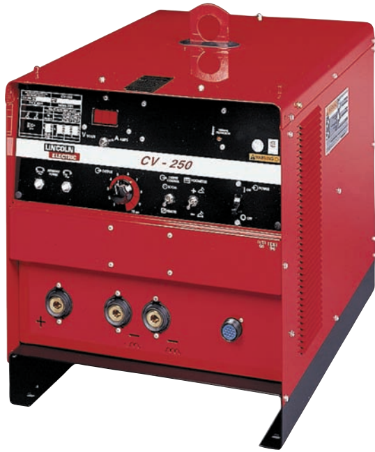
Fig. 21-30 This 250-ampere, constant voltage solid-state controlled transformer-rectifier has an output rating of 7 to 32 volts and 30 to 300 amperes available in one continuous range. Note the quick twist connections for high and low inductance and the polarity output hook-up. GMAW and FCAW up to its output capability are the appropriate applications. © Lincoln Electric
