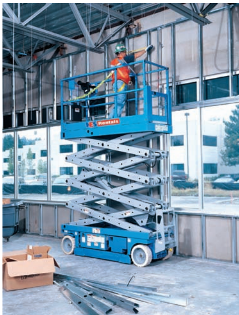
Fig. 26-18 A motorized scissor lift. A joystick is used to control lift and steering. © NES Rentals
