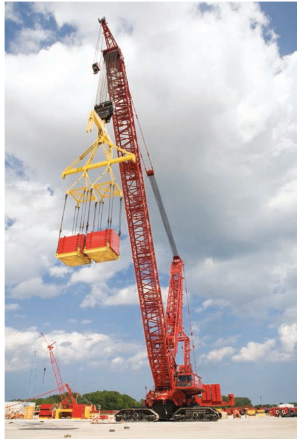
Fig. 2-11 This type of large-capacity crawler crane can lift up to 5.5 million pounds in a single lift. This design employs an innovative lift-enhancing mechanism, which eliminates the need for a counterweight wagon. This feature, called the VPC (variable position counterweight), never touches the ground and extends or retracts as needed by the crane's lift. © The Manitowoc Company, Inc.
