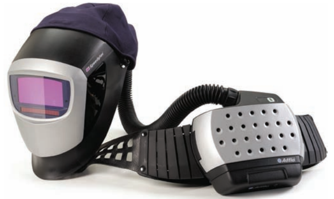
Fig. 32-15 Particle fume protection for welders. 1. Auto-darkening lens. Different models are available. 2. Narrow helmet design with extended throat protection, heat reflective silver front, and made from lightweight materials. 3. Speedglas® side window for peripheral vision which increases the welder’s field of view by 100 percent. 4. Battery, turbo fan, and filter all in one compact belt pack unit. © Hornell, Inc. Speedglas®
