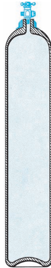
Fig. 5-5 Sectional view of an oxygen cylinder. Oxygen cylinders are seamless, drawn-steel vessels having a malleable iron neck ring shrunk on at the top and a cylinder valve screwed into the neck.
