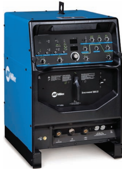
Fig. 11-14 A 300 amp a.c.-d.c. GTAW/SMAW machine. This machine has square wave output which is advantageous for TIG and stick welding. © Miller Electric Mfg. Co.
