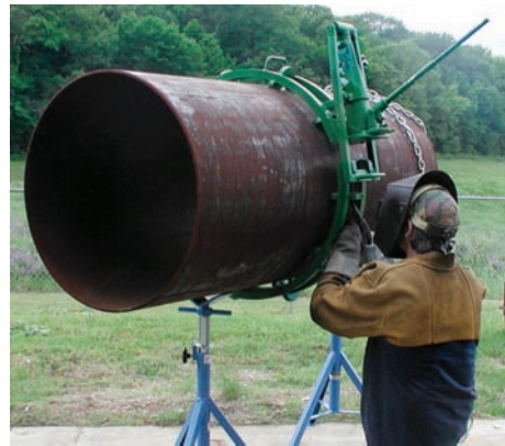
Fig. 16-25 This hydraulic cage clamp produces the extra strength necessary for aligning large pipe diameters. Pipes can be effortlessly aligned due to the design of the Hydraulic Closure Mechanism. Clamps are available for 16- to 60-inch pipes. © Mathey Dearman
