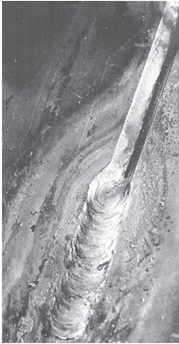
Fig. 8-44 A butt joint, V-groove weld in pipe. Note the complete fusion and penetration at the leading point of the weld. Note also the size in relation to the width of the joint. © Praxair, Inc.
