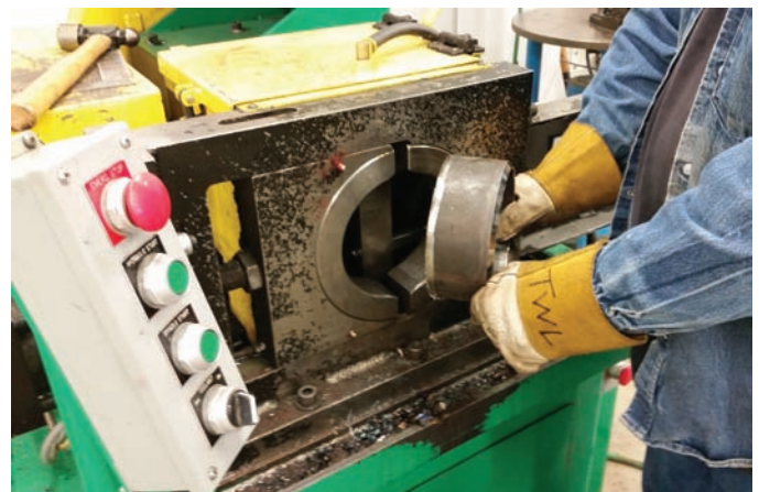
Fig. 16-84 A pipe-beveling machine preparing pipe with a heavy wall thickness. © Edward R. Bohnart
