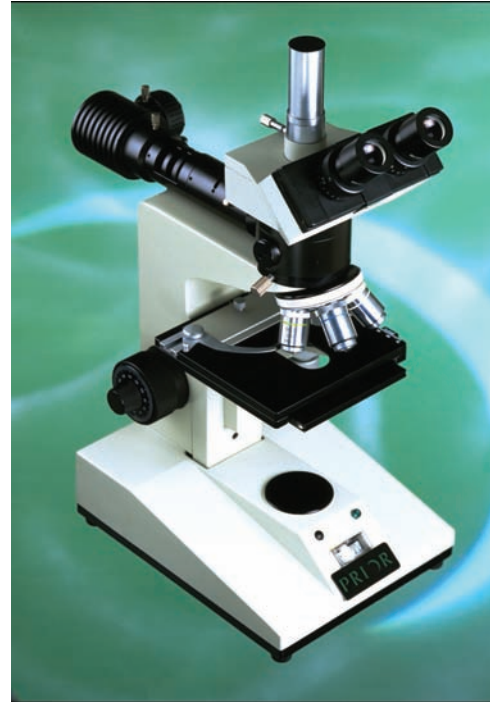
Fig. 28-91 Metallurgical microscope featuring 50× to 1500× magnification range and 20-watt variable halogen illumination for examination of polished weld specimens. © Prior Scientific
