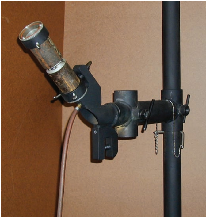
Fig. 20-1 An A106B pipe of 2-¾ inch O.D. and a wall thickness of 5/8 inch in the 6G position. For a welder qualification test coupon, this can save 80% of the weld time and material vs. a 6 inch O.D. double extra heavy pipe coupons. This coupon will qualify for unlimited thickness and diameters as small as 1 inch O.D. using two weld processes. Such as GTAW on the root and filling half the joint and SMAW for the remainder of the joint. When welded in accordance to the current ASME Section IX requirements. The purge set up may or may not be required, always follow the welding procedure. © Renee Bohnart
