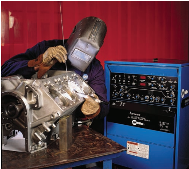
Fig. 3-41 Use of aluminum for the transportation industry for an engine block; previously made of cast iron. This block is undergoing some GTAW repair. © Miller Electric Mfg. Co.
