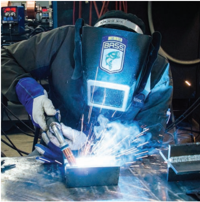
Fig. 22-1 This student is practicing gas metal arc welding. Note the dual-digital wire-feeder in the back ground, the wire cutter and practice coupon. Location: Northeast Wisconsin Technical College © McGraw-Hill Education/Mark A. Dierker, photographer
