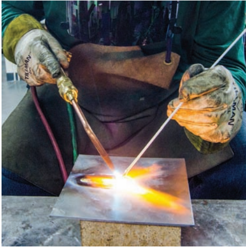
Fig. 9-3 The brazing action. After a spot at the edge of the plate has been heated to a visible red, some bronze from the fluxed rod is melted on the hot area. The bronze filler metal spreads and runs evenly over the hot surface. This practice is known as tinning . Location: Northeast Wisconsin Technical College © McGraw-Hill Education/Mark A. Dierker, photographer
