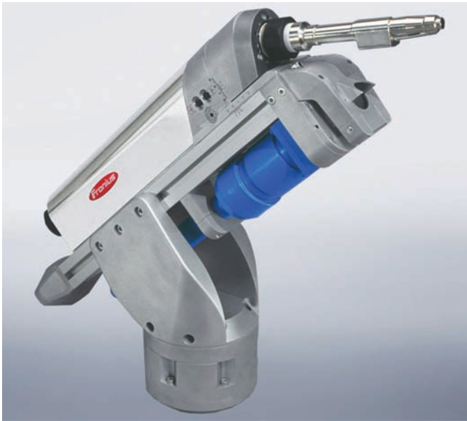
Fig. 25-13 Laser/MIG welding head designed for mounting on a robot arm. Weight is approximately 42 pounds, and size is approximately 30 × 6 × 16 inches. The MIG portion is rated at 100 percent duty cycle at 250 amps and the laser is rated at 4 kilowatts. © Fronius International GmbH
