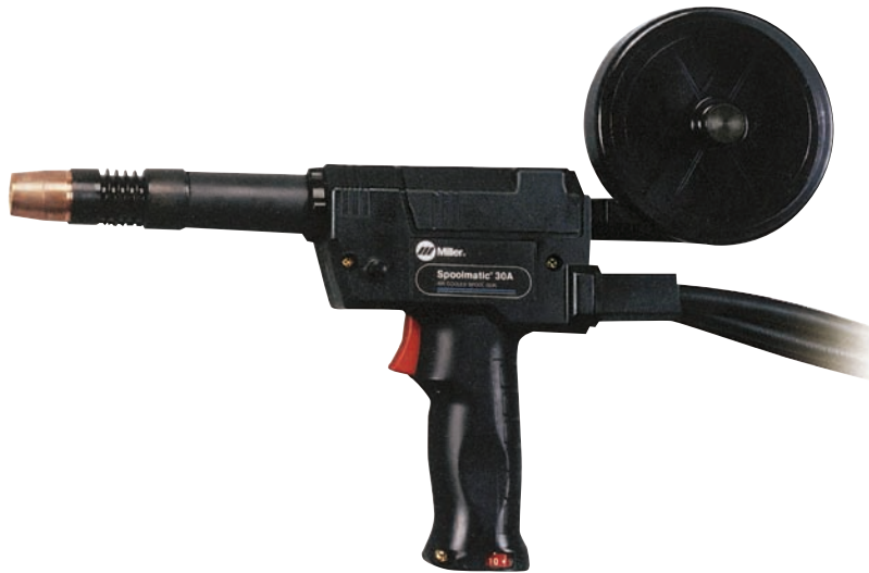
Fig. 21-44 For more industrial type applications this spool gun is rated for 200 amperes and 100 percent duty cycle. The electrode wire diameter capacity is 0.023 to \frac{1}{16} inch for aluminum wire and stainless steel and steel wire up to 0.045 inch, with wire-feed speeds of from 70 to 875 inches per minute. The maximum spool size is 4 inches. © Miller Electric Mfg. Co.
