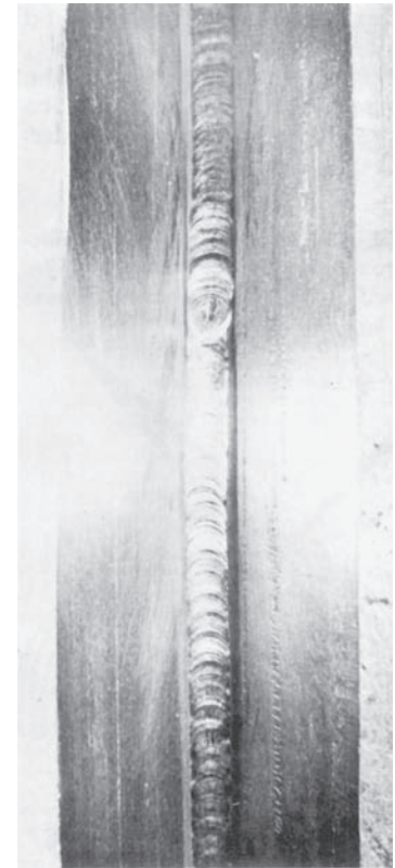
Fig. 20-21 Face contour of a satisfactory root pass in stainless-steel pipe. © Crane Co.
