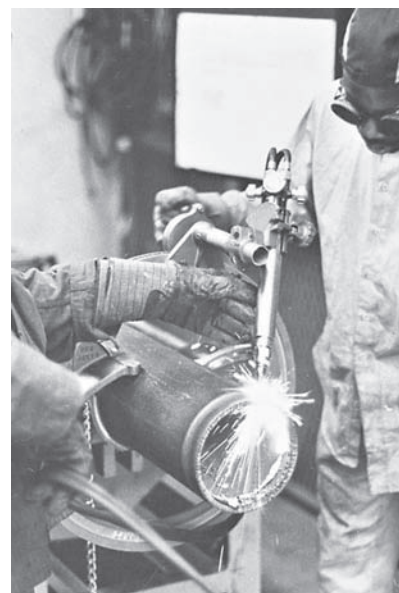
Fig. 8-41 Students beveling the edge of a pipe with a standard beveling machine.
