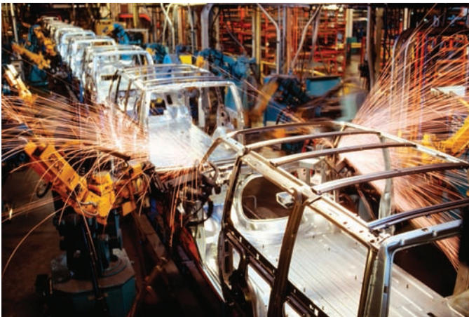
Fig. 2-8 Robotic welders assemble a vehicle chassis. © Glow Images
