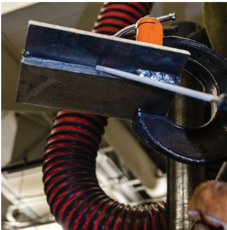
Fig. 15-14 Electrode and electrode holder positioned as instructed in Fig. 15-13. Note how the joints are held by the jig. © McGraw-Hill Education/Mark A. Dierker, photographer
