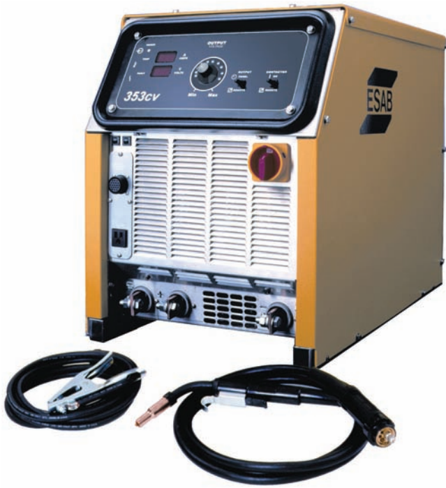
Fig. 21-21 A 350-ampere, d.c. constant voltage transformer rectifier with solid-state control for short circuit transfer MAG/MIG welding. The single knob control changes voltage in infinite units for precise control over the arc. It is capable of running continuous spray and flux cored arcs up to its amperage capability. © ESAB
