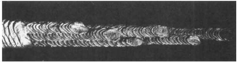
Fig. 13-97 Typical appearance of a multipass fillet weld done with the stringer bead technique and a weaving overlay in a T-joint welded in the horizontal position with DCEP or a.c. shielded arc electrodes.
