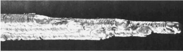
Fig. 14-37 Typical appearance of a multipass fillet weld in a T-joint welded in the horizontal position with E7016 low hydrogen electrodes for the stringer passes and DCEP or a.c. shielded metal arc coated electrodes.
