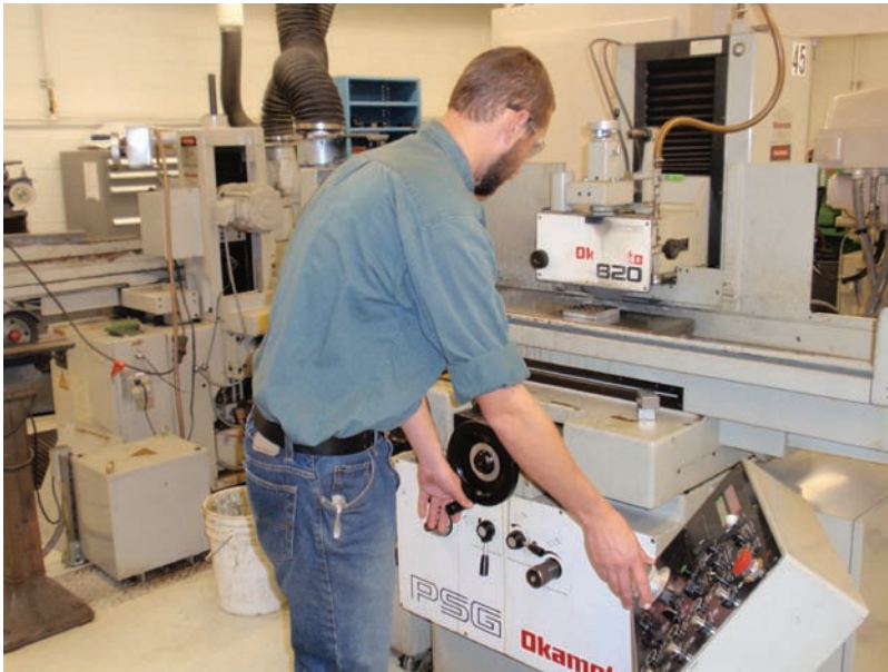
Fig. 26-75 Surface grinders can be used for various weld preparation such as tensile test specimens. © Renee Bohnart
