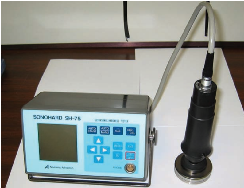
Fig. 28-58 Compact portable sonic hardness tester designed for massive workpieces. It can measure in all directions and in poorly accessible places. The RS 232 C port allows for download from memory storage. © Micro Photonics Inc.
