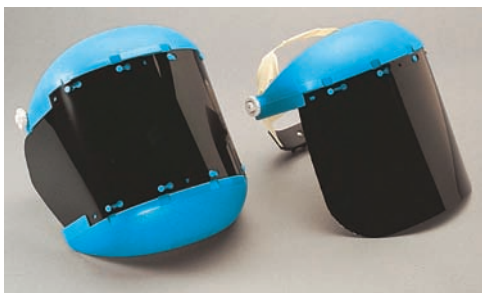
Fig. 32-3 Faceshield provides protection from sparks, spatter, grinding, and hot slag. These units are equipped with a shade 5 lens for protection against infrared and ultraviolet rays. Clear acetate lenses are also available. © Sellstrom Manufacturing Company
