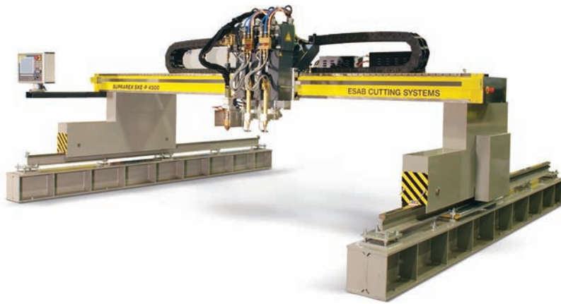
Fig. 17-23 A large gantry system with multiple-head capacity. Travel speed from 2–1,400 inches per minute. Note the vision computer numerical control. © ESAB
