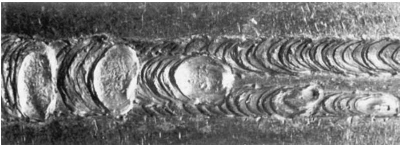
Fig. 15-62 Joint for the fillet weld soundness test welded in the horizontal position (2F). Note the sequence of weld beads and the appearance.
