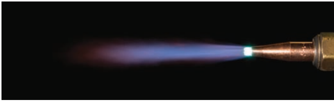
Fig. 7-29 Neutral cutting flame without excess oxygen or acetylene. At proper adjustment, the temperature of the flame is approximately 6,300°F. © David A. Tietz/Editorial Image, LLC
