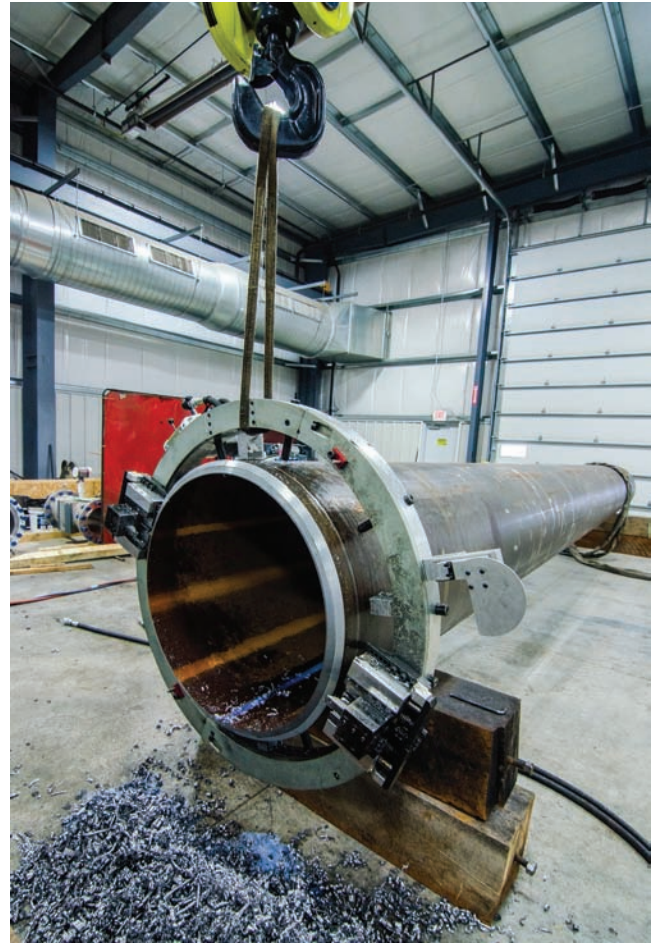
Fig. 16-93 A machine cutting tool being used to bevel pipe for both in the shop and in the field. It is capable of machining square, bevel and J's for various types of groove welds. Location: Piping System's Inc. © McGraw-Hill Education/Mark A. Dierker, photographer
