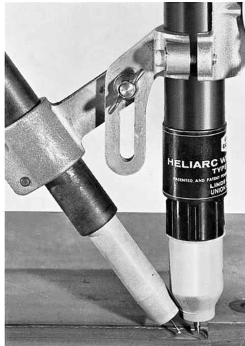
Fig. 18-55 The TIG hot wire welding system employs a special wire feed torch mounted behind the TIG welding torch to supply molten filler metal to the weld pool. © Praxair, Inc.
