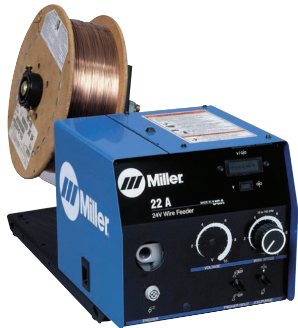
Fig. 21-34 A typical bench style wire feeder that is designed for constant wire-feed speed. This allows it to operate all the GMAW modes of transfer as well as FCAW applications. Input power required from the power source to operate the feeder is 24 V a.c., 7 amperes, 50/60 hertz. The feeder is designed to handle electrode wire diameters of 0.023 to \frac{5}{64} inch at wire-feed speeds from 75 to 750 inches per minute with a maximum spool capacity of 60 pounds. Note the simple controls for wire-feed speed, trigger hold, wire jog, and shielding gas purge. © Miller Electric Mfg. Co.
