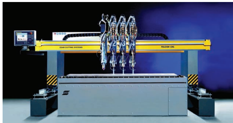
Fig. 17-21 Gantry-type mechanized cutting machine with PAC speeds up to 400 inches per minute. © ESAB
