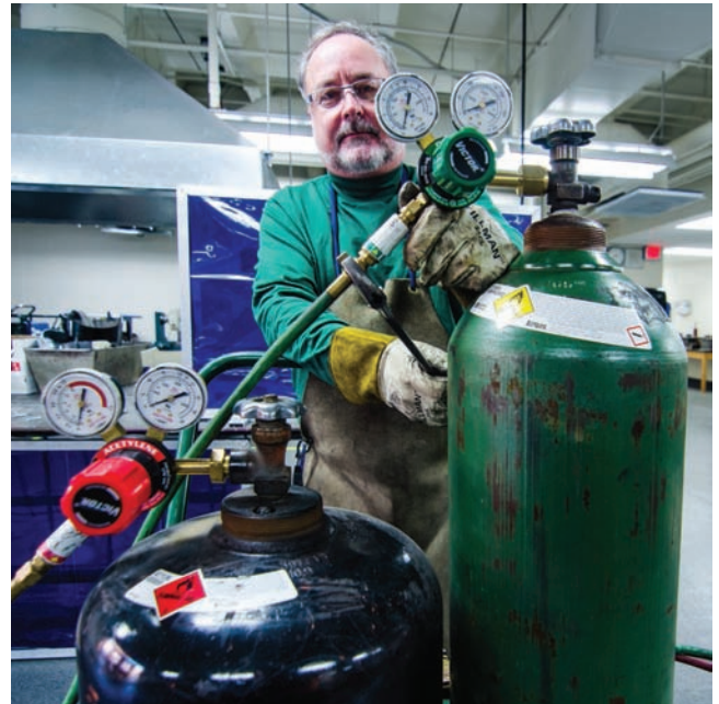
Fig. 11-40 An apron helps protect the welder from sparks and heat. Northeast Wisconsin Technical College © McGraw-Hill Education/Mark A. Dierker, photographer
