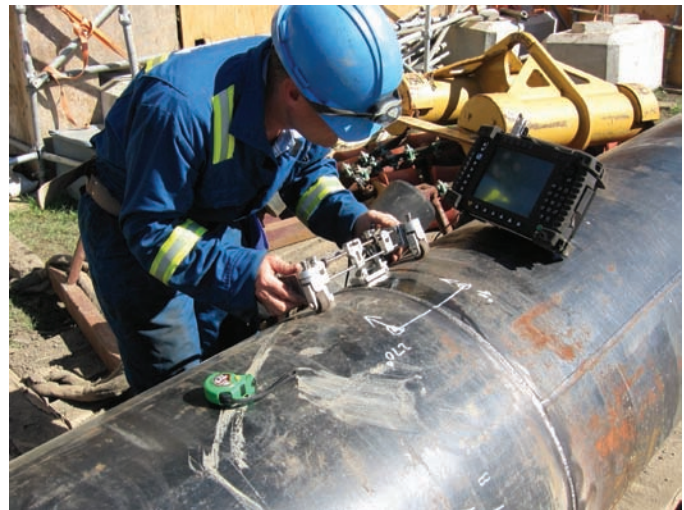
Fig. 28-46 This code-compliant conventional ultrasonic flaw detector can also perform weld or phased array inspections utilizing simple menu-driven interfaces. Training can be minimal and these systems can solve very demanding inspection applications in less time at affordable pricing. This UT technician is performing critical inspection on a piping system in a petrochemical plant. © David Mack
