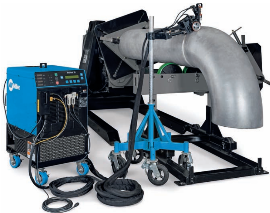
Fig. 26-31 A 35-kW high frequency induction heating system setup on a sample pipe and 90° elbow. The rolling induction system allows consistent heating which allows the welder to set target preheat temperature and maintain it as the positioner rolls the pipe and the weld is being performed. © Miller Electric Mfg. Co.
