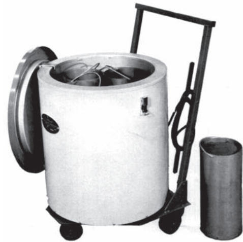
Fig. 12-12 This portable flux holding oven may also be used for flux cored wire. © Phoenix International
