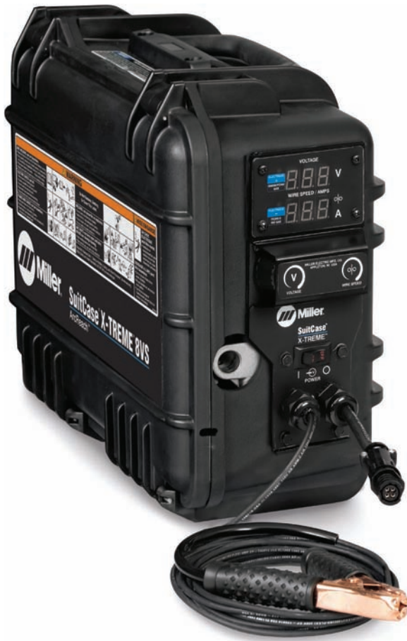
Fig. 21-37 This highly portable control-feeder weighs less than 25 pounds and fits through a 18x24 inch porthole. The small modular design and tough flame-retardant, nonmetallic case materials will withstand burning, breaking, or loss of rigidity with heat or sun. This is a voltage sensing feeder and so operates on the open circuit arc voltage of the power source and must be supplied 15 to 100 V d.c. The clamp and cable shown must be connected to the work piece. Electrode wire diameter capacity is 0.023 to 0.052 inch. Wire-feed speed is from 50 to 700 inches per minute depending on the arc voltage supplied. The maximum spool size on this feeder is 8 inches and 14 pounds. Digital display of voltage, wire feed speed, and also amperage if desired. Meters can be seen clearly even in direct sunlight. © Miller Electric Mfg. Co.
