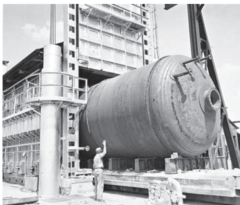
Fig. 3-33 All-welded pressure vessel being removed from a heat-treating furnace. © Nooter Corp.
