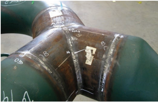
Fig. 16-82 A 10 inch diameter schedule 40 special Y, also know as “pant legs” with an elbow and two reducers welded to it. © Piping Systems, Inc.
