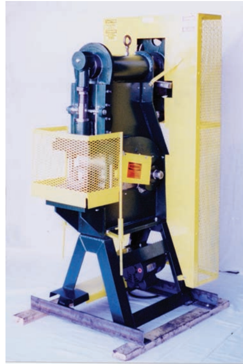
Fig. 26-79 An 18-ton power iron worker capable of shearing, punching, and forming. It is capable of approximately 48 strokes per minute. Note the safety guards. © Rogers Manufacturing Inc.
