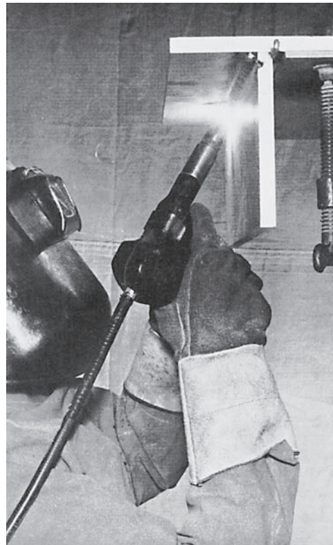
Fig. 22-39 Position of MIG gun when welding a T-joint in aluminum plate in the 4F position. © Kaiser Aluminum
