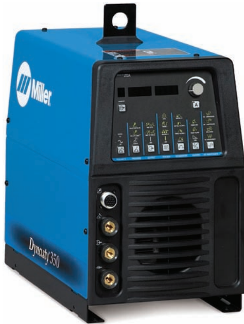
Fig. 18-16 This power source provides output from 5 to 300 amperes. It is an a.c.-d.c. inverter GTAW/SAW power source. It features frequency control and expanded balance control for enhanced square wave output. Its weight is only 90 pounds. © Miller Electric Mfg. Co.
