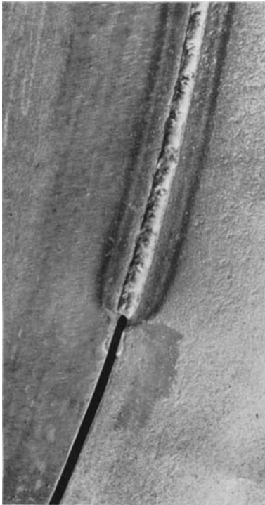
Fig. 24-43 Inside of vessel showing penetration of a root pass deposited in the pressure vessel shown in Fig. 24-44. The joint shows complete penetration free of all obstruction. Root reinforcement is between \frac{1}{32} and \frac{3}{32} inch.
