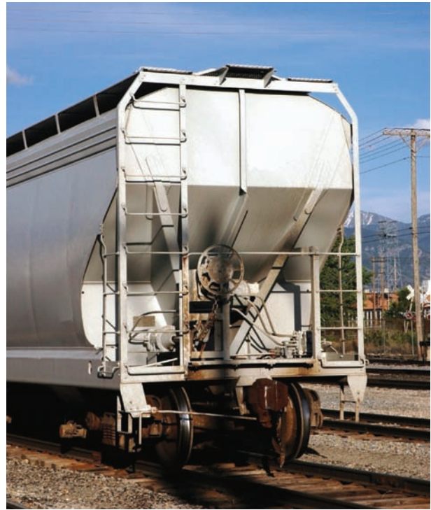
Fig. 2-25 The end view of a covered hopper railcar. Note its clean smooth appearance. Ease of cleaning and painting are other reasons for making welding a good choice in fabricating products like this. © stayorgo/iStockphoto/Getty Images
