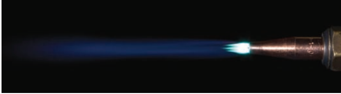
Fig. 7-28 Carburizing cutting flame. It is an excess acetylene flame. More oxygen is required for preheat flames. © David A. Tietz/Editorial Image, LLC
