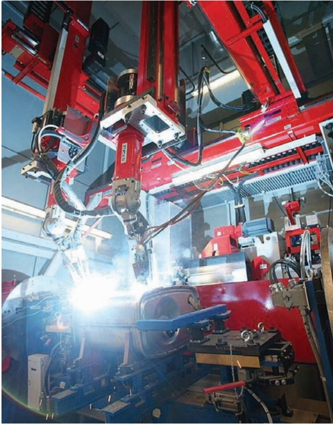
Fig. 27-21 Dual robot work cell. Note the robots are mounted overhead for easier access to welding joints. © Reis Group Holding GmbH & Co. KG
