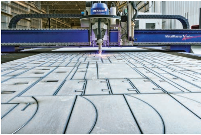
Fig. 17-4 Plasma arc cutting makes shape and line cuts on hard-to-work metals such as this 1¼-inch stainless-steel plate. © Team Industries, Inc.
