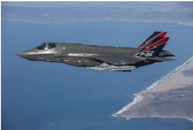
Fig. 2-2 A 5th generation F-35 Lightning II Joint Strike Stealth Fighter, capable of Mach speed with vertical takeoff and landing capability. Currently considered the world's most advanced fighter plane. U.S. Air Force
