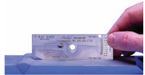
Fig. 28-111 To measure depth of undercut, set the gauge on base metal with the pointer in the bottom of the undercut. Directly read the depth on the scale as indicated. The locking screw can be tightened to hold the reading for future reference. © G.A.L. Gage Co.
