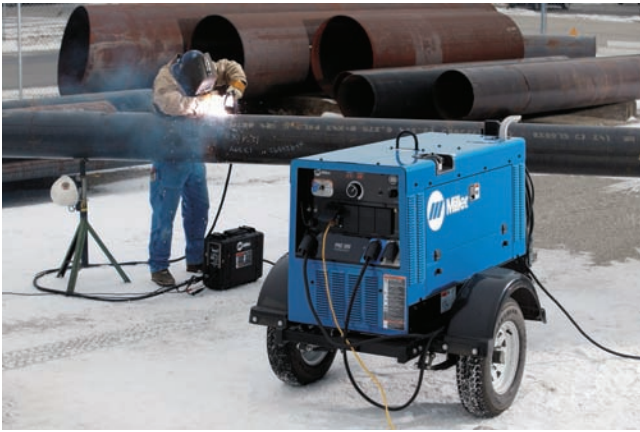
Fig. 21-33 Engine-drives of this type generator are available up to 800-amps. For industrial auxiliary strength and weld power in the field, it has c.v.-c.c. versatility. For stick welding, it also provides semiautomatic welding with large diameter, high deposition flux cored wires. The welder is using a suitcase type feed, with FCAW-S electrode wire, and trailer for mobility. © Miller Electric Mfg. Co.
