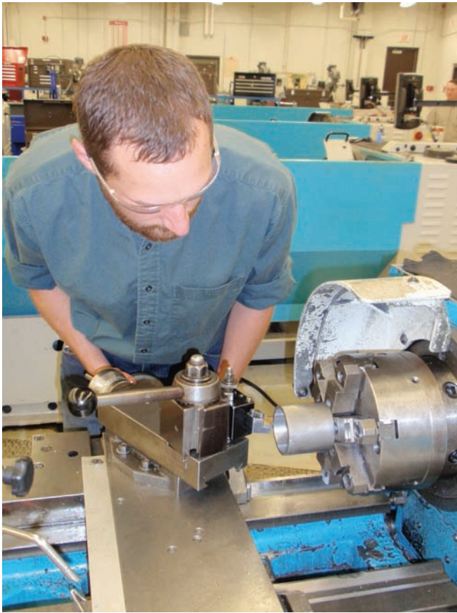
Fig. 26-69 Setting up to bevel a 3-inch diameter section of steel pipe on the lathe in preparation for welding. © Renee Bohnart
