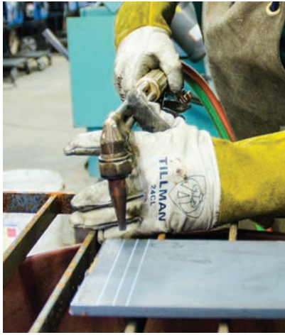
Fig. 7-39 Position of the cutting torch when making square cuts in the flat position. Location: Northeast Wisconsin Technical College © McGraw-Hill Education/Mark A. Dierker, photographer
