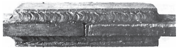
Fig. 28-87 Side view of a longitudinal fillet weld specimen.
