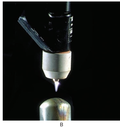
Fig. 18-56 (A) A PAW torch mounted on a robot arm. (B) A close-up view of the torch shows that the pilot arc is on. Note that the arc has not yet transferred to the weldment. © Thermadyne Industries, Inc.
