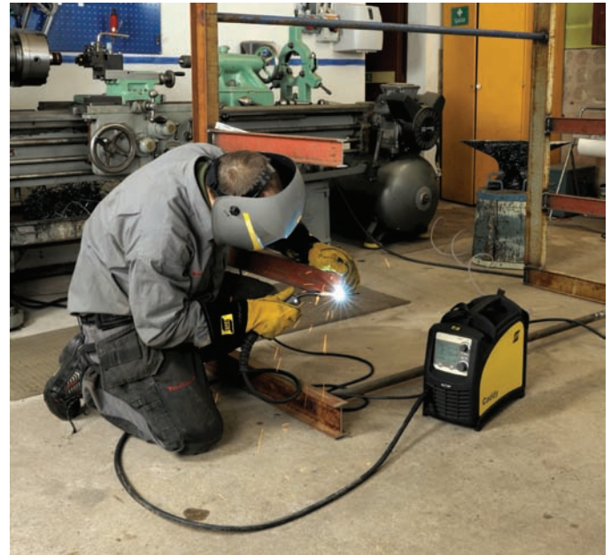
Fig. 32-2 A welder properly protected for the MIG/MAG process. He is wearing a helmet, a leather sleeve on his left arm, and leather gloves. He has rolled down the cuffs of his pants so that they cannot catch particles of hot metal. © ESAB
