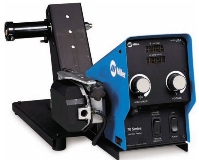
Fig. 21-36 This digital wire feeder allows much more rapid setup for a welding procedure and keeps the process in control by accurately controlling and displaying voltage and wire-feed speed. It operates from input power (24 V a.c., 10 amperes, 50/60 hertz) provided by the power source. It is capable of handling electrode wire diameters of 0.023 to 1/8 inch and wire-feed speeds of 50 to 780 inches per minute. Note the digital readout on voltage and wire-feed speed and the simple controls. © Miller Electric Mfg. Co.
