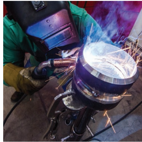
Fig. 24-25 This pipe stand allows the welder to maneuver around it to maintain proper eye contact with the leading edge of the weld pool. The pipe is positioned so that it is a good height for the body mechanics required. Along with contact tip to work distance, travel speed, travel angle, and work angle to assure complete joint penetration and weld profile. Location: UA Local 400 © McGraw-Hill Education/Mark A. Dierker, photographer
