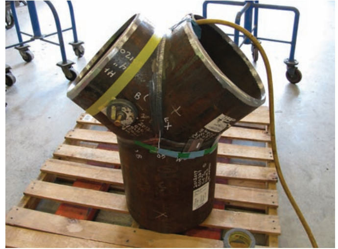
Fig. 2-17 A 'Y' branch shop fabricated undergoing NDE to assure weld quality through soundness testing. GMAW root pass followed by FCAW fill and final beads. © Piping Systems, Inc.
