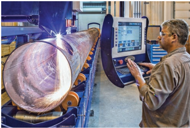
Fig. 17-5 Cutting various branch connections like T, K, and Y in pipe with the plasma process. Pipe diameter 3–48 inches can be accommodated. This machine can use plasma or oxyfuel for cutting. Equipment conveys pipe from outside storage rack to the cutting machine. The cutting head is a CNC controlled with a 5-axis and a touch sensitive screen for ease and accuracy of production requirements. © Team Industries, Inc.
