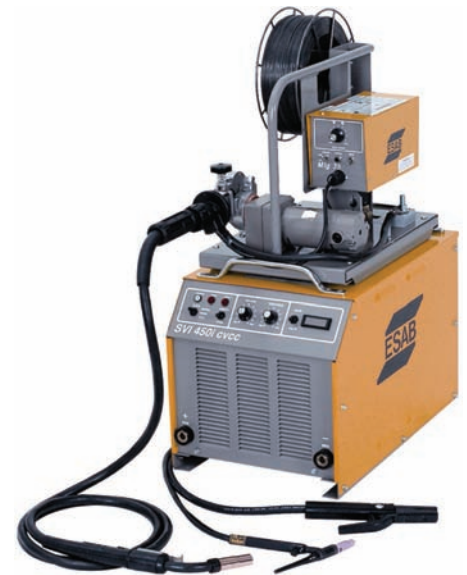
Fig. 23-8 Constant voltage and constant current, 350 ampere at 34 volts, 100 percent duty cycle machine with wire feeder. This power source is designed to operate off of single- or three-phase primary power and is a d.c. inverter machine weighing in at 150 pounds. With its variable inductance and selectable slope, it allows ultrafine tuning and improves arc characteristics for all types of GMAW modes of metal transfer plus FCAW, SMAW, and GTAW. © ESAB
