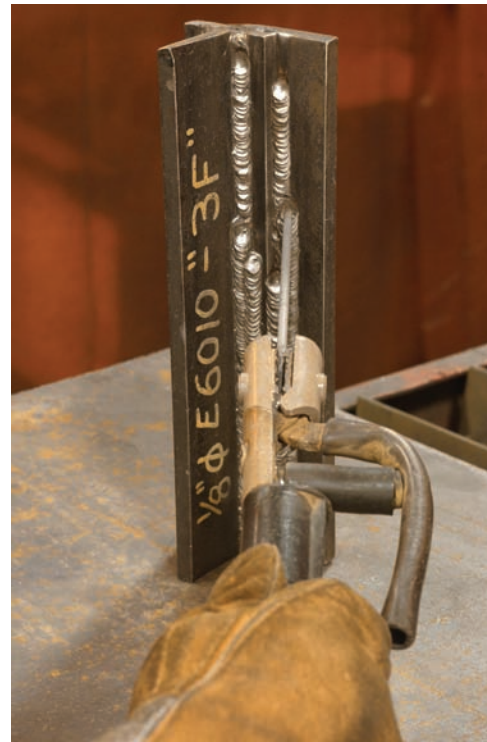
Fig. 14-39 Electrode and electrode holder positioned as instructed in Fig. 14-38. © Prographics
