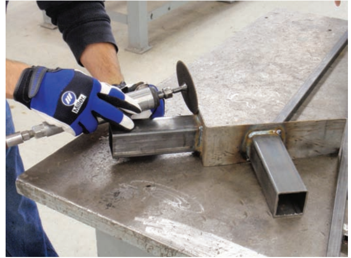
Fig. 26-59 A welding student using a pneumatic die grinder with a cutting disk to profile a weld. Because of the high speed 20,000 rpm and guarding issues this type work should be done with double eye protection. That is safety glasses along with a full face shield. Grinding should be done as an exception for poor weld profile at starts, stops, root passes and not as a rule because of poor welding technique which results in the entire weld having to be ground. © Renee Bohnart
