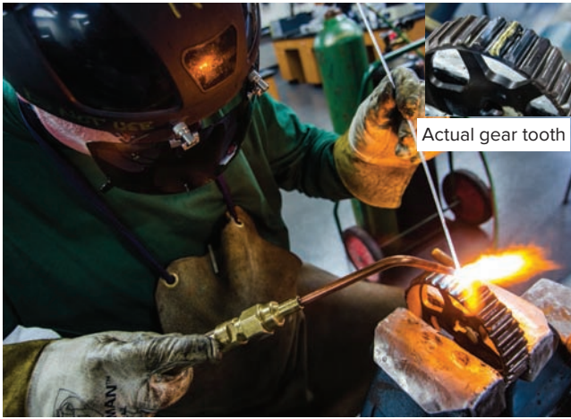
Fig. 2-1 A welding instructor demonstrates bronze repair of a damaged gear tooth on a sintered manufactured gear blank. Location: Northeast Wisconsin Technical College © McGraw-Hill Education/Mark A. Dierker, photographer
