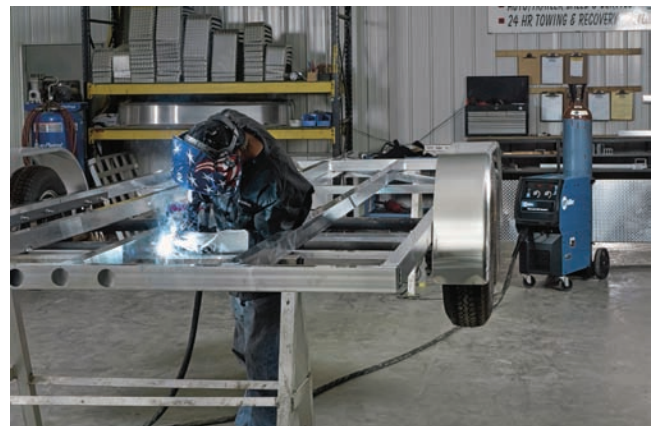
Fig. 21-29 Shop portable GMAW welding outfit includes 350-ampere c.v. single or three phase input inverter power source. It is equipped with up to 35 feet, of 200 amp push-pull aluminum gun. Note four wheeled cart and single gas cylinder of argon. As shown being used to weld an aluminum trailer frame. © Miller Electric Mfg. Co.
