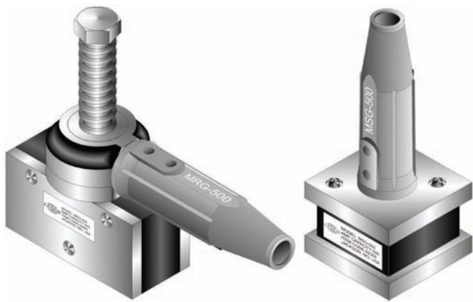
Fig. 26-13 Magnetic welding ground (work) connectors rated for 500 amps and designed to accept 3/0 and 4/0 welding cable. The rotating work connector on the left covers 12 square inches giving good stability on rotating weldments. It has 4 inches of current carrying contact surface. The model shown on the right is only a magnetic work connection not intended for rotating applications. © Lenco dba NLC, Inc.
