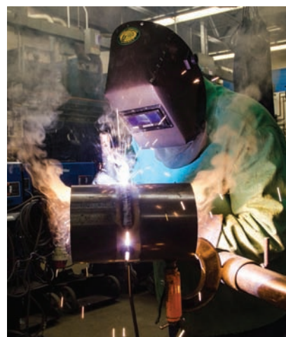
Fig. 16-9 This welding student is making a circumferential V-groove weld on a butt joint in pipe in the horizontal fixed position (5G). Location: Northeast Wisconsin Technical College © McGraw-Hill Education/Mark A. Dierker, photographer
