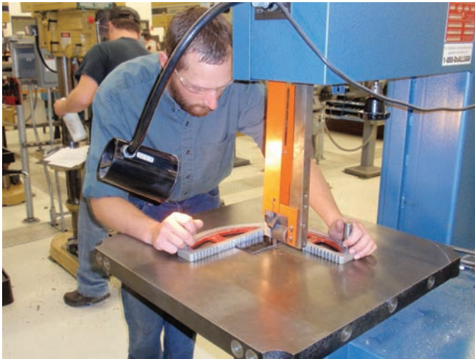
Fig. 26-85 Vertical band saw in use. Note the material handling tool to keep hands away from the blade and also the well-lighted work surface. © Renee Bohnart
