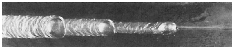
Fig. 13-63 Typical appearance of a multipass fillet weld in a T-joint welded in the flat position with DCEN shielded arc electrodes.
