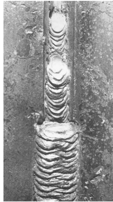
Fig. 15-50 V-groove butt test joint with a backup bar and a 1/4-inch root opening welded in the vertical position, travel up (3G). Note the sequence of weld beads and the appearance.
