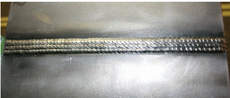
Fig. 22-21 GMAW final passes short circuit transfer on \frac{3}{8} -inch thick plate. Groove angle 60^\circ , SG-AC-25, and 0.035 wire diameter. Note the complete fusion, uniform bead width, location, and the ripple pattern created by the slight whipping motion. © Edward R. Bohnart
