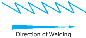
Fig. 24-28 Suggested pattern for gun manipulation in making the root pass for a 2G weld.
