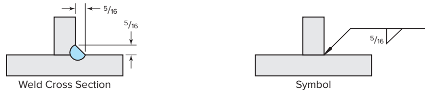
Size of Single-Fillet Weld
