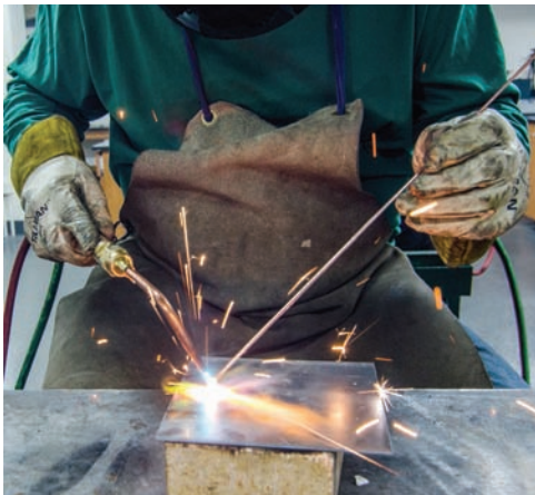
Fig. 8-14 Torch and filler rod position when welding in the flat position. The torch may also be held like a hammer. Location: Northeast Wisconsin Technical College © McGraw-Hill Education/Mark A. Dierker, photographer
