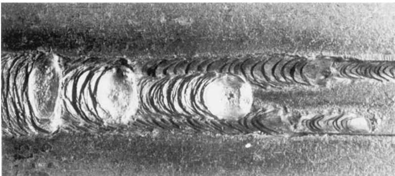
Fig. 15-64 Joint for the fillet weld soundness test welded in the overhead position (4F). Note the sequence of weld beads and the appearance.
