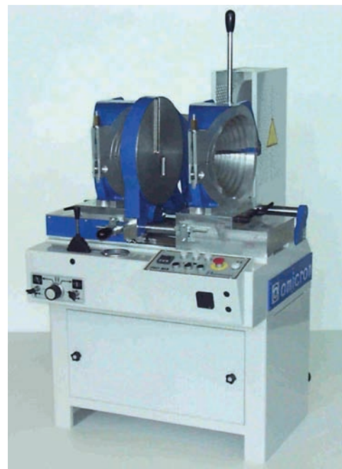
Fig. 31-7 A shop machine hot plate welding machine. It is suitable for PP, PE, PVC, CPVC, and PVDF. Ideal for fabrication of elbows, tees, laterals, and crosses. Sizes range up to approximately 24-inch pipe. Also capable of welding IPS, DIPS, PIP, and sewer materials. © Wegener
