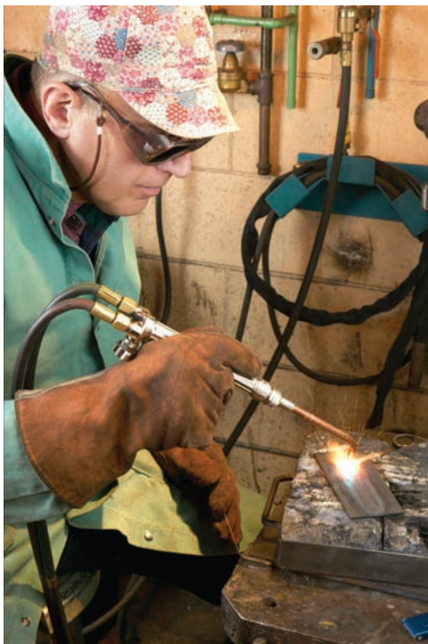
Fig. 8-9 Ripple welding. A light welding torch can be held like a pencil. A larger torch is held like a hammer. © Prographics
