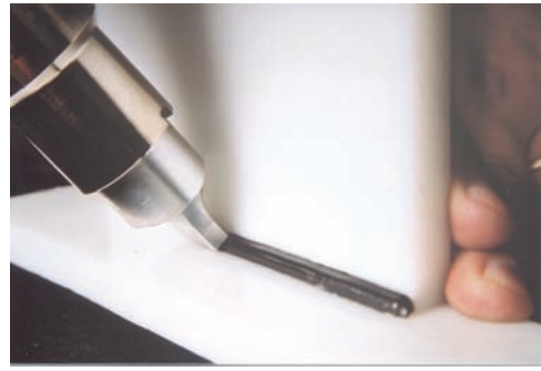
Fig. 31-9 Weld being made on inside of a corner joint with the injector welding machine. The one-hand operation frees up the hand for holding the plastic part in position. © Drader Manufacturing
