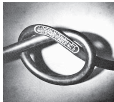
Fig. 11-21 Welding cable with thousands of fine wires has greater flexibility. A specially finished, durable paper wrapper allows the conductor to slip easily when the cable is bent.
