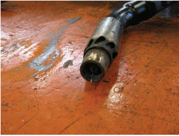
Fig. 32-21 GMAW-FCAW gun equipped with a smoke exhaust device. © NovaTech
