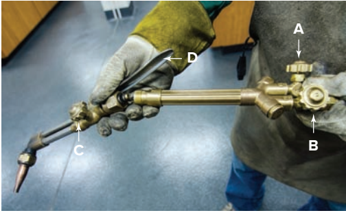
Fig. 7-37 Attaching an adaptable cutting head to the welding torch body. The welding torch may now be used as a cutting tool. Location: Northeast Wisconsin Technical College © McGraw-Hill Education/Mark A. Dierker, photographer
