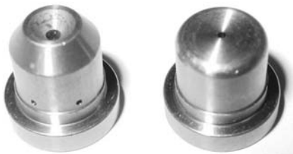
Fig. 17-32 Gouging tip and cutting tip comparison. © Miller Electric Mfg. Co.
