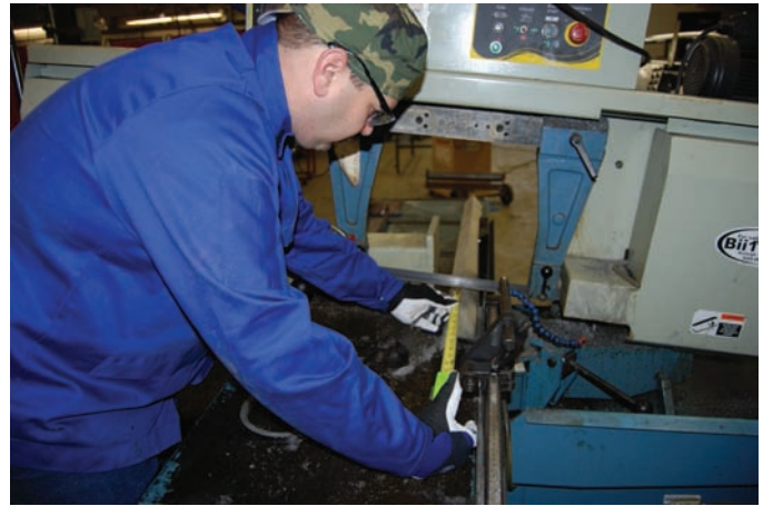
Fig. 26-86 Horizontal band saw in use. Once the angle iron length to be cut is measured and securely clamped in place, the saw blade guides will be repositioned as close as possible to the part being cut. © Renee Bohnart
