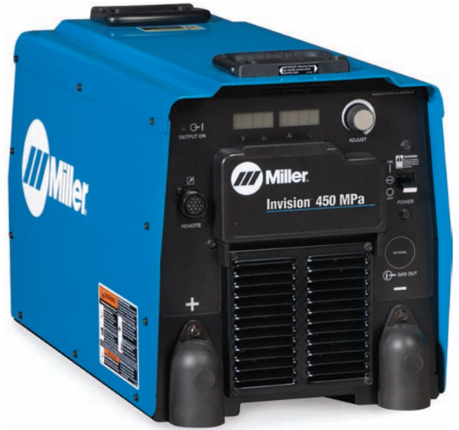
Fig. 21-23 A 450-ampere, d.c. constant voltage/constant current inverter power source. Capable of running all modes of gas metal arc transfers including pulse. A variable inductance control provides additional arc performance. © Miller Electric Mfg. Co.
