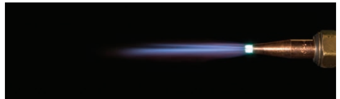
Fig. 7-32 Neutral flame with the cutting lever depressed. The cutting jet is straight and smooth. © David A. Tietz/Editorial Image, LLC
