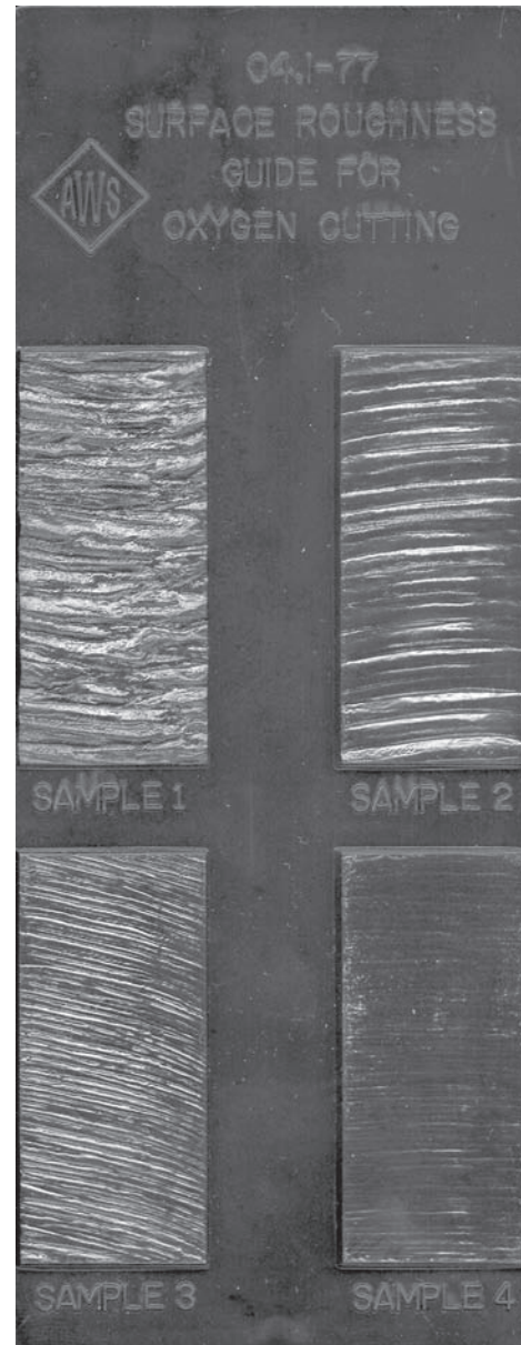
Fig. 7-42 Surface roughness guide for oxygen cutting. For materials up to and including 4 in. thick, Sample 3 should be used, and for materials over 4 in. and up to 8 in. thick, Sample 2 should be used. © American Welding Society. C4.6M:2006 (ISO 9013:2002 IDT), fig. C.8
