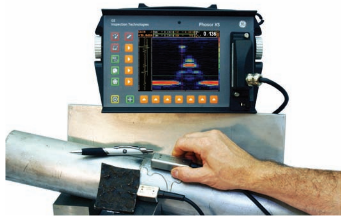
Fig. 28-43 Portable ultrasonic weld flaw detector with built-in trigonometric flaw location calculations with curvature correction and AWS D1.1 weld rating calculations. It combines a phased array imaging device and a conventional flaw detector into one instrument, with a phased array probe that allows significantly increased confidence in inspection data. Compared with traditional thickness gauge and flaw detector inspection, it offers greater probability of detection as well as faster and more reliable scanning. (left) © Agfa Corporation; (right) © General Electric Company
