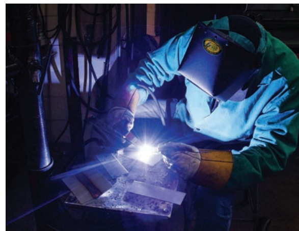
Fig. 19-13 Student is properly protected and is in the proper position for bench welding. Location: Northeast Wisconsin Technical College © McGraw-Hill Education/Mark A. Dierker, photographer
