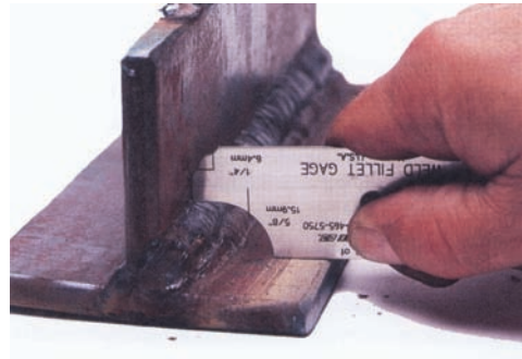
Fig. 4-51 Measuring fillet weld size. On the left, a concave fillet weld; on the right, a convex fillet weld. © American Welding Society. Welding Inspection Technology , 5th ed., p. 10–12, fig. 10.14; 2008
