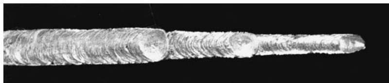
Fig. 13-64 Typical appearance of a multipass fillet weld in a T-joint welded in the flat position with a.c. type (E6013) shielded arc electrodes.
