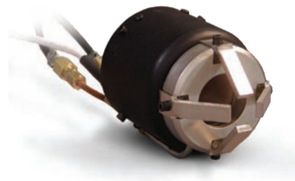
Fig. 27-3 Magnetic probe used in conjunction with control shown in Fig. 27-2. The probe mounts on the torch or gun and creates a magnetic field that precisely positions, oscillates, and stabilizes the arc. © ITW Jetline - Cyclomatic
