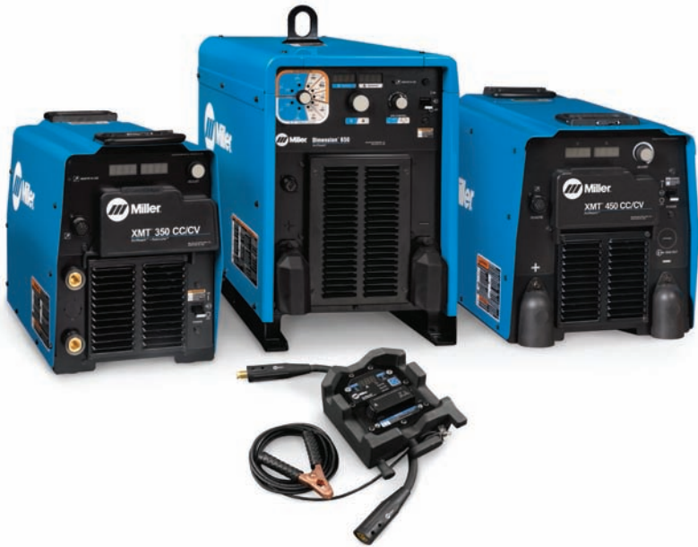
Fig. 23-7 Constant voltage/constant current family of d.c. welding machines. These are industrial rated machines at 100 percent duty cycle. Output ratings from 300 through 1,000 amperes are available to meet demanding needs. All the major processes like FCAW, SAW, GMAW, SMAW, and GTAW are capable with this type of equipment. These machines are capable of running ArcReach™ which allows control of the power source with the displayed remote control connected at the wire-feeder. © Miller Electric Mfg. Co.
