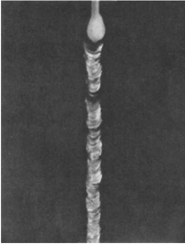
Fig. 14-56 Penetration and fusion through the root side of the outside corner joint shown in Fig. 14-57.
