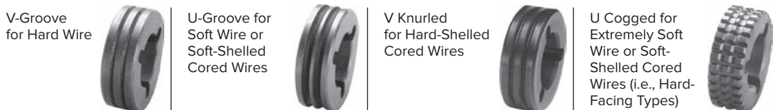
Fig. 21-39 Drive roll types and applications. © Miller Electric Mfg. Co.
