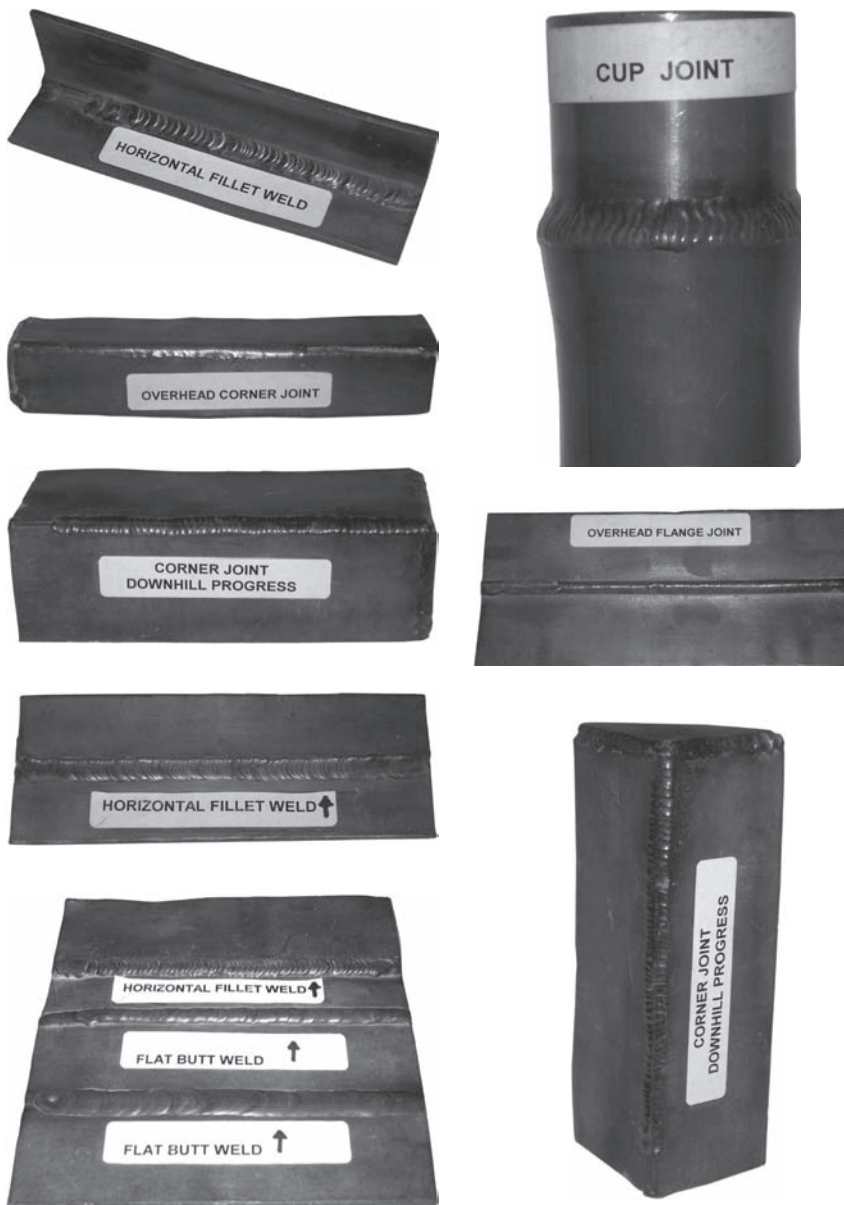
Fig. 9-12 Standard joint design in lead welding. It is possible to weld in all positions. © Tony DeMarco
