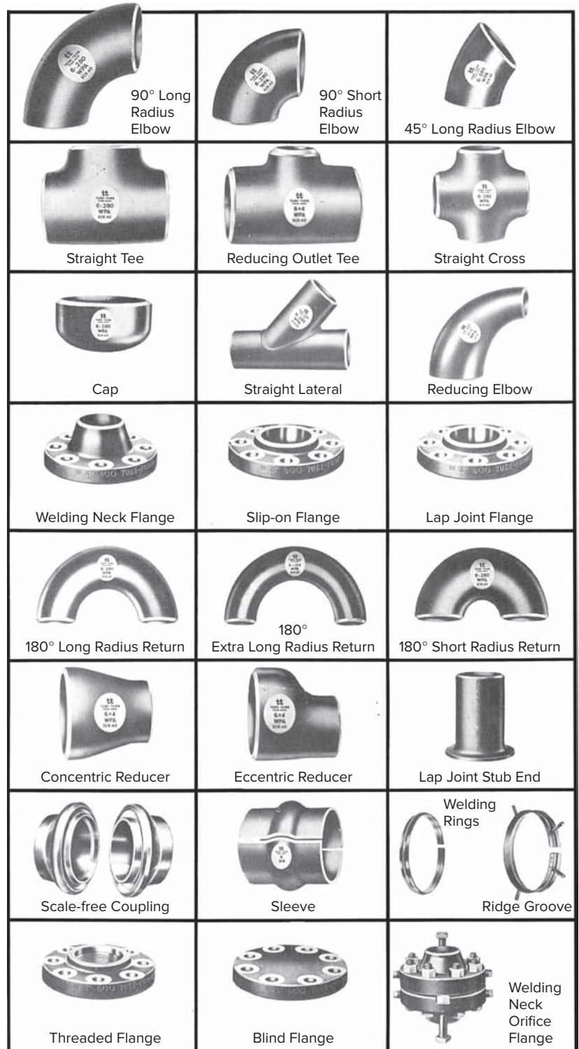
Fig. 16-12 Machine-beveled manufactured welding fittings. Source: Sypris Technologies, Inc.
