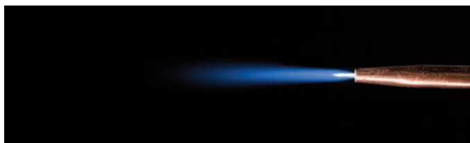
Fig. 8-7 Oxidizing welding flame commonly used for brazing with bronze rods. © David A. Tietz/Editorial Image, LLC
