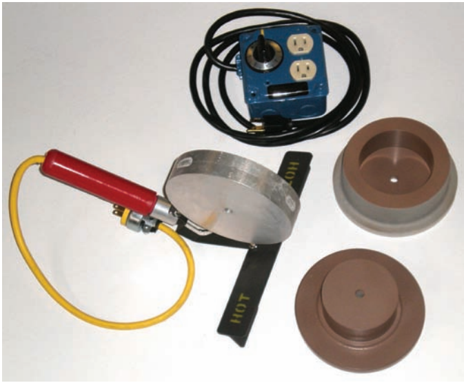
Fig. 31-38 Fusion pipe welding machine. Uses an electric tubular heater and is mounted on the clampable base. A stepless rheostat is used to control the heat. Can be used in shop or field for welding of PE, PP, and PVDF pipes and couplings. Two sizes are available from this manufacturer. One for 1/2–2 inch and another for 3–4 inch pipe. © Laramy Products Co., Inc.
