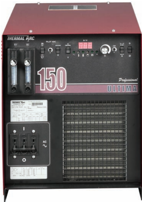
Fig. 18-60 A 0.5- to 150-amp PAW power source that will operate on 208- to 460-volt a.c. single- or three-phase power. It is equipped with interfaces for manual or automatic controls.
