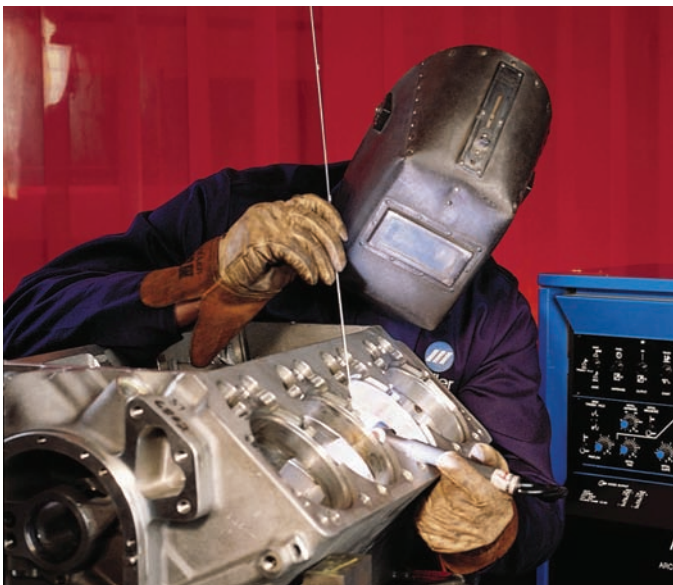
Fig. 18-2 Welding an aluminum cylinder with the gas tungsten arc process. © Miller Electric Mfg. Co.
