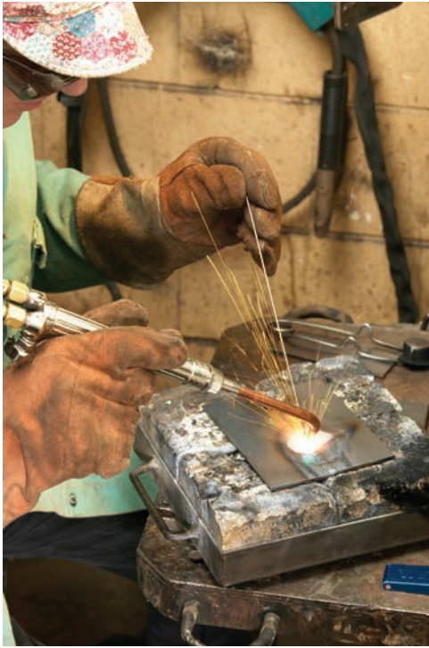
Fig. 8-13 Torch and rod being held as typical for right-handed welder. © Prographics
