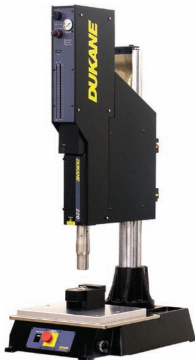
Fig. 31-6 Ultrasonic plastics welding machine available in 20, 30, 40, 50, and 70 kHz frequencies. They can be purchased as single units, stand-alone assembly systems, or incorporated into automated machinery. © Dukane
