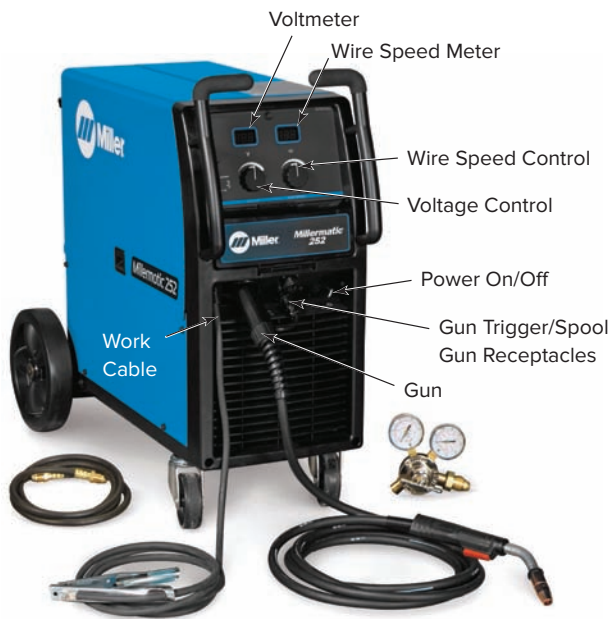
Fig. 21-19 Control panel of a typical 250 ampere constant current power source, wire-feeder combination with adjustable voltage and wire-feed speed control. With digital read out of voltage and wire-feed speed. Gas metal and flux cored arc capable. As well as aluminum welding with push pull or spool gun. © Miller Electric Mfg. Co.
