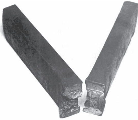
Fig. 28-84 A nick-break specimen after it has been broken for inspection of the weld deposit. A sound weld is free of slag and oxide inclusions and gas porosity and shows complete fusion.
