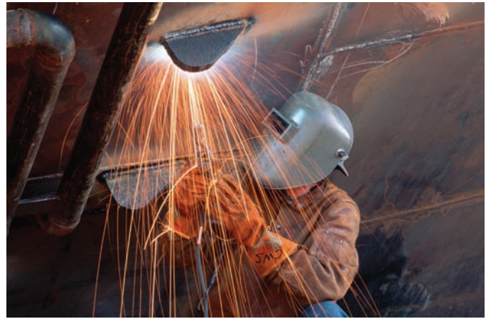
Fig. 2-28 Welder at work in shipyard. Note the overhead position and leather safety protection. © Kevin Fleming/Corbis/VCG/Getty Images
