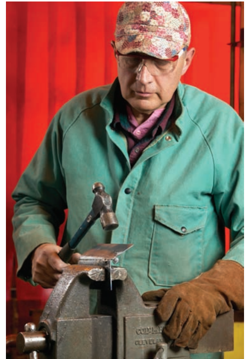
Fig. 8-30 Hammering welded square butt joint in vise positioned so that root of the weld is exposed to the most stress. © Prographics
