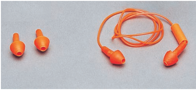
Fig. 32-11 Earplugs with a collapsible air cavity design. They have a noise reduction rating of 24.0 dB and are nontoxic, hypoallergenic, and reusable and can be washed in warm water with mild soap. They meet ANSI S3.19 specifications. © Sellstrom Manufacturing Company
