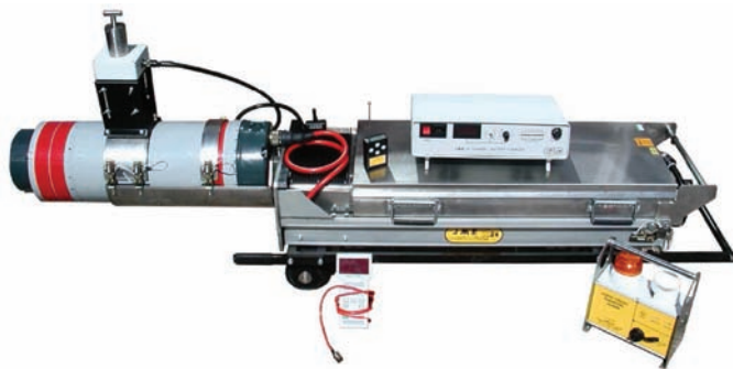
Fig. 16-42 Smart pigs come in a variety of designs and capabilities. They are typically able to inspect pipe from 6 to 72 inches in diameter with either gamma or X-ray inspection techniques. These crawlers are available to meet quality and rigid production quotas. Operators must be qualified and well-experienced. © Shaw Pipeline Services
