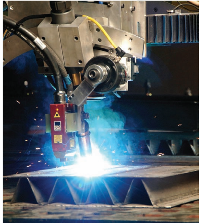
Fig. 27-13 A precision laser sensor and laser vision camera for applications in the shipbuilding industry. AUTO-TRAC is for seam finding, seam tracking, and adaptive control for hard automation (special-purpose CNC machines) welding processes like GMAW being shown here. It is capable of detecting weld slope, mismatch, undercut, bead width, convexity, open porosity, pinholes, and metal drops. The laser profiler acquisition rate is 16,000 points per second while the sensor acquisition rate is 2,000 Hz allowing it to easily keep up with the hybrid laser/GMAW process. Advantages of laser vision-based seam tracking systems over mechanical probes, human adjustments, or other means include optimized adaptive welding parameters, extremely accurate wire positioning, no material damage due to contactless sensing, preweld joint variation information, and a perfect overlap for cylindrical parts required to be leakproof. It is designed for precise torch positioning, the modular components allow for Ethernet connectivity, and the adaptive software module can be interfaced directly to the welding equipment. All this makes for faster welding speeds, decreases the amount of operator monitoring, lessens intervention requirements, reduces tooling cost, and increases quality and productivity with no mechanical probe parts to replace. © Servo-Robot Corp.
