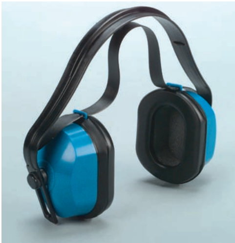
Fig. 32-12 Earmuffs that feature polyfoam ear cushions for extra comfort. They have a noise reduction rating of 21.0 dB and when used with earplugs, as shown in Fig. 32-11, provide for very effective hearing protection. They meet ANSI S3.19 specifications. © Sellstrom Manufacturing Company
