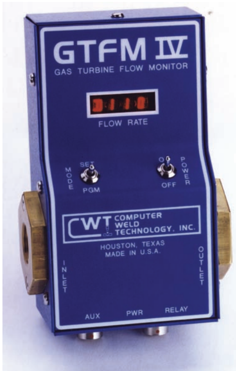
Fig. 27-11 Gas turbine flow monitor precisely measures the flow rate of welding gases. It can be used for argon, helium, CO 2 , or any mixed inert welding gas. Flow rates can be digitally displayed from 5 to 255 SCFH in 1 SCFH increments. The accuracy of the 1 percent of full scale reading is much better than a conventional ball-type flowmeter. © Computer Weld Tech., Inc.
