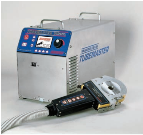
Fig. 18-38 This orbital welding equipment has an all-digital programmable portable power source rated at 200 amps. It has repeatability, precision, and QA/QC verification possibilities. Note the weld head, which makes fusion, welds meeting aerospace, pharmaceutical, food processing, and instrumentation quality requirements. © Magnatech Limited Partnership
