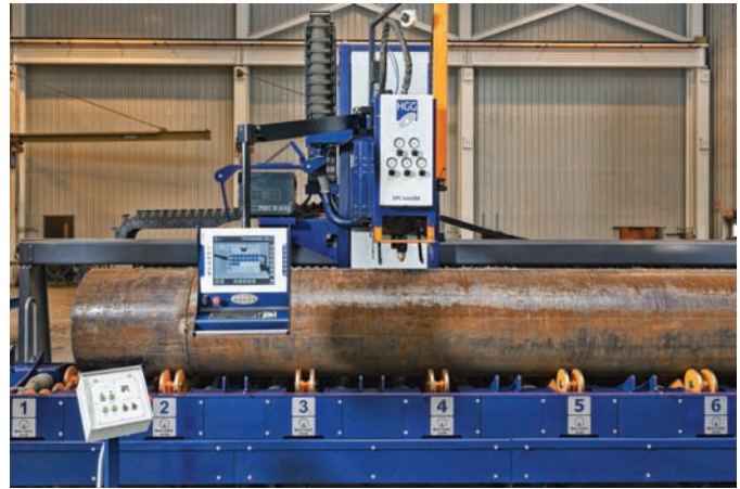
Fig. 17-20 This custom control system will closely track all pipe spools throughout the production process, from the isometric drawing to shipment. It can pinpoint materials shortages, allocates material to each pipe spool as required while tracking man-hours required. Automated systems like this are required to speed production and delivery while ensuring the accuracy of each pipe spool. © Team Industries, Inc.
