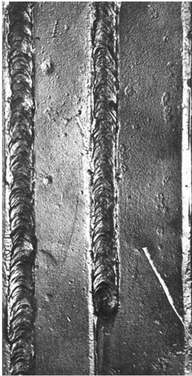
Fig. 13-50 Typical appearance of a fillet weld in a lap joint welded in the vertical position, travel down, with DCEN or a.c. shielded arc electrodes.
