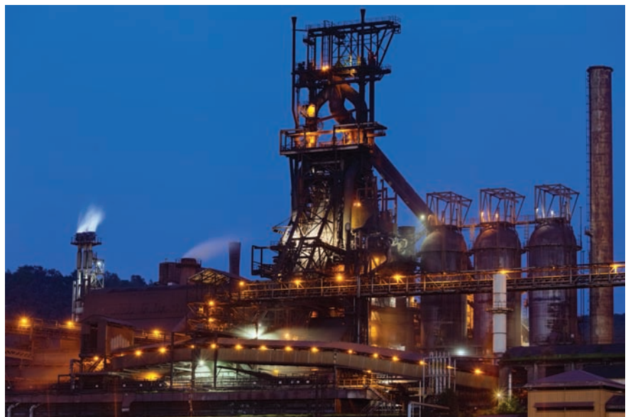
Fig. 3-8 In a blast furnace operation, new charge enters from the top while liquid iron and slag are drawn away below. © Thomas Saupe/Getty Images
