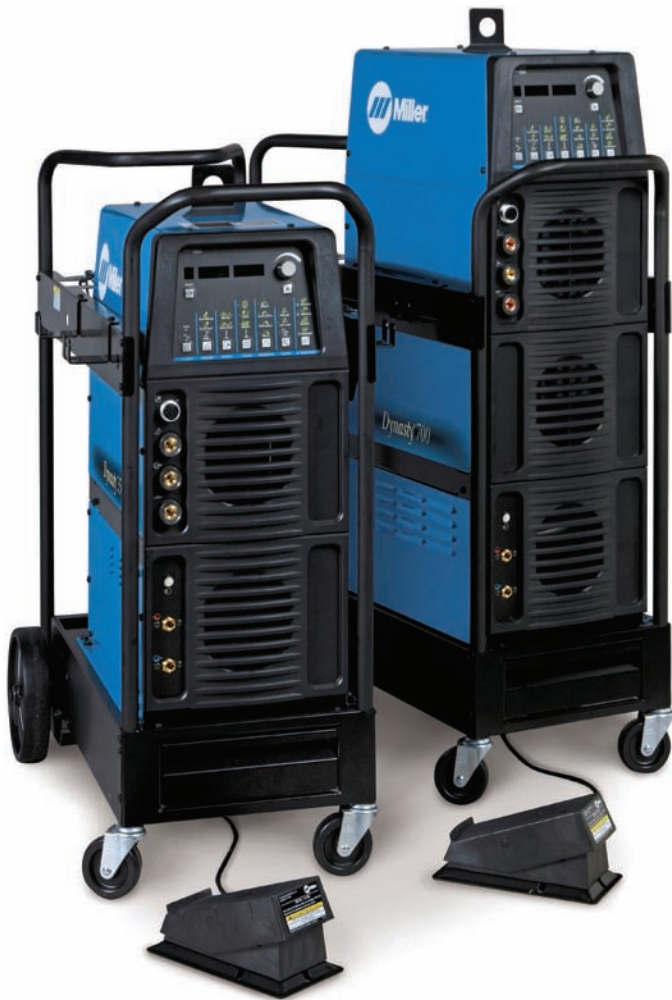
Fig. 18-23 How well the arc can be controlled is important when selecting equipment. The welder must be able to shape the arc and control the weld bead. Miller's Aerowave 300 (an a.c.-d.c. power source) features advanced square wave arc, independent current control, adjustable frequency, a.c. balance control, and lift arc for TIG arc starts. Examples of industrial uses of this machine include aerospace, tube and pipe manufacture, bicycle assembly, fillet welds, and automation. © Miller Electric Mfg. Co.
