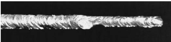
Fig. 14-60 Typical appearance of a multipass fillet weld in a T-joint welded in the horizontal (2F) position with shielded metal arc, low hydrogen, iron powder, coated electrodes (DCEP or a.c.).
