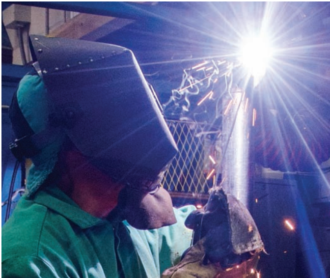
Fig. 14-1 Making a weld in the vertical (3) position. Note the protective clothing. Location: Northeast Wisconsin Technical College © McGraw-Hill Education/Mark A. Dierker, photographer
