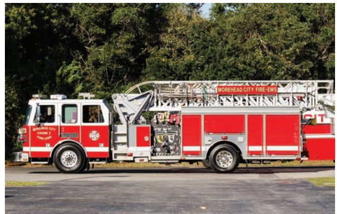
Fig. 2-6 These life- and property-saving vehicles must perform in all types of conditions. Welding plays an essential role in their manufacture. Carbon steel, stainless steel, and aluminum are all typically used in fire-fighting vehicles. Location: Northeast Wisconsin Technical College © McGraw-Hill Education/Mark A. Dierker, photographer
