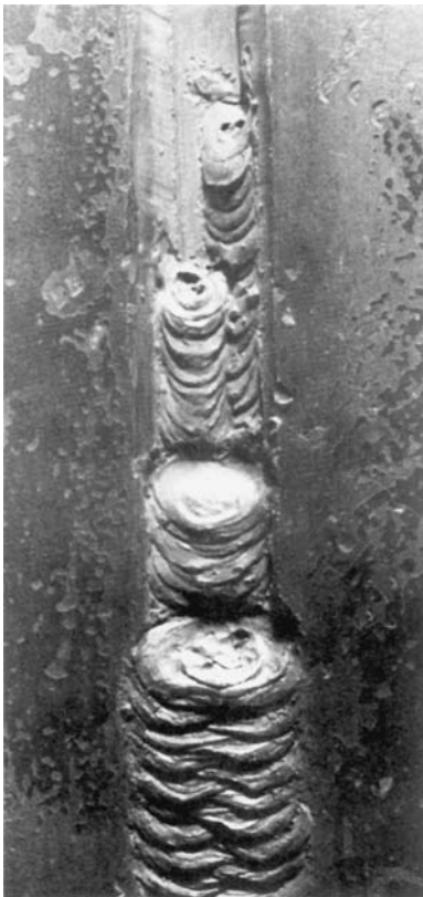
Fig. 15-54 V-groove butt test joint with a backing bar and a \frac{3}{8} -inch root opening welded in the vertical position, travel up. Note the sequence of weld beads and the appearance.
