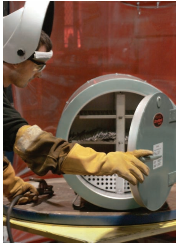
Fig. 12-11 An electrically heated shop electrode oven. This oven has the capacity to hold 350 pounds of 18-inch electrodes. It is equipped with a thermostat control with a temperature range from 100°F to 550°F. © Phoenix International
