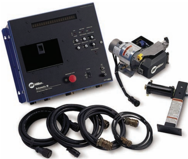
Fig. 27-19 Microprocessor-based weld control for automatic systems and robots lacking weld control capability. This model is ready to operate, with eight preprogrammed synergic pulse (adaptive/nonadaptive) programs that can be easily customized. Additional memory space and the ability to transfer data from one control to another is available on data cards. The unit features 17 dedicated inputs, 14 dedicated outputs, and two user-defined outputs. A quick disconnect allows easy interface with PLC or other control systems. This controller comes with interconnecting cables, wire drive head, and wire supply support assembly. © Miller Electric Mfg. Co.
