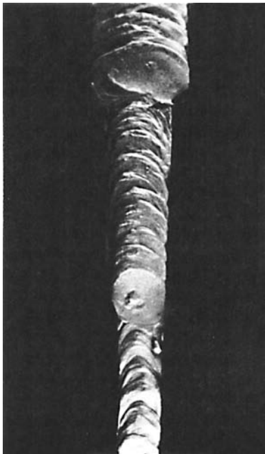
Fig. 24-46 Face appearance of root, filler, and cover passes, welding with pipe axis horizontal and fixed. Weld was made in the 5G position downhill. Travel was somewhat slower than welding shown in Fig. 24-45 so welds are heavier. © Plumbers and Pipefitters Union, Alton, IL
