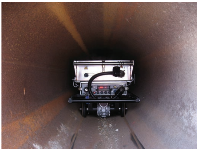
Fig. 16-43 The smart pig is located in the pipe and is making its way into position to radiograph a girth weld in a cross-country pipeline. Signals are sent to the crawler at each weld being inspected. © Shaw Pipeline Services
