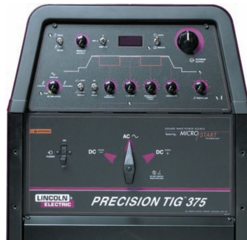
Fig. 18-37 A 375-ampere a.c.-d.c., constant current transformer with solid-state controls and square wave output. This machine can be used for a.c.-d.c. TIG and a.c.-d.c. stick electrode welding. Note the accessories and the cart with built-in water cooler. © Lincoln Electric
