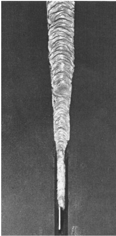
Fig. 15-21 Typical appearance of a multipass groove weld in a V-groove butt joint without a backing strip welded in the vertical position, travel down, with DCEP or a.c. shielded arc electrodes.
