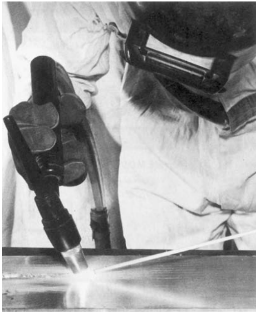
Fig. 19-18 Correct positions of the torch and filler rod at the start of bead welding. © Kaiser Aluminum
