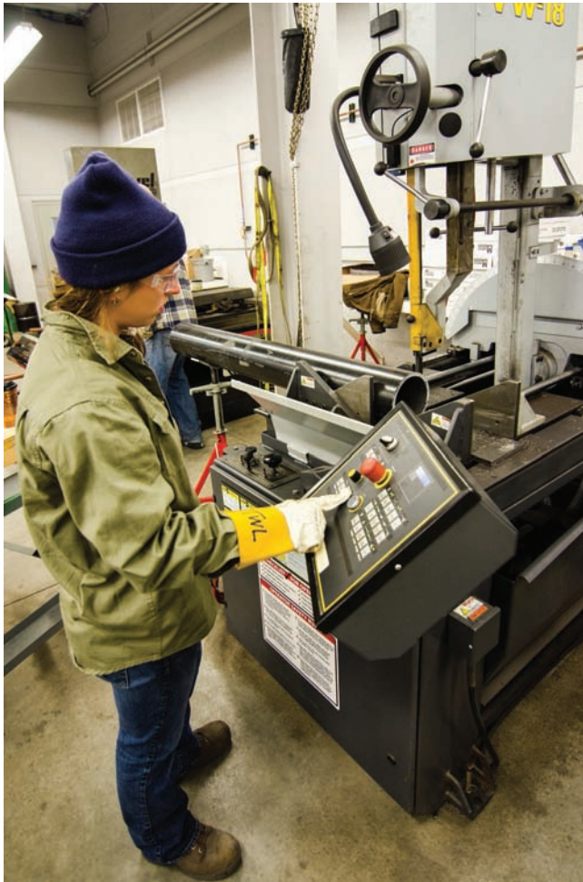
Fig. 16-92 Welding apprentice using a digital control panel to cut pipe practice coupons on a power feed vertical band saw. Location: UA Local 400 © McGraw-Hill Education/Mark A. Dierker, photographer
