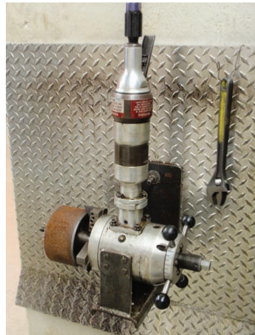
Fig. 26-65 This 80 lb. BevelMaster by Tri Tool is designed to handle pipe from 4–12 inches in size with wall thicknesses up to 1.32 inches. It is pneumatic and requires 85 cfm at 90 psi. At this school it is mounted and the short pipe nipples are brought to the machine. Lighter units are available for application where the bevel machine must be brought to the pipe. © Renee Bohnart
