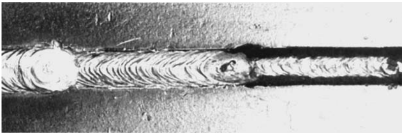
Fig. 14-34 Joint construction and typical appearance of a multipass single V-groove weld in a butt joint welded in the flat position with DCEP or a.c. shielded metal arc electrodes.
