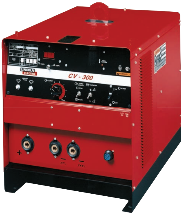
Fig. 21-22 A 300-ampere d.c. constant voltage transformer-rectifier with solid-state control and built-in predetermined slope control. © Lincoln Electric
