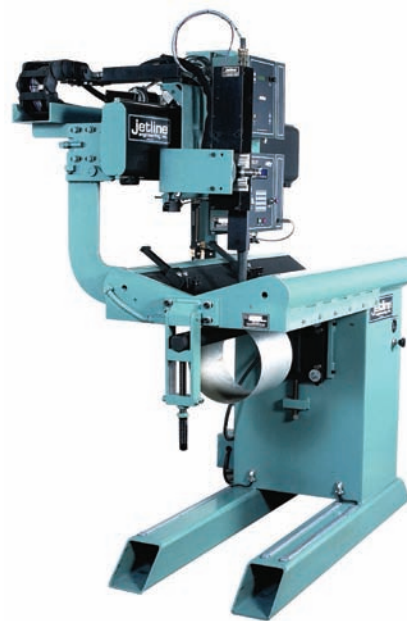
Fig. 26-14 Seamers of this type are available for lengths from 24 inches to 10 feet. Some models can clamp materials as thin as 0.005 inch and with linear accuracy of 0.005 inch over 10 feet for high precision capability. © ITW Jetline - Cyclomatic
