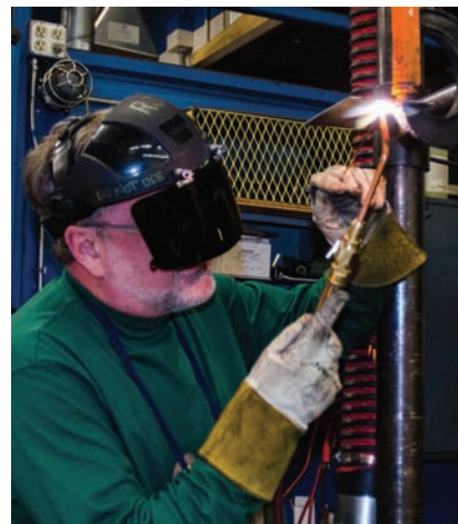
Fig. 8-23 Welding in the overhead position on steel plate. A small torch and steel filler rod are used. Location: Northeast Wisconsin Technical College © McGraw-Hill Education/Mark A. Dierker, photographer
