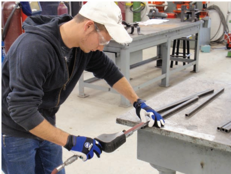
Fig. 26-58 A welding student using a pneumatic belt sander to remove burs on some square tubing. The belt is approximately ½ inch wide and 24 inch long and is moving at 20,000 r.p.m. © Renee Bohnart
