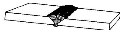
Fig. 31-29 Single V-groove weld for butt joints welded from one side only. Source: Kamweld Products Co.
