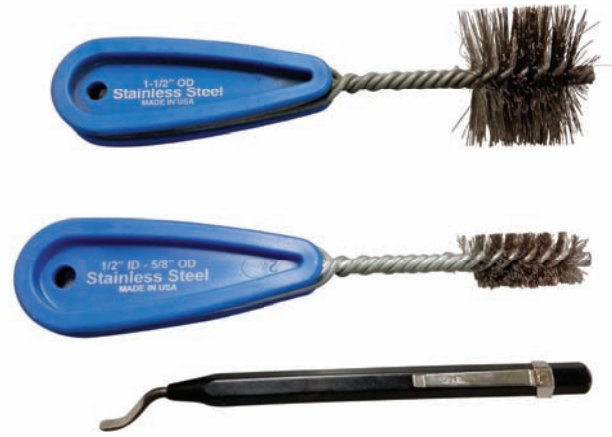
Fig. 10-10 Remove the burr on the inside of the pipe with the deburring tool shown below. Then clean with the wire brushes. Location: UA Local 400 © Edward R. Bohnart, Photographer
