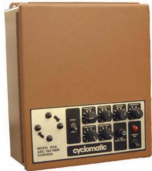
Fig. 27-2 This unit controls the sweep frequency, sweep amplitude, arc position, dwell time (on each toe), and shaping via the magnetic probe. © ITW Jetline - Cyclomatic
