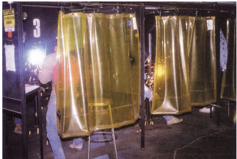
Fig. 32-1 A welding shop with individual stations. Note that the welding cables are suspended so that they are free of the floor and weld curtains protect between booths. © Wilson Industries, Inc.
