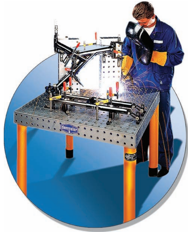
Fig. 26-4 Modular tooling being used to hold an irregular shape for welding. © Bluco Corporation
