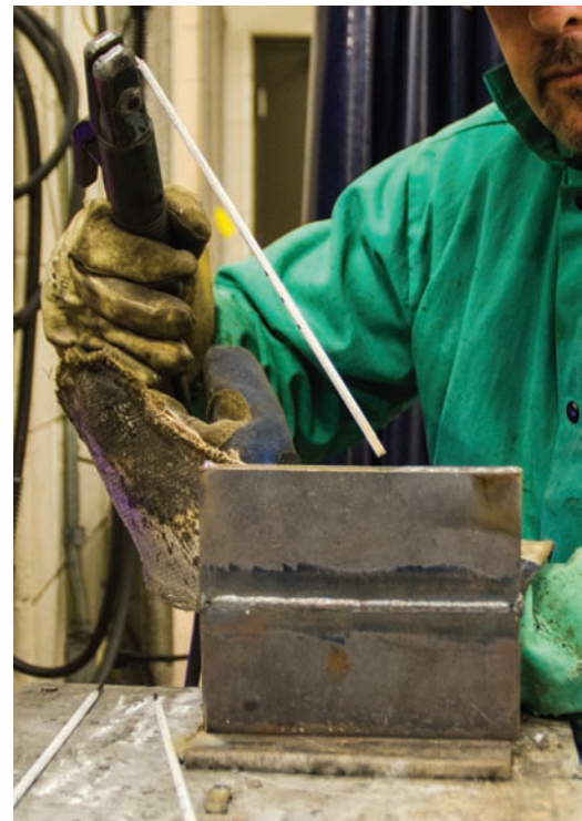
Fig. 13-27 Welding an edge joint. The electrode and electrode holder are positioned as instructed in Fig. 13-26. Location: Northeast Wisconsin Technical College © McGraw-Hill Education/Mark A. Dierker, photographer
