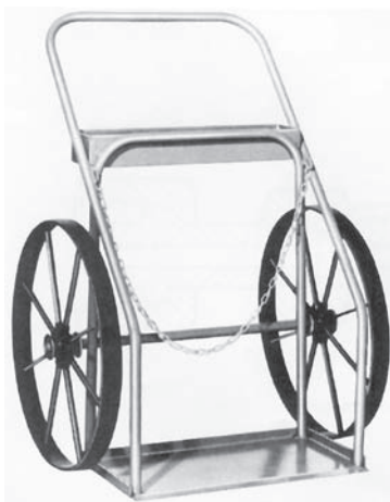
Fig. 5-19 Steel handtruck used to carry oxygen and acetylene tank and welding equipment. A portable outfit offers wide flexibility in the use of gas welding in both shop and field. © Thermadyne Industries, Inc.
