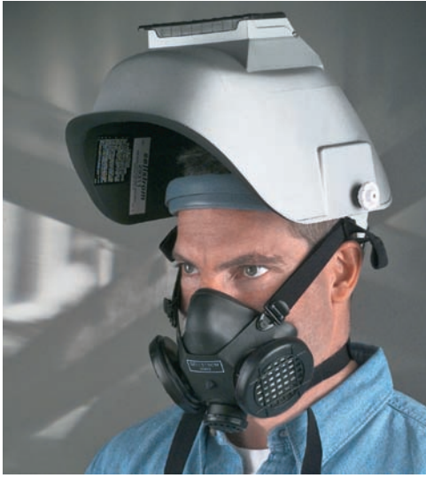
Fig. 32-14 A neoprene half-mask respirator facepiece. The soft nature of neoprene provides a comfortable fit and seal. These facepieces are available in various sizes and must be properly fitted. They comply with NIOSH 42 CFR Part 84 standard. © Sellstrom Manufacturing Company
