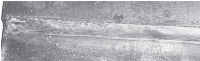
Fig. 23-27 Lap joint in \frac{3}{8} -inch mild steel plate welded in the flat position. The horizontal fillet weld was made in a single pass with flux cored filler wire \frac{3}{32} inch in diameter. Welding required 450 amperes and 32 volts.
