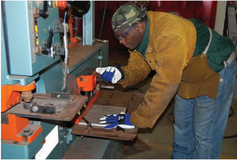
Fig. 26-46 A welding student is using a squaring shear on an ironworker to create some practice plates for welding. Plate up to 10 inches wide and \frac{3}{8} inch thick can be sheared on this 50 ton capacity machine. These type machines are capable of doing much more than just square shearing. © Renee Bohnart
