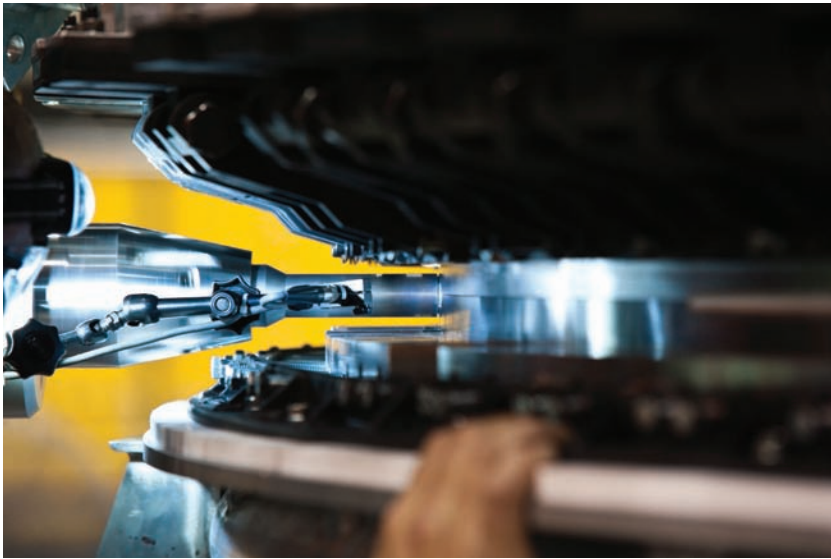
Fig. 2-5 An automatic friction stir welding machine weld being observed on an aerospace component. NASA
