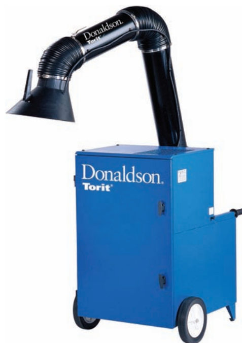
Fig. 32-13 In confined areas, where ventilation is restricted and/or ceiling height is not sufficient, fumes can be removed with extractor equipment. The advantage of this type of equipment is that the cleaned air is returned to the environment, thus reducing heating and cooling expenses. Note the position of the pickup arm. Do not position the pickup arm to draw the fumes around your head. Extractor equipment can be equipped with an in-hood light and in-hood remote power switch. © Donaldson Company, Inc.
