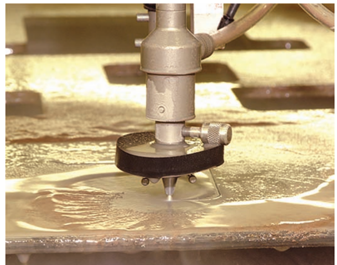
Fig. 26-89 Water jet being used to cut a gear out of a plate. © ESAB
