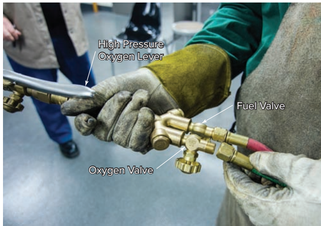
Fig. 7-25 Connecting the oxygen hose to the oxygen outlet on the cutting torch. The fuel hose is already connected. Location: Northeast Wisconsin Technical College © McGraw-Hill Education/Mark A. Dierker, photographer
