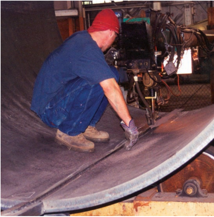
Fig. 23-34 Mechanized Submerged Arc Weld Made on a Bridge Pile Casing. Note the starting and or run off tab. These tabs assure good weld soundness at the ends of the production joint. © American Welding Society
