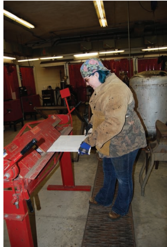
Fig. 26-40 A welding student bending a part in hand bending brake. © Renee Bohnart
