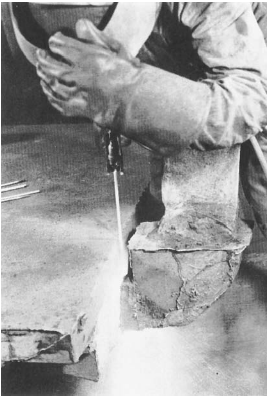
Fig. 17-19 The oxygen arc cutting of cast iron risers in the foundry. Risers are 5 inches square. The operation required 5 minutes cutting time. © Arcos Corp.
