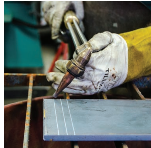
Fig. 7-41A Position of the cutting torch when making bevel cuts in the flat position. Location: Northeast Wisconsin Technical College © McGraw-Hill Education/Mark A. Dierker, photographer
