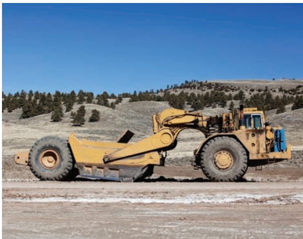
Fig. 2-10 A scraper bowl that can move up to 44 cubic yards of earth. © iStock/Getty Images Plus
