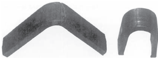
Fig. 28-79 Face-bend specimens. The specimen on the right withstood the test satisfactorily whereas the specimen on the left cracked and failed before the bending could be completed.
