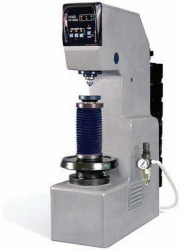
Fig. 28-54 A bench model Brinell hardness tester. This unit is capable of applying eight standard Brinell loads. © Newage Testing Instruments, Inc.
