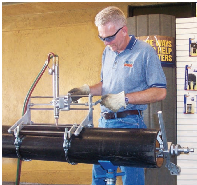
Fig. 16-47 A test coupon cutter used in the field for quick, on-the-spot testing. © Mathey Dearman
