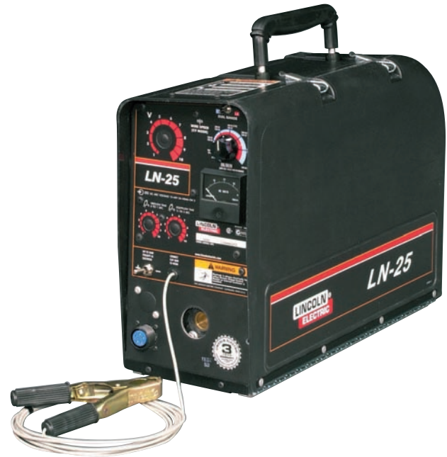
Fig. 21-38 This voltage sensing feeder is powered across the arc by the welding current. As with all voltage sensing feeders no control cables are needed. To operate, simply connect the weld cable and attach the work clip, and the feeder is ready to weld. This portable unit is designed for MIG/MAG or flux cored wire diameters of 0.023 to \frac{5}{64} inch with a wire-feed speed range from 50 to 700 inches per minute. The totally enclosed case accepts 10- to 44-pound wire packages. The feeder dimensions are 16 × 15 × 31 inches with a net weight of 65 pounds. © Lincoln Electric
