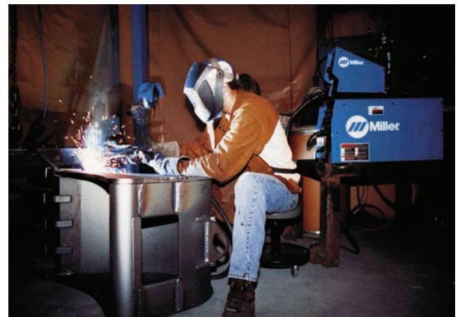
Fig. 22-19 Typical gas metal arc welding station in industry. Note the inverter power source with microprocessor-based wire-feeder/controller on this steel back-hoe bucket. © Miller Electric Mfg. Co.
