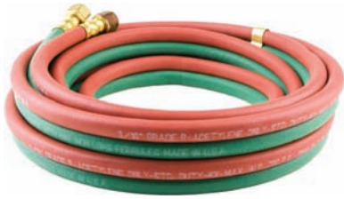
Fig. 5-32 Gas welding hose with fittings attached. It is a \frac{3}{16} -inch diameter. The diameter is determined by the volume of gas required and the length of the hose. Red is the fuel gas hose while green is the oxygen hose. © David A. Tietz/Editorial Image, LLC
