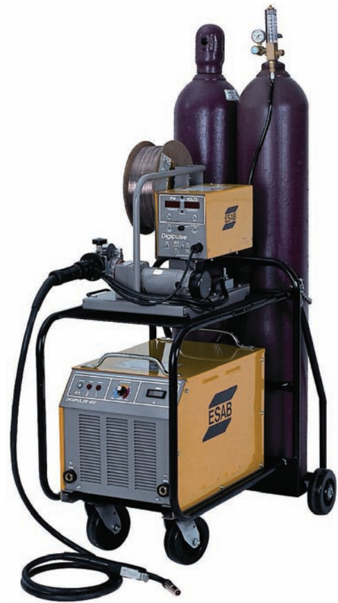
Fig. 21-32 This 450-ampere d.c. inverter power source uses the digital microprocessor-based feeder for standard MIG synergic programming of the following wire sizes: 0.030, 0.035, 0.045, 0.052, and \frac{1}{16} in. The following wire types are also preprogrammed: steel, alternate steel, stainless steel, 4000 aluminum, 5000 aluminum, and silicon bronze. This power source is also multiprocess capable as it can output both c.v. and c.c. © ESAB
