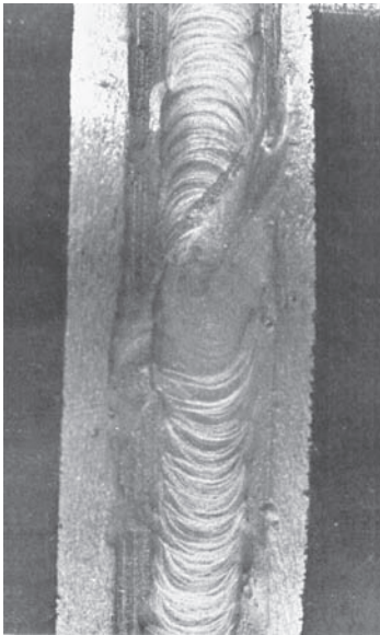
Fig. 20-23 Face of a root pass that shows proper termination where the bevels meet. This is a V-groove butt joint in stainless-steel pipe.
