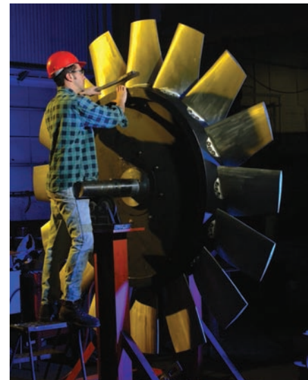
Fig. 2-42 Turbine blades being inspected and adjusted. These types of devices travel at very high velocities and at extreme temperatures. Welding plays an important role in the fabrication of the turbine blades and housings. Issues with dissimilar metals and superalloys must be considered. © Howden Buffalo Inc.
