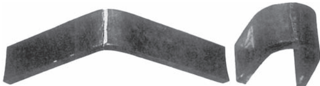
Fig. 28-80 Root-bend specimens. The specimen on the right withstood the test satisfactorily whereas the specimen on the left cracked and failed before the bending could be completed. Note the full penetration in the specimen that passed.
