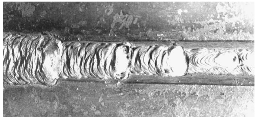
Fig. 15-55 V-groove butt test joint with a backing bar and a \frac{3}{8} -inch root opening welded in the overhead position (4G). Note the sequence of weld beads and the appearance.
