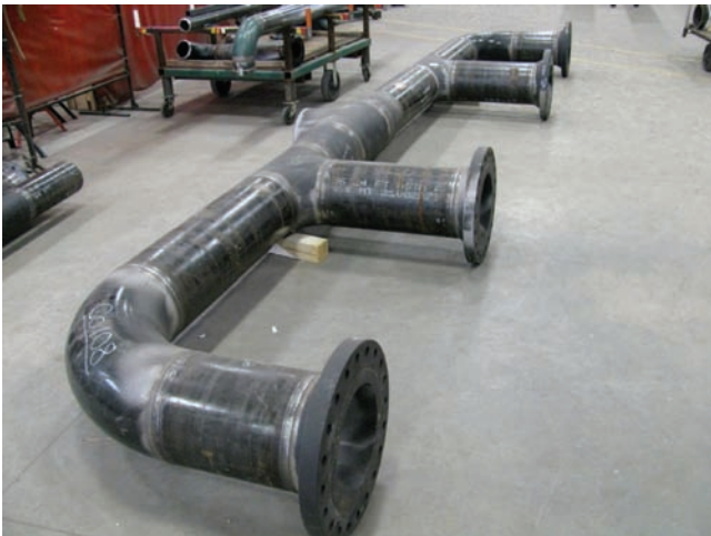
Fig. 16-78 A manifold with two elbows, 3 Tees, and 4 flanges. This type pipe spool must accurately bolt into position as specified on the drawings. While meeting all the weld acceptance criteria per code. © Piping Systems, Inc.
