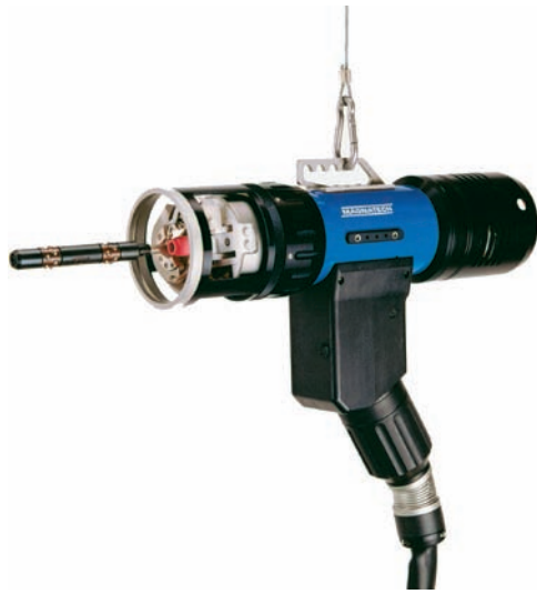
Fig. 26-27 This style head is for tube-to-sheet seal welding applications for boilers and heat exchangers. GTA welds can be made autogenously or with filler metals. Various tube to head joint geometries can be accommodated such as the tube and head flush, extended, or recessed. © Magnatech Limited Partnership
