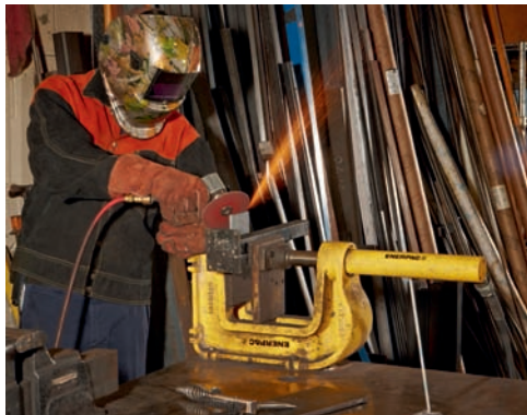
Fig. 26-35 A welder with a hydraulic C-clamp. Using proper safety precautions. © Enerpac Inc.
