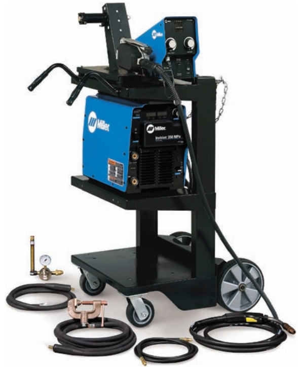
Fig. 24-6 A 300 amp d.c. inverter power source, constant speed wire feeder/controller, and shielding gas cylinder. This setup is light-weight and very portable. It is capable of running off of a variety of primary voltages and with either single or three-phase power. © Miller Electric Mfg. Co.
