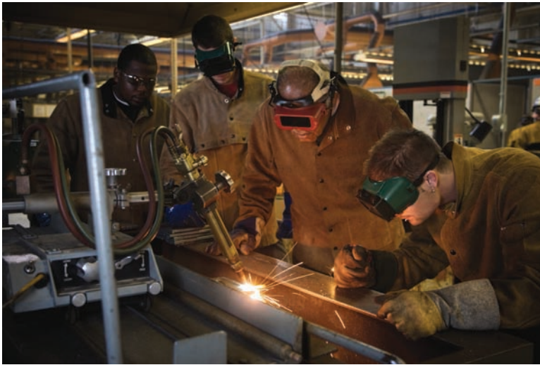
Fig. 7-1 These young welders are being observed by their instructor as to the proper procedure for cutting a bevel on a flat bar. A track type cutting machine is being used. Note the PPE being used. © Hill Street Studios/Blend Images/Getty Images
