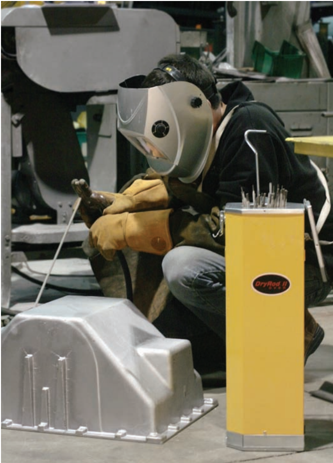
Fig. 12-9 The electric dry-rod electrode oven on the job. © Phoenix International
