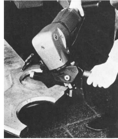
Fig. 26-64 A portable electric beveling tool. It can cut along straight edges, convex and concave curves, and circles. The machine’s capacity is ⅝ inch for single-V bevels and 1¼ inch for K- or double-K bevels. © Renee Bohnart
