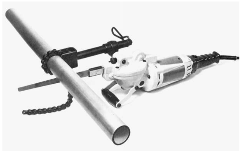
Fig. 16-88 A portable power hacksaw has the advantages of being light and highly portable. This one is shown with 3-inch stainless-steel pipe.
