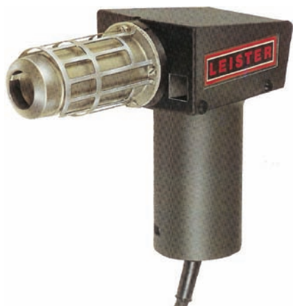
Fig. 31-4 Heat gun used for forming plastics and other plastic work. Weighs only 2¾ pounds, has adjustable air intake, with a 1¾-inch diameter nozzle. Is equipped with a 6-foot power cord and a toggle on-off-cold switch. © Malcom
