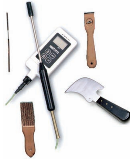
Fig. 31-34 Typical tools used for making plastic welds: (1) scraper, (2) moon knife, (3) roller, (4) temperature gauge, and (5) wire brush. © Wegener
