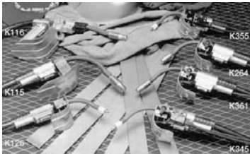
Fig. 21-48 FCAW-S guns rated from 250 to 600 amperes. Note the exposed contact tips on the guns set up for short electrode extension electrodes and the insulated guide tubes on other guns for the long electrode extension electrodes. Use the appropriate gun setup per the manufacturer's specification for the FCAW electrode extension being used. © Miller Electric Mfg. Co.
