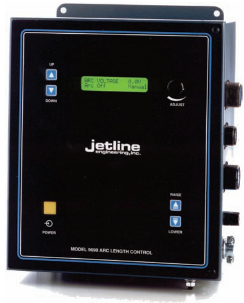
Fig. 27-7 Arc voltage control helps maintain the proper arc length at high speed on material with uneven surfaces, or when total adaptive control of this important variable is required for automatic welding. © ITW Jetline - Cyclomatic
