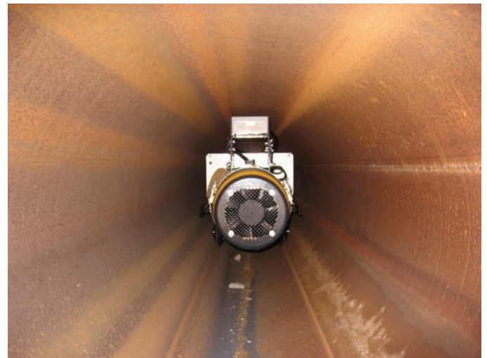
Fig. 16-43 The smart pig is located in the pipe and is making its way into position to radiograph a girth weld in a cross-country pipeline. Signals are sent to the crawler at each weld being inspected. © Shaw Pipeline Services
