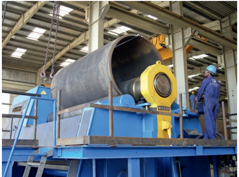
Fig. 26-37 A hydraulic bending machine with a capacity of 12 ft \times \frac{3}{4} -inch thick mild steel. The machine is bending 8 ft \times \frac{1}{2} -inch stainless-steel plate. Note the use of the hydraulic loading support. © Baileigh Industrial, Inc
