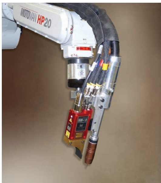
Fig. 27-24 Articulated robot arm fitted with laser camera for seam tracking and seam finding, and capable of doing weld inspection. This robot cell, along with a laser camera, provides real-time joint tracking, adaptive control, and visual inspection system integrated with Servo-Robot advanced 3-D laser vision techniques and advanced sensing devices. One benefit of the unique hybrid sensor technology is that it can dramatically speed up and simplify applications traditionally done with 2-D sensors. Sensors of this type can be applied to various industrial sectors to ensure process quality and efficiency. © Servo-Robot Corp.
