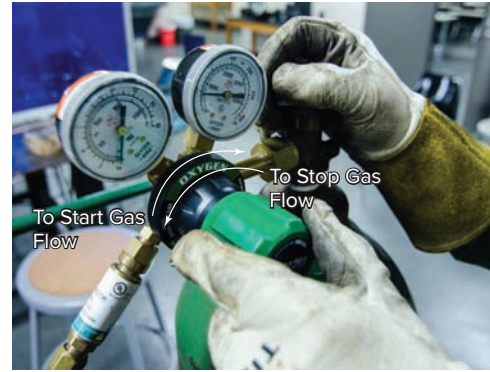
Fig. 7-24 Regulator-adjusting screw is turned to the right to cause the flow of gas through the regulator and hose to the torch. Location: Northeast Wisconsin Technical College © McGraw-Hill Education/Mark A. Dierker, photographer
