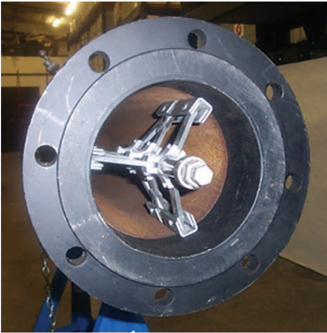
Fig. 16-21 A flange is being set up with a length of pipe for a butt joint. Note the internal clamp. © Mathey Dearman
