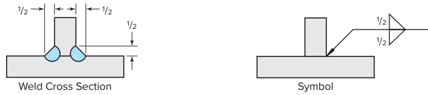
Size of Equal Double-Fillet Welds
