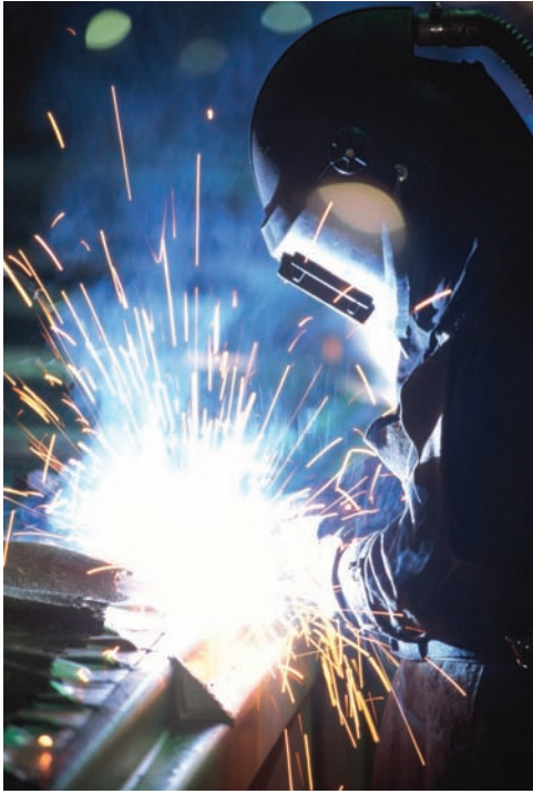
Fig. 2-22 Welding frames of railway cars. Note the safety gear and fresh air welding helmet. © Bruce Forster/Stone/Getty Images
