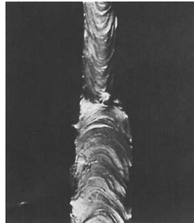
Fig. 24-41 Typical face appearance of a filler pass and a root pass in the 5G position downhill. © Plumbers and Pipefitters Union, Alton, IL
