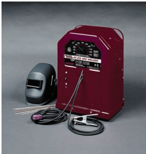
Fig. 11-17 A simple SMAW welding machine with mechanical control of the welding output. Note the switch type stepped current control. © Lincoln Electric
