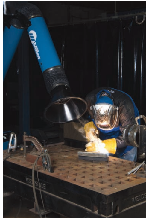
Fig. 11-43 A well-protected student welder. Note the platen table, clamps, and the position of the fume extractor for optimum protection. © Miller Electric Mfg. Co.
