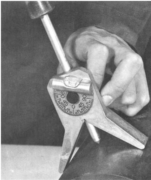
Fig. 16-98 Center head equipped with a dial-set level and center punch for locating the center line of pipe.
