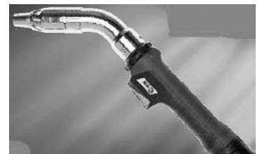
Fig. 21-50 To help reduce fumes some guns are equipped with extractor devices directly above the gas delivering nozzle system. This gun is so equipped, is water cooled, and is rated at 300 amperes at 100 percent duty cycle with carbon dioxide shielding. © Lincoln Electric
