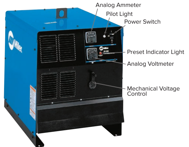
Fig. 21-24 A 300-ampere, d.c. constant voltage transformer-rectifier with mechanical brush control for voltage and tapped-inductance control. © Miller Electric Mfg. Co.
