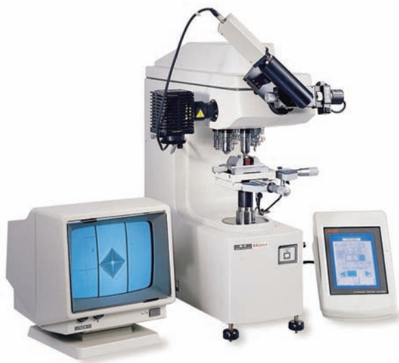
Fig. 28-57 A bench model microhardness testing system. Designed to test both Vickers and Knoop hardness scales. © Mitutoyo
