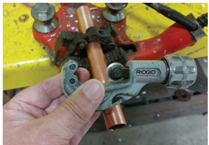
Fig. 10-6 Bench chain vise holding copper tubing to be square cut with a pipe cutter. Location: UA Local 400 © Edward R. Bohnart, Photographer
