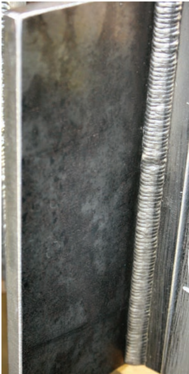
Fig. 22-22 A 3F vertical-up fillet weld using GMAW short circuit transfer. SG-AC-25 with 0.035 wire root pass was stringer. Note the uniform ripple pattern, uniform width, and minimal spatter on this as-welded \frac{3}{8} -inch weld. © Edward R. Bohnart
