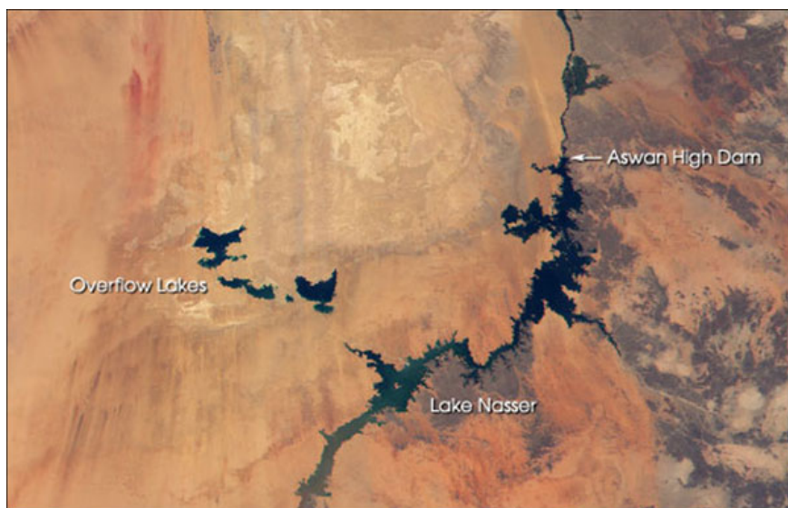
Figure 17: Satellite image of the Nile River around Lake Nasser and Aswan High Dam, 10 Oct. 2000. The exceptional rainfalls in the Nile River Basin after c.1994 slowly filled Lake Nasser to capacity, for the first time in its 35-year history. The excess waters were diverted into the Toshka Depression, out in the open Sahara Desert, where four giant overflow lakes were created. (From the MODIS imaging spectroradiometer, NASA.) (Web ref.5)
