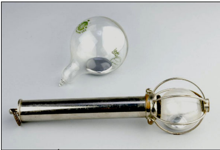
Figure 19: Early Scale-Buoy Devices, as used for boiler de-scaling and several of the Piccardi experiments (Piccardi 1962; Faigl 1990)
