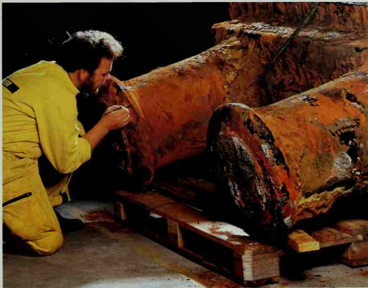
▲ Dr. Stéphane Penneç of LP3 Conservation in France studies the amount of corrosion on the Titanic 's bits. Left: Another set of bits remains unrecovered in the murky waters of the ocean bottom.
