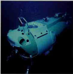
▲ The three-man submersible can reach a maximum depth of 20,000 feet on dives up to twelve hours long.
