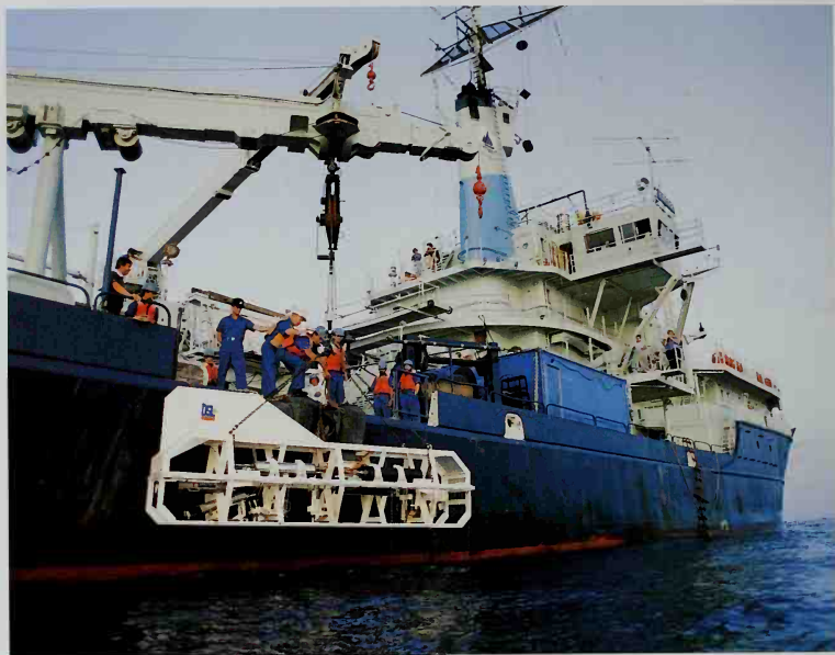
▲ Argo is launched from the Knorr on one of her numerous dives to explore and photograph the wreck site.
