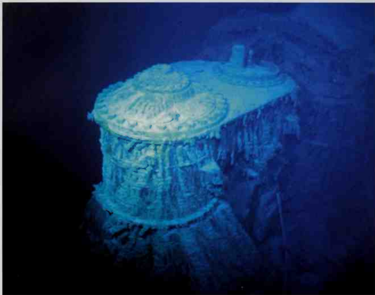
▲ A rustle-encrusted cylinder head, a part of one of the Titanic's giant, four-story reciprocating engines, appears out of the darkness. Left: A silver plate recovered from the Titanic's debris field.
