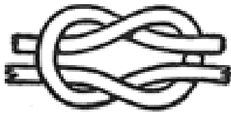
REEF or SQUARE KNOT for tying bandages and ropes.
