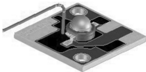
Figure 14.5 Location of thermocouple to measure LED temperature. (Source: Thermal Design Using Luxeon® Power Light Sources, Lumileds AB05, 2006.)
