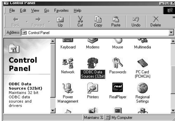
Figure 17-8: ODBC Data Sources (32 bit) contains the information about the MySQL ODBC connection.
