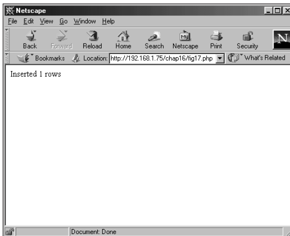
Figure 16-17: Using mysql_affected_rows to see how many rows were affected by the operation
