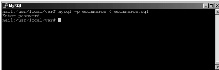
Figure 13-44: Importing an actual file produced with mysqldump into the CLI with the use of the redirect character
