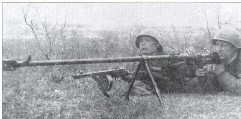
The Soviet 14.5mm Degtyarov PTRD-41 AT rifle (see also Plate F), with a length of 6½ft, was actually reasonably light for its size at 17.44kg (38lb). The barrel could be separated from the action at the point where the assistant gunner's hand rests in this photo; on the march the No.2 carried the barrel and the No.1 the action.
