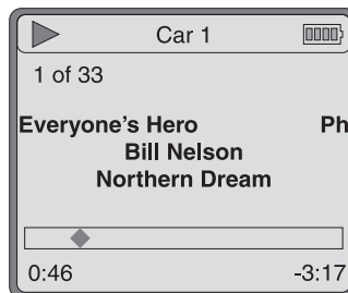
FIGURE 1-4 From the Now Playing screen, you can change the place in the song by pressing the Select button, and then scrolling counterclockwise (to move backward) or clockwise (to move forward).
