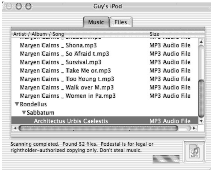
FIGURE 14-5 Podestal can quickly copy song files from your iPod, but it doesn't rename them.
