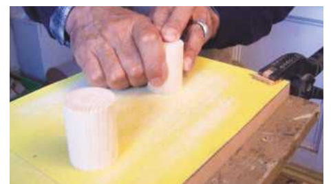
STEP 29. Squaring the ends of the blocks on a flat sanding board
