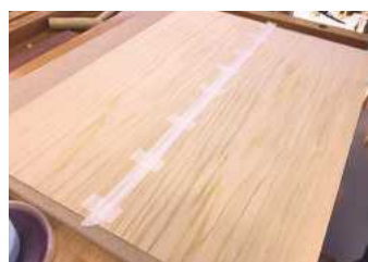
Cellulose craft paper veneer tape holding crown cut ash
