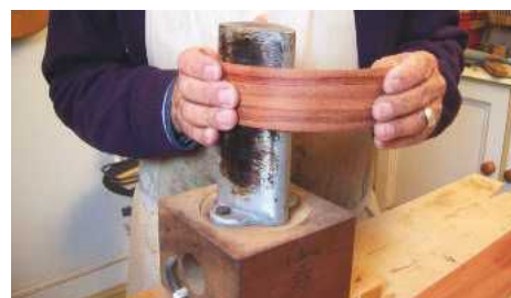
STEP 35. Bending the ribs on the hot iron
