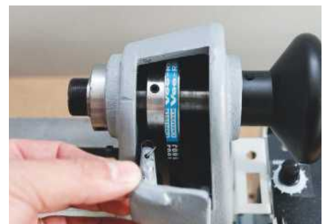
The lathe is driven by a single belt, which is accessed via a hinged flap
