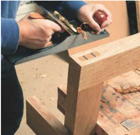
PIC 13. This through-tenon has been made very slightly longer than the depth of the mortise so it can be planed off flush on the far side. Before planing, little wedges of contrasting wood were hammered into slots in the tenon to lock it in place
