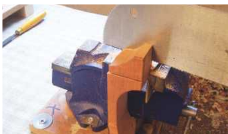
STEP 10. Reducing the width of the 'slipper'
