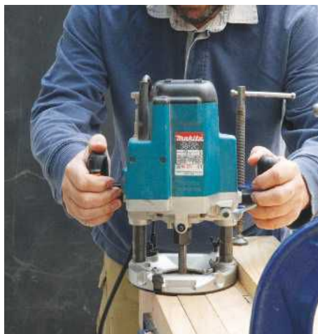
PIC 16. I am using the router to chop a mortise in a piece of wood clamped in the bench vice. To steer the router accurately down the centre of the wood I have clamped a guide rail alongside the vice (right-hand side)
