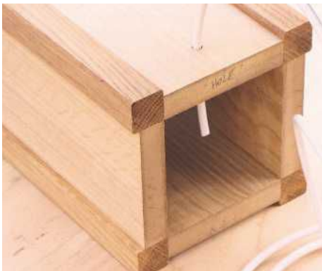
STEP 15. Drill a 6mm hole at the lower end of one side to enable three-core flex to be pushed through easily
