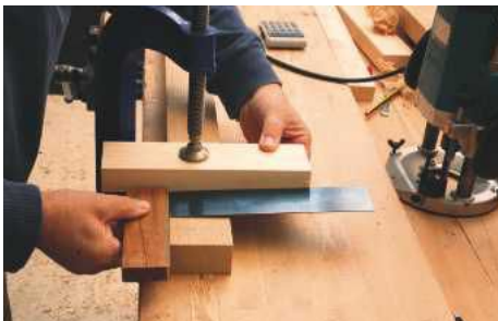
PIC 18. The guide rail must be accurately clamped at right-angles otherwise the shoulders of the tenon will be squint
