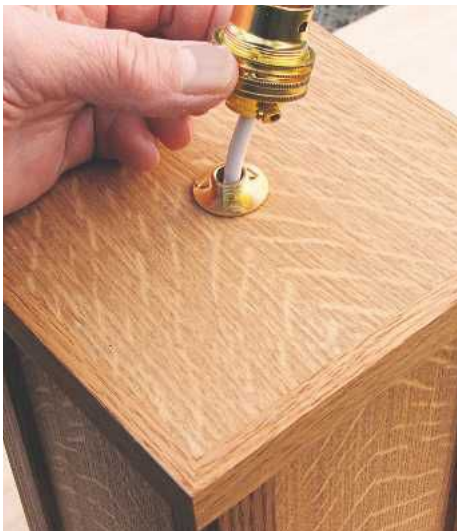
STEP 17. Strip the ends of the flex and screw to the bulb holder, making sure that the earth wire is attached
