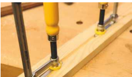
Slid in as a pair they can be used as a straightedge clamp guide for routing or sawing
