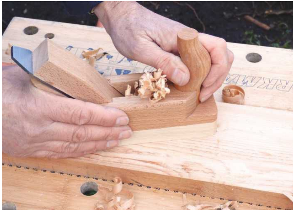
Planing up some sawn softwood and ash I found the tool delightful to use, making a pleasing hiss as it sliced across the surface
