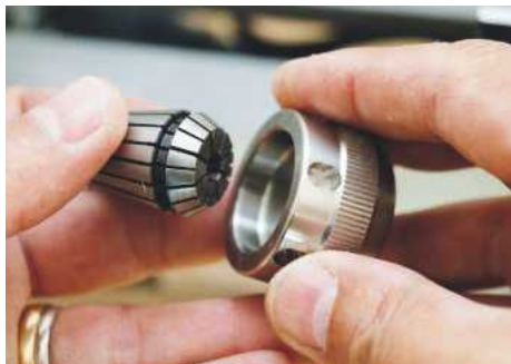
The lathe uses high quality collets to hold the various drive centres
