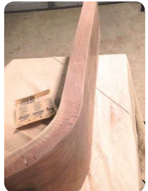
STEP 9. ... before moving on to hand sanding until all the tool marks had been removed
