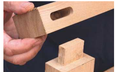
PIC 20. The problem with this router-cut joint is that the tenon has square ends while the mortise has rounded ends
