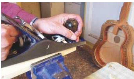
STEP 27. Preparing the pine billet for the rib- and end-blocks ready for turning
