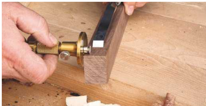
PIC 3. I'm using the chisel as a size template to adjust a marking gauge for marking out the tenon; this will ensure the tenon is the same width as the chisel and hence the same width as the mortise socket chopped by the chisel
