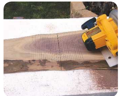
STEP 6. Starting the kerf cuts in the middle
