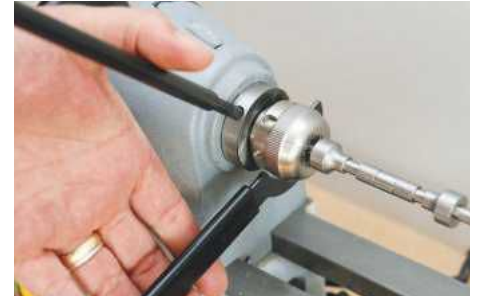
A tommy bar and pin spanner are used to tighten the collets to the drives
