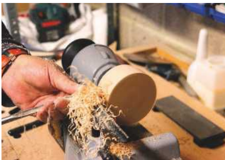
Small bowl-type jobs can be carried out using the screw chuck and faceplate
