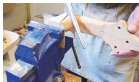
STEP 14. Final shaping of the heel is completed using a razor file
