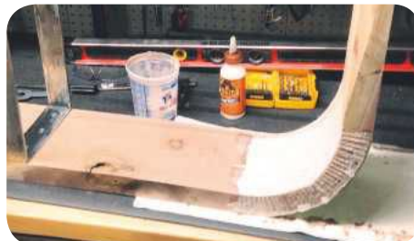
STEP 7. Gorilla Glue was mixed with the sawdust to form a flowable paste that I eased into the kerfs
