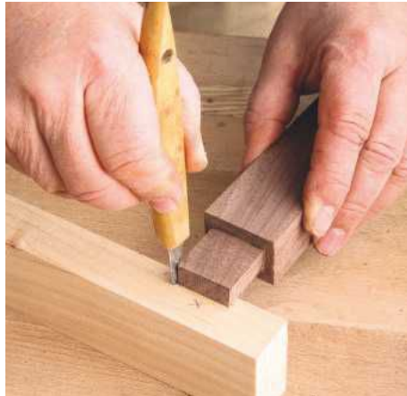
PIC 7. After the tenon has been sawn out I use it as a template to mark the length of the mortise socket
