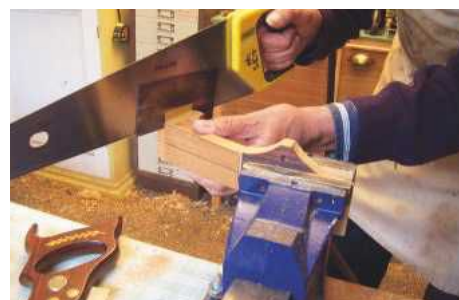
STEP 9. Cutting the 2mm rib slots
