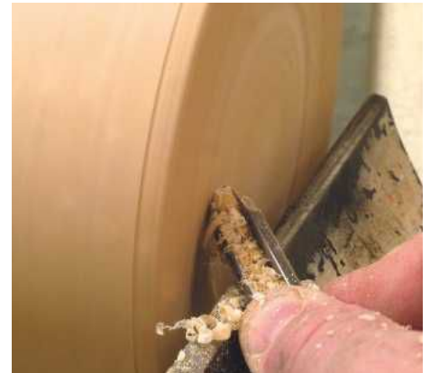
STEP 3. Just to show you shouldn't be a 'one trick pony', the pull cut is best done across the bottom of the blank. Try to match the feed speed of the tool to the speed of the wood in order to achieve the best cut possible
