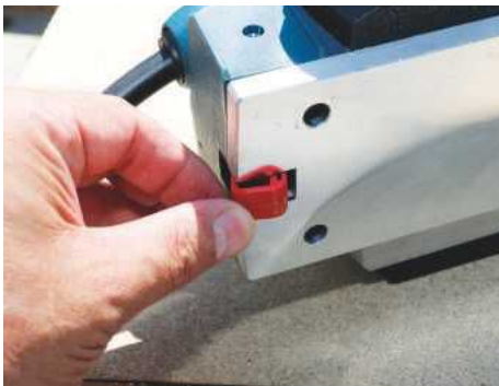
The parking shoe is spring-loaded so always sticks below the sole until used
