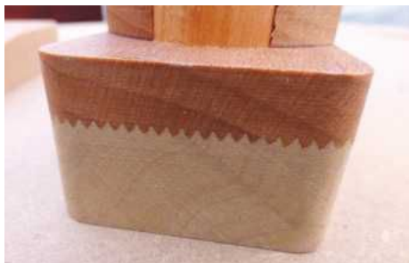
Mating surfaces are carefully machined to create a fine, toothed joint along their length before laminating the body and sole together
