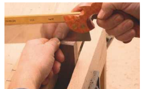
PIC 5. With the wood clamped firmly upright in a vice the sides or 'cheeks' of the tenon can be sawn by carefully following the waste side of the gauge line
