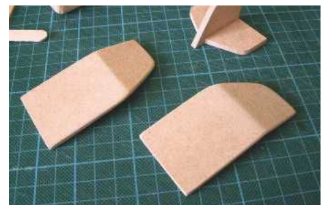
STEP 10. The sanded wings help to hide any evidence of gluing
