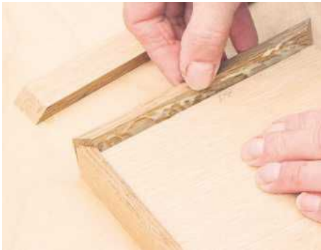
STEP 13. Trim the lipping to length with a block plane and glue to the top and bottom. Place flush when dry
