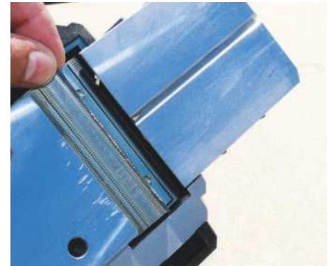
The laminated block uses a single blade; note the chamfer option on the front sole
