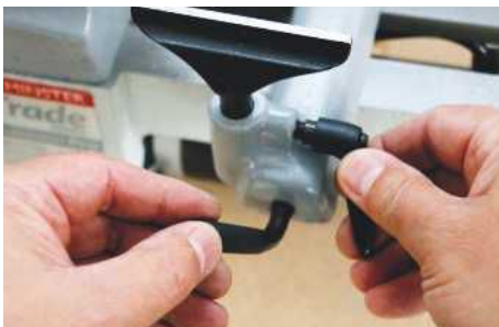
There are two toolrests supplied, both of which lock firmly into the banjo
