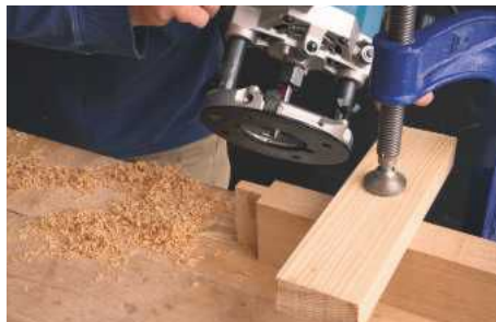
PIC 19. A simple tenon can have two shoulders, or it can be turned on edge as here to allow the router to cut four shoulders
