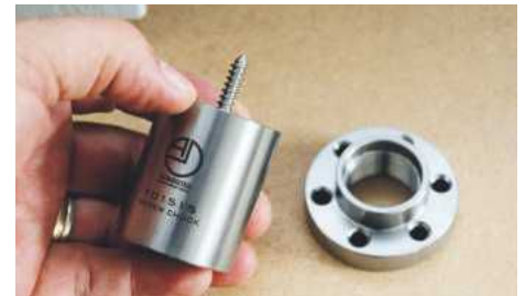
There is a small faceplate and a screw chuck that fit to the threaded spindle
