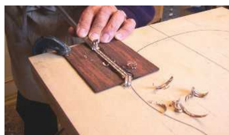
STEP 17. Trimming the head facing centre strip using a paring chisel
