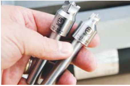
A range of drive centres are also available but require different collets to use them
