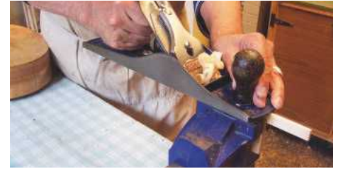
STEP 46. The harmonic bar under preparation
