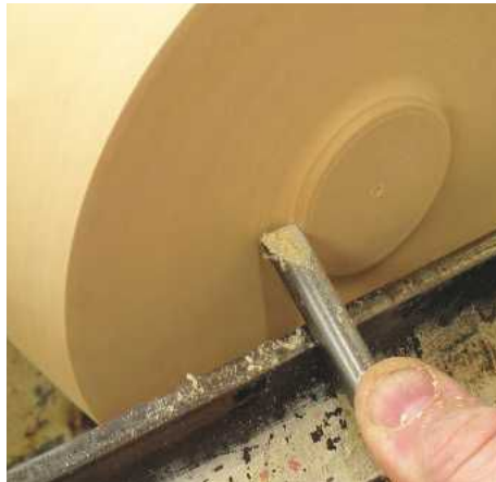
STEP 5. Here I am using the 10mm round skew chisel to square up the spigot after I have removed the excess wood with the gouge. It's easy enough to angle the tool slightly to create a small dovetail shape to match the chuck jaws
