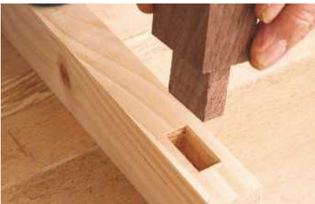
PIC 10. The series of chippings can be scooped out with the chisel held bevel down. The process is repeated until the socket is deep enough to receive the tenon
