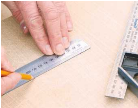
STEP 1. With veneered boards, find the centre of each bookmatched pattern in order to maintain symmetry
