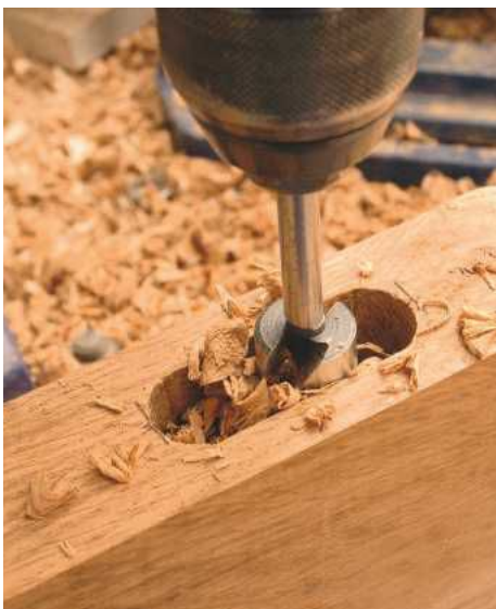
PIC 25. A pillar drill is an alternative to the router for sinking mortise sockets. Forstner bits are ideal for this because they can produce a series of overlapping round holes with clean edges
