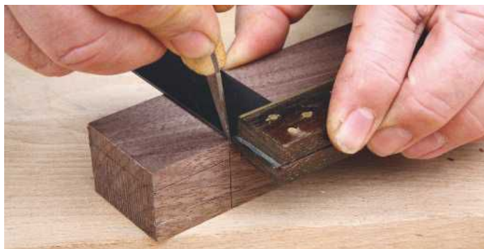
PIC 4. To mark the shoulder lines around the base of the tenon, I use a try-square and a fine-bladed knife
