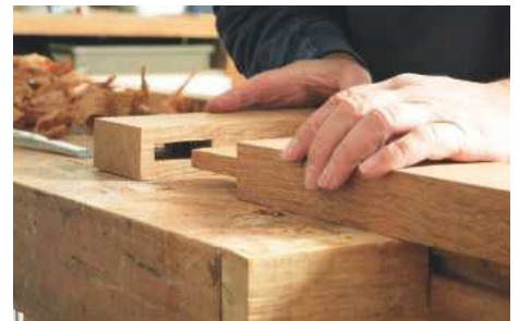
PIC 12. You can see daylight out the other side of this mortise, so it is known as a through-mortise. I chop these out from both sides of the wood, so they meet in the middle like a tunnel
