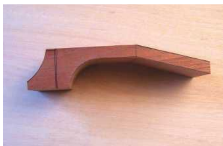
STEP 8. The layout of the rib slots and soundboard ledge
