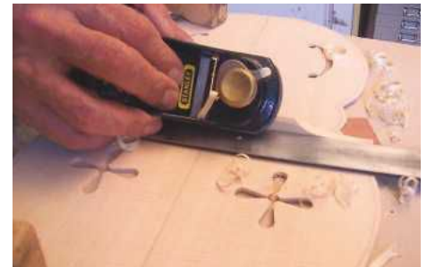
STEP 50. Gabling the ends of the harmonic bar
