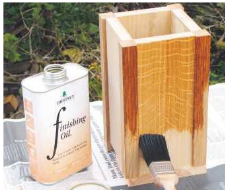
STEP 16. After sanding the box with fine abrasive, brush on two coats of finishing oil before attaching the top and base
