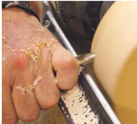
STEP 2. Hole the blank on a screw chuck or faceplate and true up the timber using a bowl gouge. I like to use a push cut for this as I find it leaves a better finish than a pull cut
