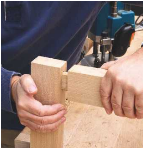
PIC 22. The mortise & tenon joint should be firmly fitted by hand without forcing. Adjustments can be made if it is too tight but this takes time
