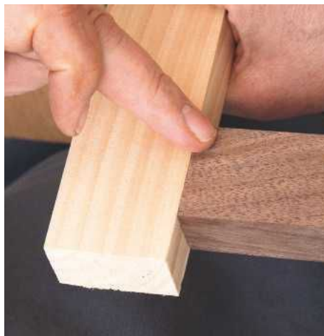
PIC 11. When a mortise & tenon are well fitted they slide together with firm hand pressure but no forcing
