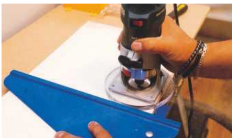
Slots can be routed against a straightedge and can be short...
