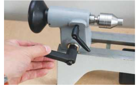
The tailstock locks off with a good quality large lever at the rear side
