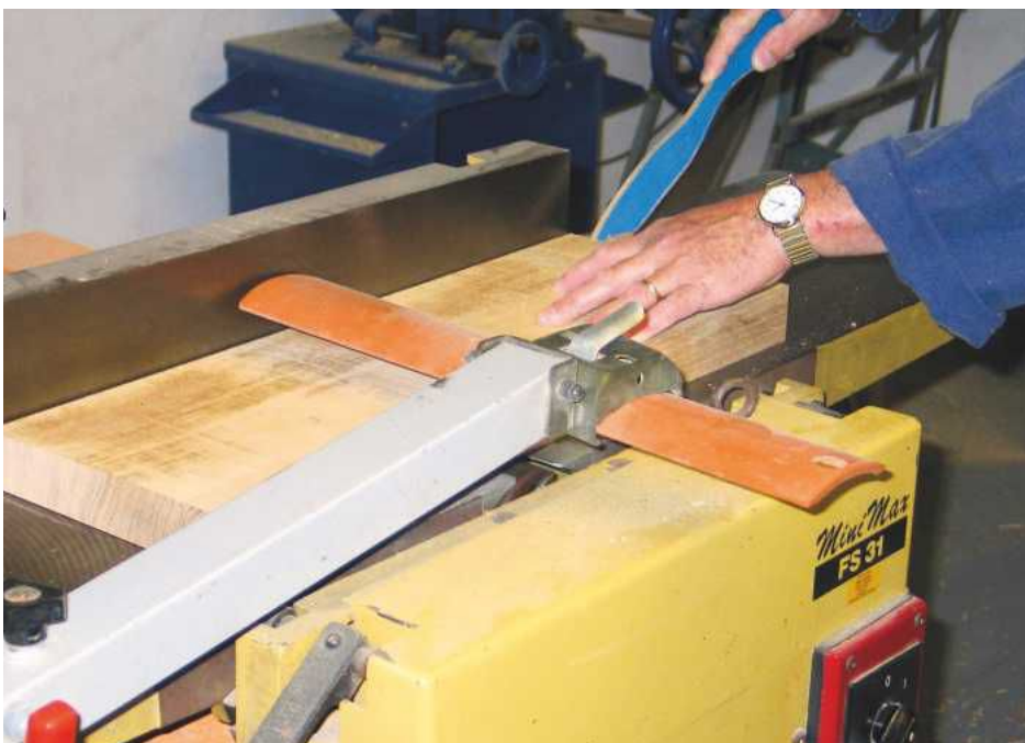
Surfacing the timber
