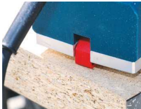
It protects a surface by lifting the cutter away when placed down while still running
