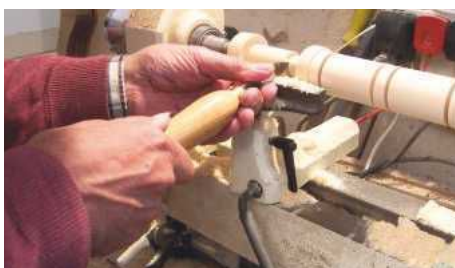
STEP 28. Turning the rib- and end-blocks on the lathe
