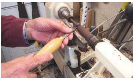
STEP 24. Turning the rosewood pegs on the lathe
