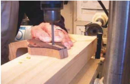
STEP 21. Drilling out the peg holes
