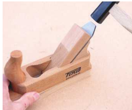
Cutting depth is simple enough to set by gently tapping the end of the blade with a small hammer
