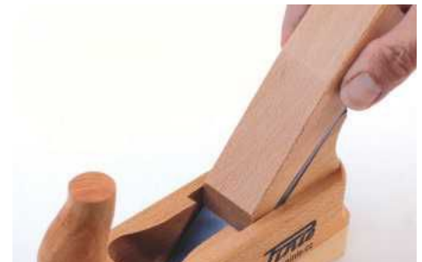
The blade is held in place with a beech wedge, which acts as a chipbreaker
