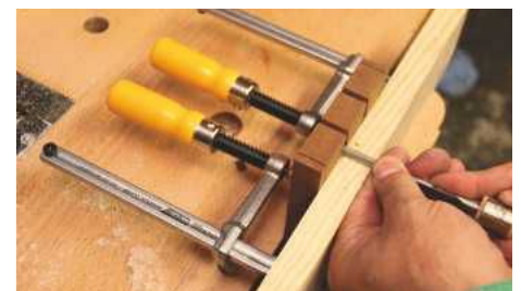
The clamps pull the work to the guide for accurate paring of the dovetail sockets
