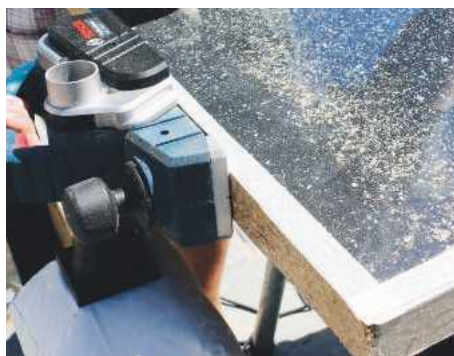
Laminated worktops are easily planed and without snipe when running off the edge
