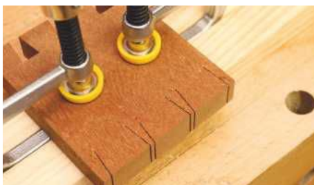
Slid up close the clamps are great for holding small components like this dovetail
