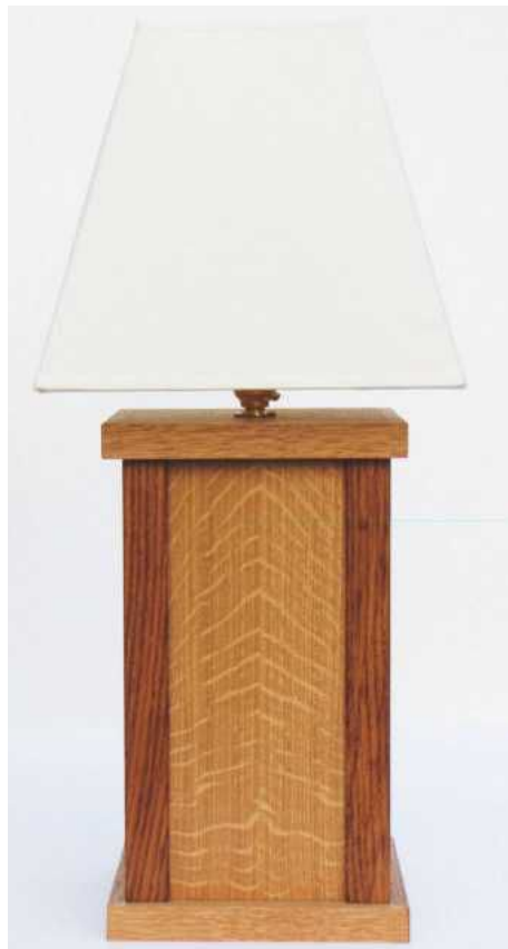
STEP 16. After sanding the box with fine abrasive, brush on two coats of finishing oil before attaching the top and base
