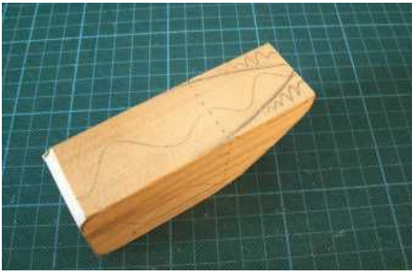
STEP 4. Next, mark off the parts of the wood that need to be sanded off
