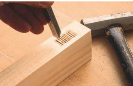
PIC 9. A series of shallow chops along the length of the mortise avoids denting the wood
