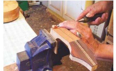
STEP 23. Chiselling the soundboard ledge
