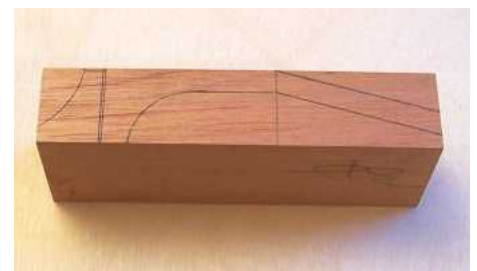
STEP 4. The head and neck outline transferred onto the cedar billet
