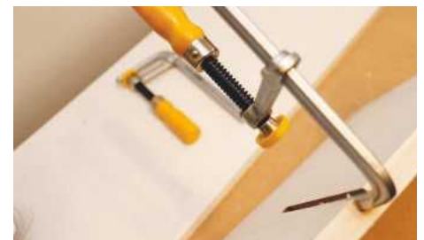
The clamp slides in just below the surface. As a single clamp it's useful as a basic hold down
