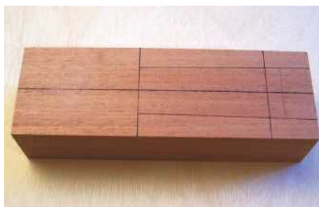
STEP 5. The outline of the fingerboard transferred onto the cedar
