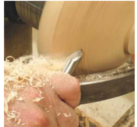
STEP 6. The 13mm bowl gouge is my desired tool to use when turning bowls of this size. An aggressive pull cut will allow me to achieve the shape I want quickly. The round toolrest aids support of the tool throughout the cut
