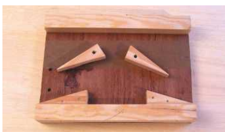
STEP 15. The headstock facing jig
