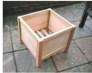
➤ The narrow cut channels help to give the piece a 'ship-lap' look
