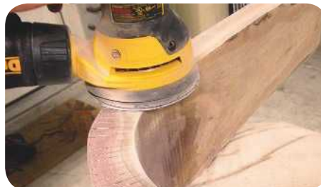
STEP 8. Using a random orbital sander, I sanded the piece down to 320 grit...
