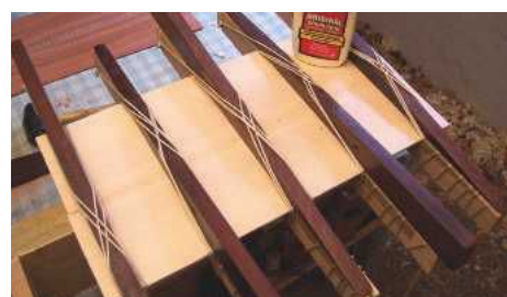
STEP 41. The two halves of the soundboard in the wedge and lace jig
