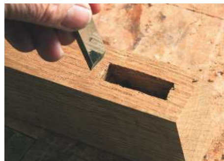
PIC 26. Round-ended sockets cut with a router or drill can be chopped square by hand with a chisel
