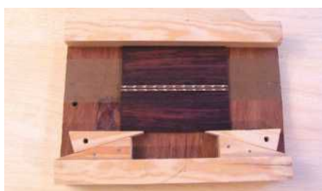
STEP 16. The headstock facing held firmly in the jig while the glue sets
