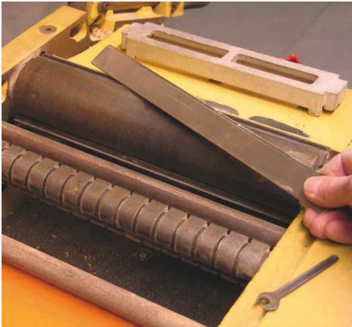
Most of these planers will have two or three cutters set in their blocks
