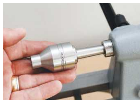
The tailstock has a standard Morse taper fit for live centres and such like
