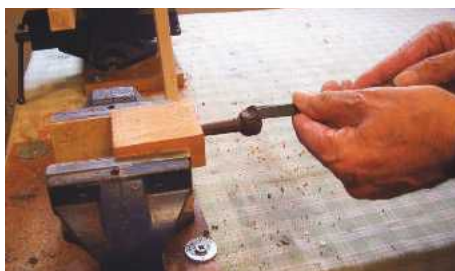
STEP 25. Chiselling the flats on the peg buttons
