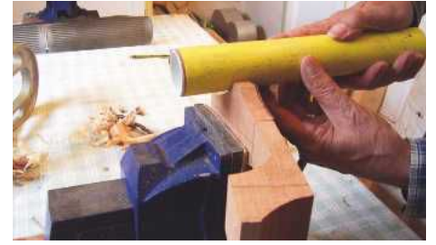
STEP 20. Shaping the headstock with a round sanding stick
