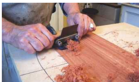
STEP 34. The ribs are reduced to 2mm thickness using a scraper plane
