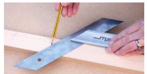
Unlike some mitre squares the blade is offset, enabling you to mark a line across material up to 95mm wide
