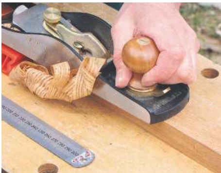
STEP 4. Plane contrasting timber square for the corners. Make these about 12mm longer than panel height
