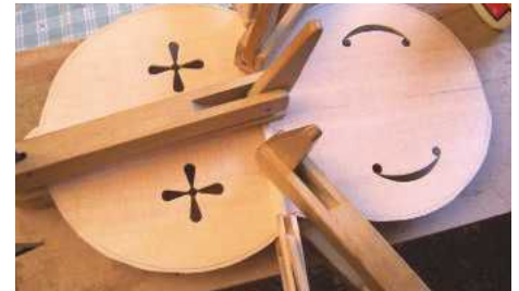
STEP 48. The bar is clamped into position using Titebond glue
