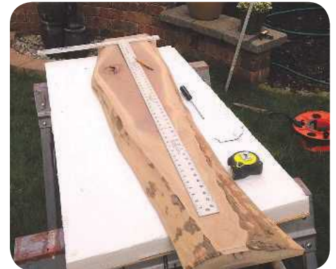
STEP 5. Squaring the end of the board and laying out the kerfs
