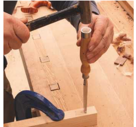
PIC 8. Chopping out a mortise socket the traditional way with the chisel held vertical and tapped with a mallet
