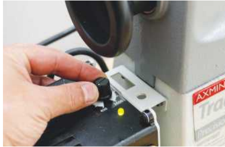
The variable-speed runs from 400-3,600rpm and works very smoothly throughout
