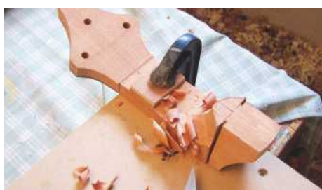
STEP 12. Using a Japanese marking knife to shape the heel
