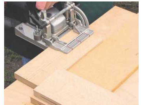
STEP 6. Cut slots for biscuits, making sure that the panels are flush with the corner pieces on the rear faces
