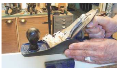
STEP 39. The soundboard edges that will meet are planed true
