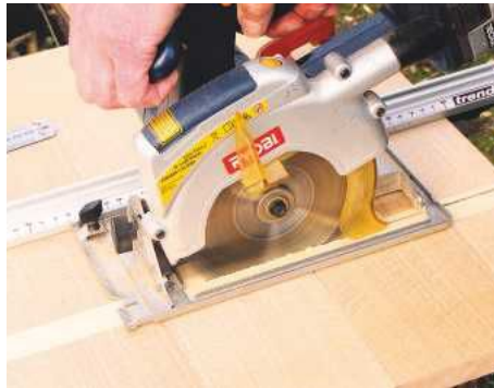
STEP 2. Saw the panels slightly oversize. Use masking tape along the line of cut to prevent the veneer splintering on the face
