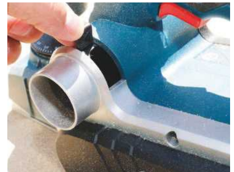
This lever directs the dust and shavings to either side of the tool as required
