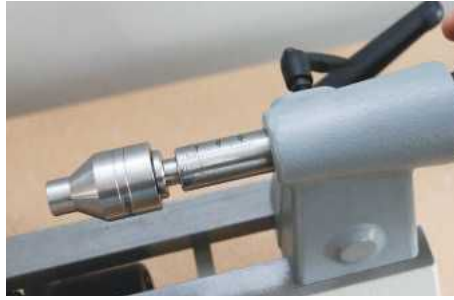
The tailstock features a graduated scale; useful for blind drilling jobs
