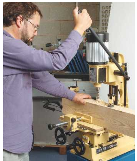
PIC 27. The mortiser looks similar to a pillar drill but is specially designed to chop a series of square holes. It has a sharp-edged square cutter around a specially designed auger bit
