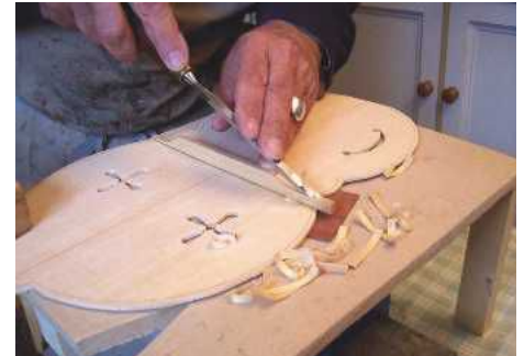
STEP 49. Scalloping the ends of the harmonic bar
