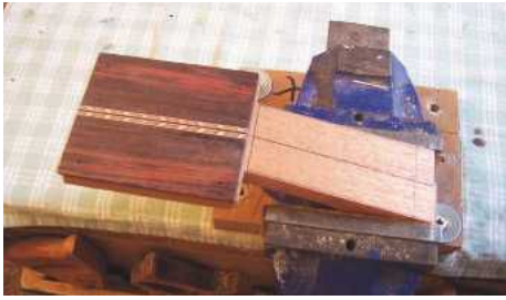
STEP 18. Pin holes are placed on the facing to prevent movement
