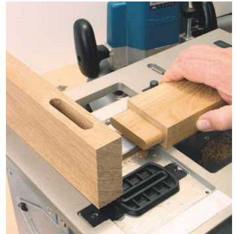
PIC 24. This jig is designed to produce round-ended tenons to match the round-ended mortises
