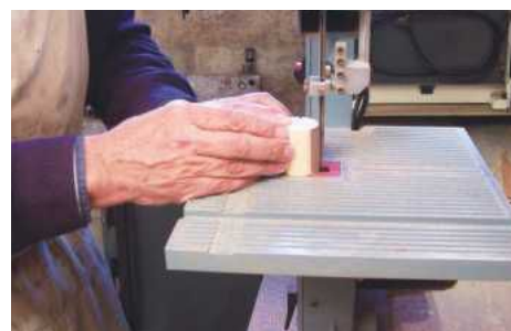
STEP 32. Cutting the first rib slots on the bandsaw
