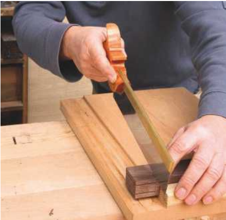
PIC 6. The wood must be held horizontally while sawing the shoulders of the tenon. Here I am using a bench-hook and securing the wood against it with my left hand while carefully following the waste side of the knife line
