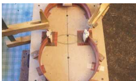
STEP 37. Cams help to keep the shape
