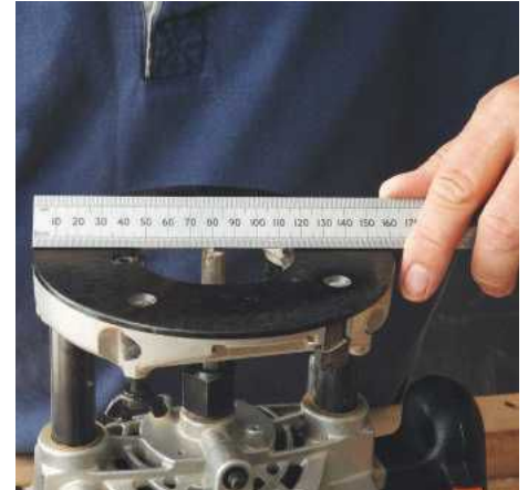
PIC 15. The router must be positioned accurately so we need to measure the distance between the edge of the cutter and the edge of the router sole plate
