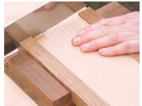
STEP 9. Saw off the excess at the top and bottom of the corners. Trim the end-grain flush with a plane and shooting board
