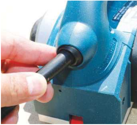
A neat ball socket on the cable helps protect it as well as easing movement in use
