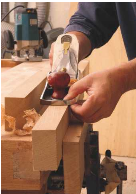
PIC 2. If you want your joints to be straight without gaps around them, then the wood must first be planed to have accurately square edges
