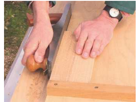
STEP 3. Trim the veneered panels square and to exact size on a shooting board
