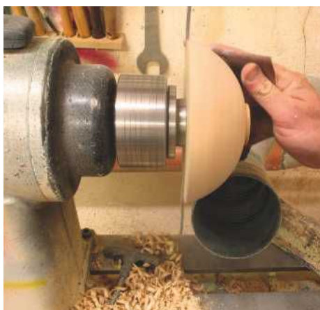
STEP 7. After going around the shape with the small gouge to increase the quality of the finish, it's time for sanding. I am only sanding with 100 grit abrasive at this stage
