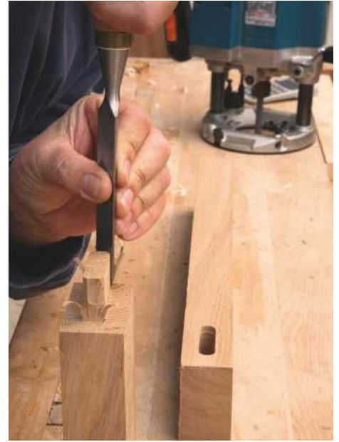
PIC 21. One simple solution is to round off the ends of the tenon with a chisel
