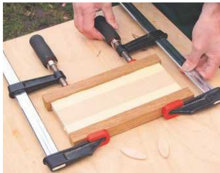
STEP 8. Glue the corner pieces and panels together and clamp for at least 30 minutes when using PVA
