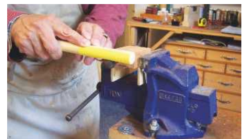
STEP 26. Applying a curve to the flats on the peg button
