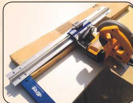
STEP 3. Using the Kreg Rip-Cut tool allowed me to guide, measure and keep my cuts consistent
