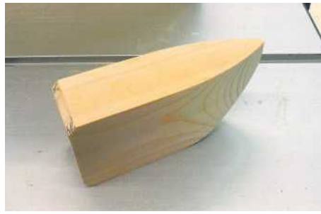
STEP 5. Take your block to the disc sander or sand by hand until all the sawn edges are smooth
