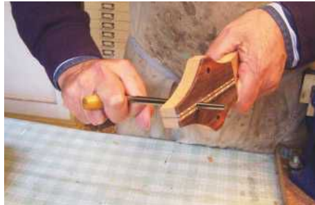
STEP 22. Reaming the peg holes
