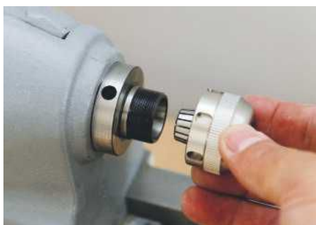
You screw the chuck directly to the headstock; there is no Morse taper at this end
