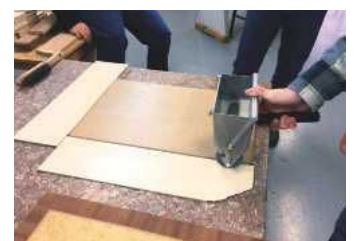
The gravity feed roller applying an even layer of UF adhesive
