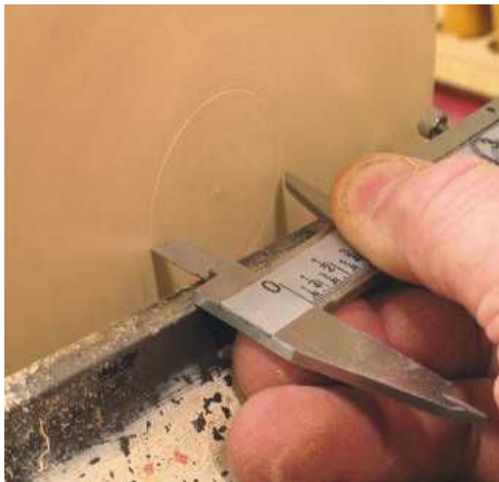
STEP 4. Transfer the diameter of your chuck jaws to the bottom. As with most of my bowls, I like to grip onto a spigot rather than expand into a recess
