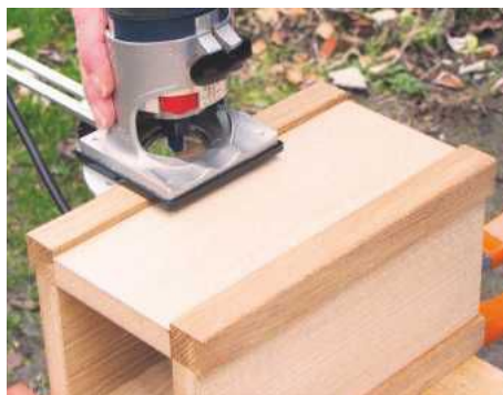
STEP 11. Create a small chamfer along the edges of the corners with a router and 'V' cutter or block plane
