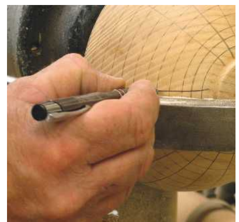
STEP 9. I have marked the bowl out as I would have done for a barley twist. I decided that I would have the bricks evenly spaced rather than just placed randomly
