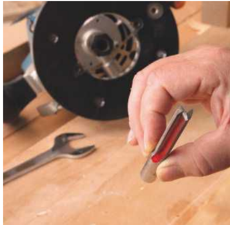
PIC 14. The router, fitted with a sturdy straight-sided bit matching the width of the joint, can be used for chopping mortises
