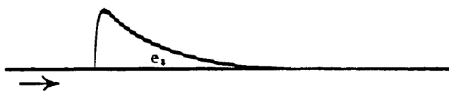
Figure 3: Reproduction of Oscilloscope of Propagation of Impulse Over Transmission Line; no Reflection. Voltage.
