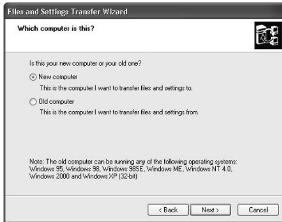
Figure 1-9: The Files and Settings Transfer Wizard can send most (but not all) of your important information from an old PC to a new one.
