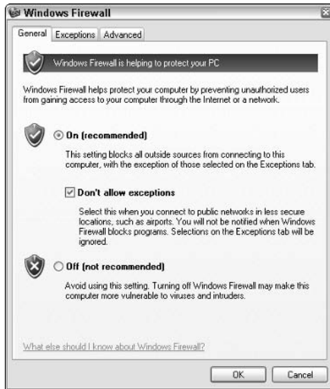
Figure 4-1: The Don't Allow Exceptions check box allows you to lock down your computer with a couple of simple clicks.
