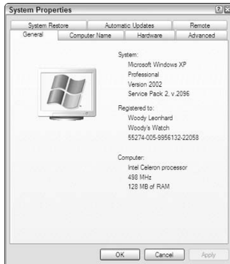
Figure 1-6: The System Properties dialog box displays the amount of RAM in your system.
