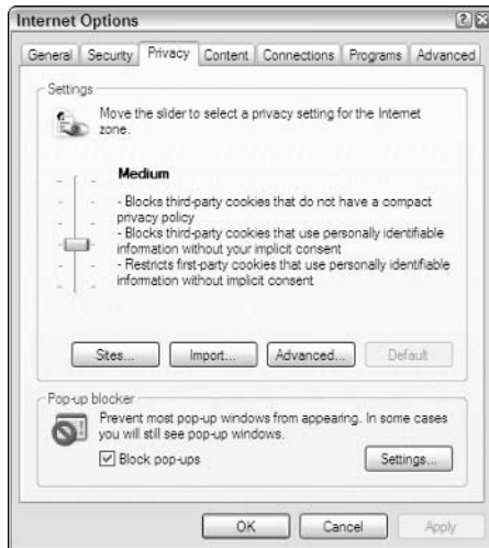
Figure 4-4: Internet Explorer's cookie handling is tied directly to the site's P3P policies.
