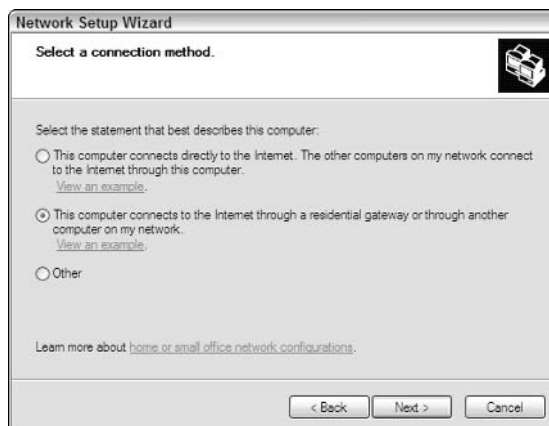
Figure 2-3: Configuring a networked computer to use a cable/ DSL/satellite modem.
