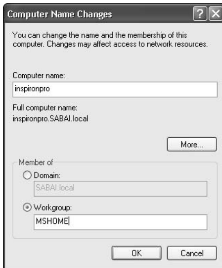
Figure 8-4: Switching your Windows XP/Pro machine from a Domain (client/server network) to a Workgroup (peer-to-peer network).
