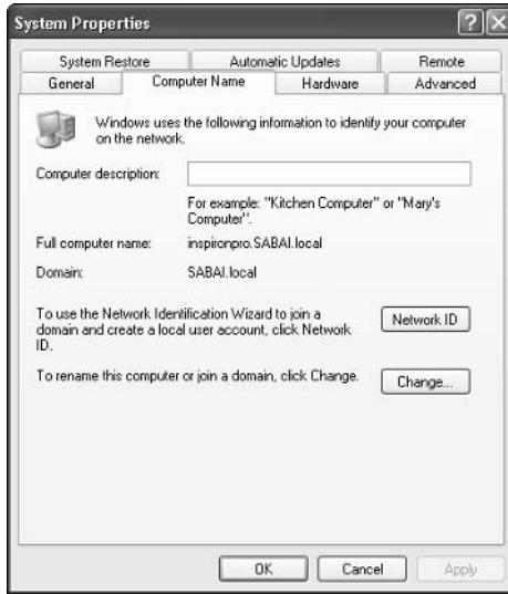
Figure 8-3: Tell Windows XP/Pro to attach the PC to a different network by going through the Computer Name tab.
