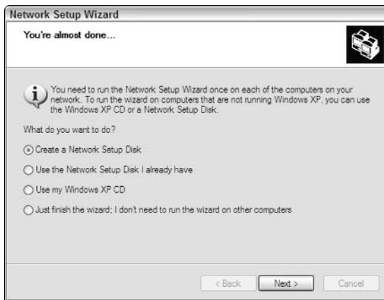
Figure 2-9: If any computer on your network is not running Windows XP, create a Network Setup diskette.
