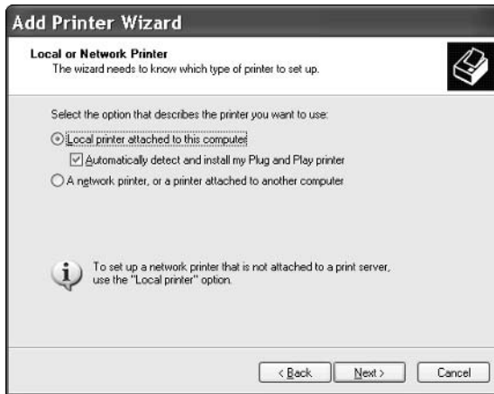
Figure 2-2: The Add Printer Wizard asks if you have a local or network printer.
