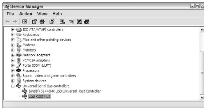
Figure 1-2: This USB controller is not USB 2.0 — it's an older USB 1.1.
