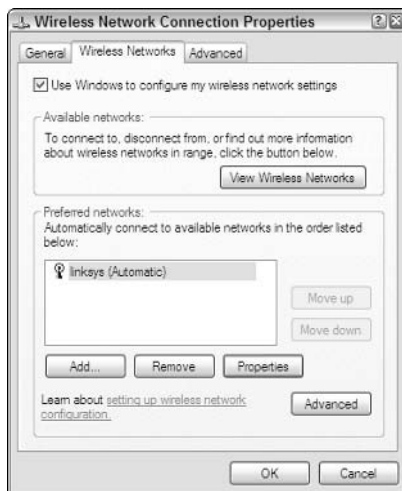
Figure 3-5: A list of the networks that Windows will auto- matically connect to.
