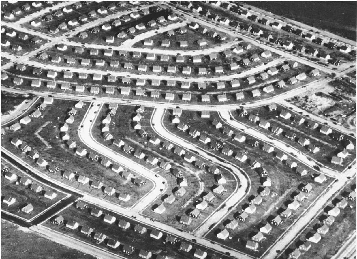
This aerial photograph of Levittown, New York, was taken in 1948, shortly after the planned community was completed on Long Island farmland near Manhattan. Real estate developer William J. Levitt created mass-produced, low-cost, tract housing to address the housing crunch after World War II. (AP/Wide World Photos)
