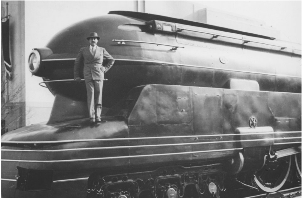
Early twentieth-century Modernism celebrated the machine, speed, and motion. Industrial designer Raymond Loewy poses next to the prototype of the streamlined S-1 locomotive, created for the Pennsylvania Railroad and on display in this photograph in Wilmington, Delaware, in 1937. (Library of Congress)
