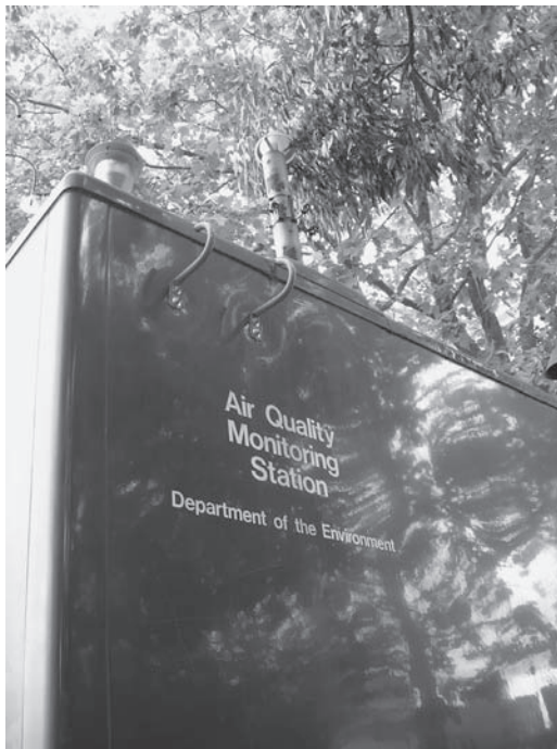
Figure 7.1 Automated air quality monitoring station, Centenary Square, Birmingham
