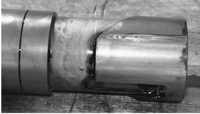
Figure 15.12 Low viscosity low sulfur fuel leads to sticky plungers (Reproduced from MAN B&W Diesel A/S, Copenhagen, Denmark, “Operation on low-sulphur fuels, two-stroke engines,” © 2009.)
