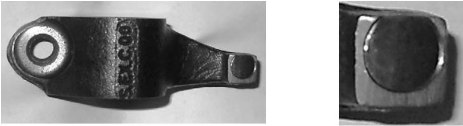
Figure 4.22 Wear of rocker lever tip. Left: Tip wear of cast iron rocker lever with chilled toe, without a valve cap. Right: Enlarged view of dimple shaped wear of the toe (Hardness of the valve tip, Rc 50; hardness of rocker toe, Rc 23)
