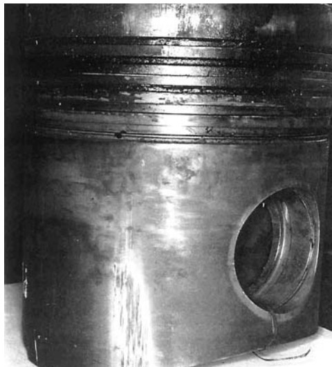
Figure 7.6 Field engine piston – hard carbon at the top land
