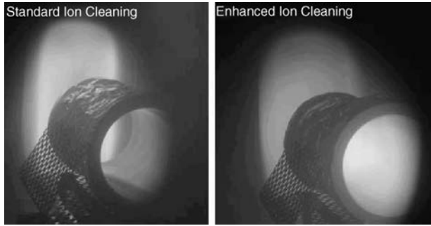
Figure 11.11 Photo shots of cylinder liners in front of Cr target during ion cleaning; the standard ion cleaning (left) did not produce plasma penetration whilst an enhanced ion cleaning (right) produced the desired penetration (Igartua et al. , 2004)
