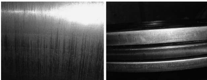
Figure 15.16 Scuffed liner and piston ring surfaces due to catalyst fines (Reproduced with permission from MAN B&W Diesel A/S, Copenhagen, Denmark, All rights reserved.)
