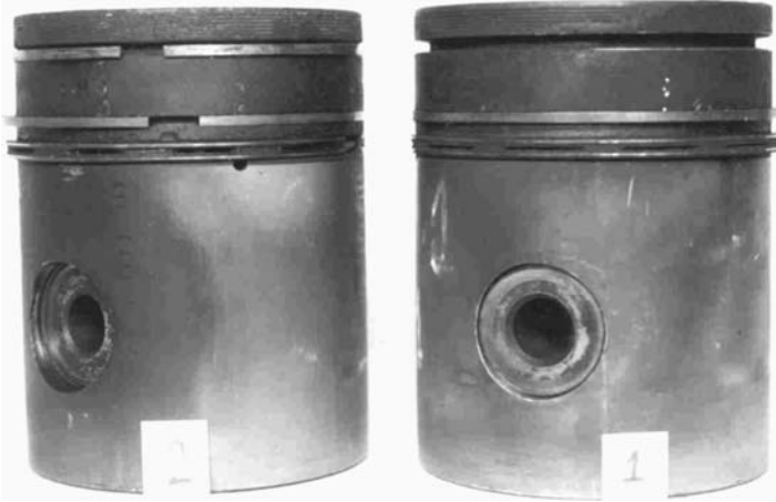
Figure 9.11 Formation of varnish on the piston skirt and land areas
