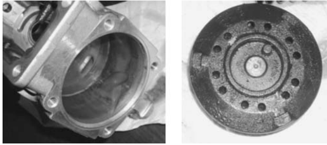
Figure 14.8 Rusting of parts in the fuel injection equipment
