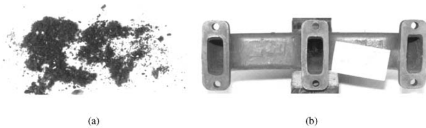
Figure 9.13 Dust in the inlet manifold due to an inefficient oil bath type air cleaner. (a) Dust particles collected; (b) dust on the surfaces in the inlet manifold
