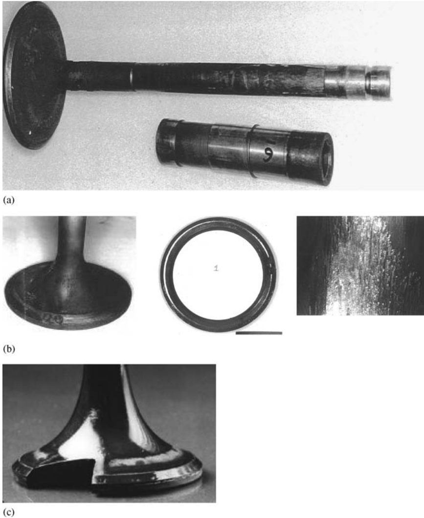
Figure 15.21 Damage due to wear by high temperature corrosion. (a) Damaged exhaust valve assembly due to eutectic deposits of sodium and vanadium; (b) exhaust valve head and valve seat damaged by low melting eutectic mixture of sodium and vanadium, valve stem shows heavy wear; (c) damage leading to breakage of exhaust valve head
