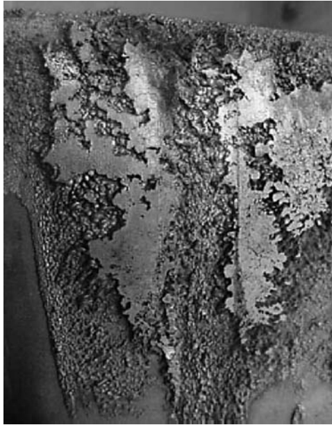
Figure 15.14 Close-up view of piston showing a deposit build up sufficient to contact the liner surface. In this condition there is a high risk of sudden severe wear (Reproduced from Welsh, M. “Considerations for using low-sulphur fuel,” Wärtsilä Corporation, 2001.)
