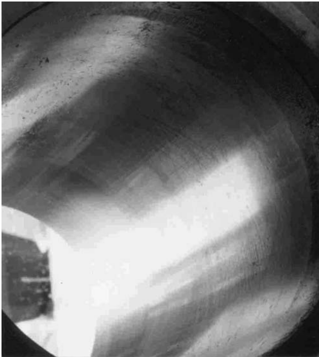
Figure 9.12 Liner wear during accelerated test using old type air cleaner – abrasive action
