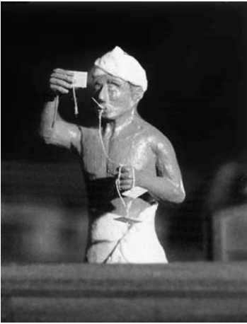
Illustrations 50 & 51 (Left) A model of a mariner using the kamāl (courtesy of The Mariners' Museum, Newport News, Virginia); (right) an Indian Ocean navigator measures with the kamāl , Capella ( ʿayyūq ) and η Ursae Majoris ( naʿsh ) (after Brice 1981: 3)
