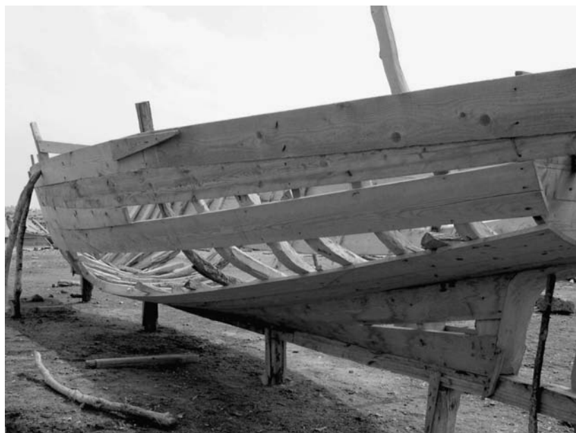
Illustration 38 The shell technique method, fitting first the planks to the sides followed by laying the frames, applied in Suakin 2004 (photo author)
