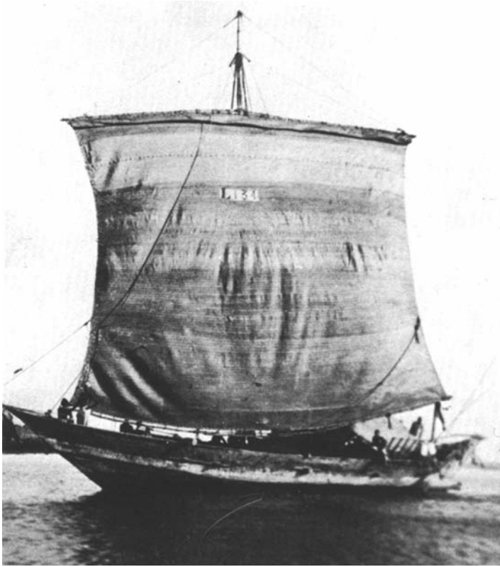
Illustration 57 A square sail made of matting on the dau la mtepe , Mombasa 1900 (after Hawkins 1977: 21)
