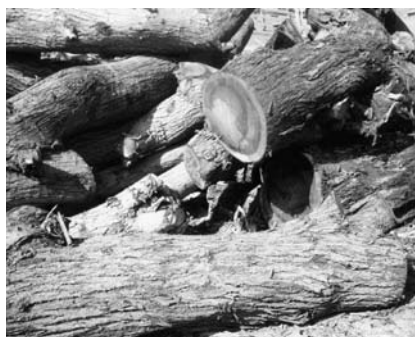
Illustrations 35 & 36 Qaraṭ timber (left) is good for framing and sidir wood (right) is for the ribs, Suakin 2004 (photos author)
