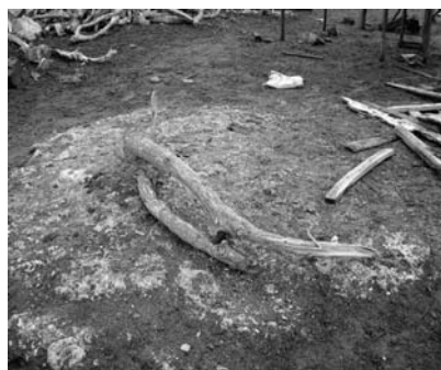
Illustrations 35 & 36 Qaraṭ timber (left) is good for framing and sidir wood (right) is for the ribs, Suakin 2004 (photos author)
