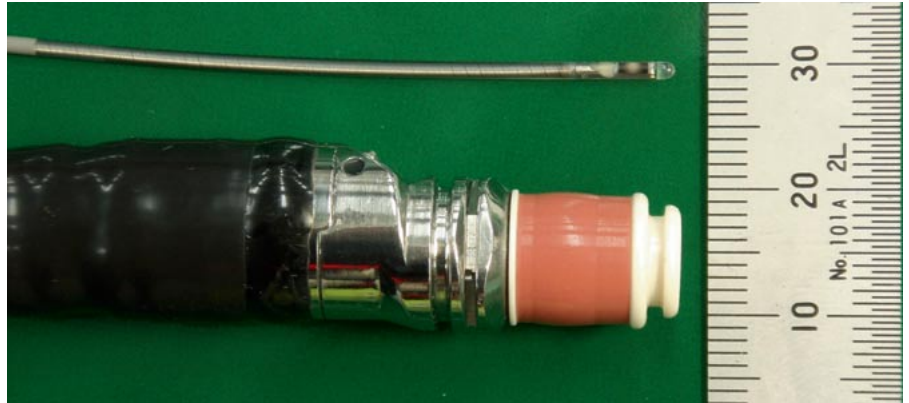
Fig. 13. Electronic radial scanning gastro-scope GF-UE160-OL5 and mechanical radial scanning miniprobe UM-S20-175.
