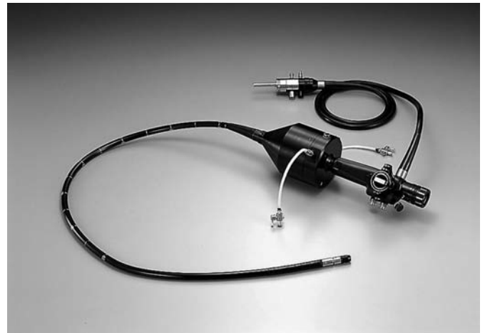
Fig. 1. The first prototype of a mechanical mirror-type ultrasound endoscope.
