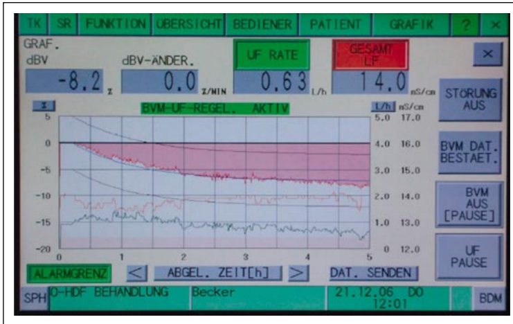
Fig. 2. Screenshot of BVM with UF and conductivity regulation with Haemomaster (Nikkiso Co. Ltd, Japan).
