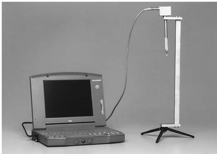
Fig. 1. QC scaler clinical unit as used today. Computer control of transducer-modified scaler permits real-time collection of scaling information on a tooth-site basis. Scaler hand-piece with curette is shown on the right.
