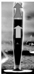
Figure 4: Electron micrograph of a GaAs micro-post cavity. The photons are emitted by an InAs quantum dot (depicted schematically by a triangle) embedded in the center of the microcavity, and resonant with the fundamental cavity mode. These photons will be channeled preferentially into that mode, and thus produce a highly directional beam (image: Izo Abram, LPN Marcoussis).
