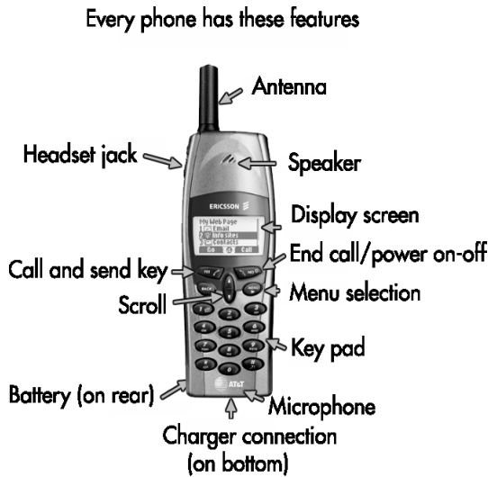
Figure 5.1 The Basic Components of All Cellular Phones Illustrated Using the Ericsson R289LX
