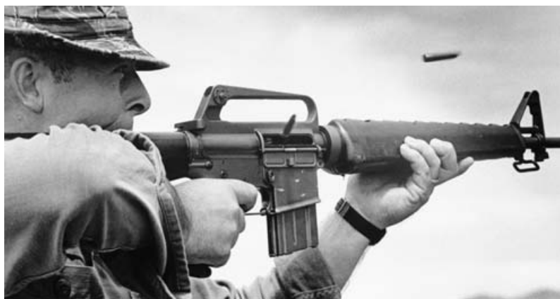
A US Navy Mobile Riverine Force sailor fires an early production XM16E1 into riverbank foliage where VC movement was spotted, Mekong Delta, 1967. Note the lack of a forward assist device. Prior to 1967 riverine assault and support craft of the MRF were armed with Mk 1 Mod 2 rifles – M1 Garands converted to 7.62mm NATO. (Bettmann/Corbis)
