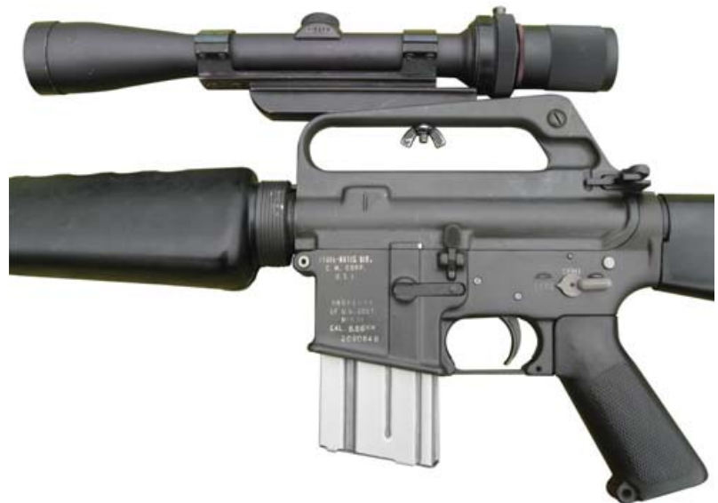
An M16A1 rifle mounting a Colt/Realist 3× telescope. Almost 400 were sent to Vietnam in March 1967 and used by specialist marksmen. It by no means turned the M16 into a sniper rifle. The carrying handle proved to be an inadequate mount for telescopes. (Trey Moore collection)
