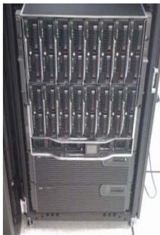
Figure 5.7. HP Proliant blade enclosure (full of blades), with two 3U UPS units below (Source: Wikipedia, http://en.wikipedia.org/wiki/Blade_server )
