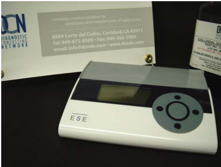
Fig. 1.5 ESEQuant portable benchtop lateral flow strip reader by ESE GmbH. Fluorescent or visual labels can be read
