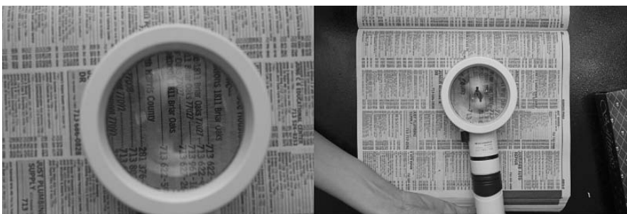
Fig. 6.3 Stand magnifier resting on a phone book to provide a virtual, enlarged image
