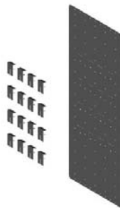
Figure 4.4 A planar 4 \times 4 antenna matrix made of quarter wave patch elements [12].
