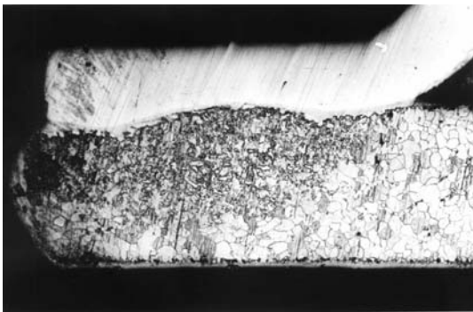
Figure 7.37 A cross section of the corner of the welded housing. The basic geometry of the cover can easily be seen (scaling \times 10 ).
