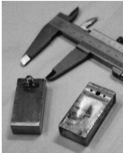
Figure 7.11 The laser welded steel prototype is completely sealed except for the small coaxial SMA-type connector. The outside appearance of the test unit is of no technical importance. The rectangular cavity resonator has six conducting walls and a coaxial feed. The wave propagates and resonates along the z -axis. The detailed 3-D CAD model is presented on the attached CD-ROM [7].
