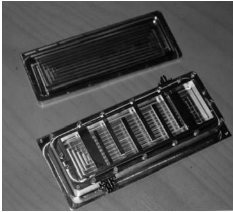
Figure 9.2 The tested filter is a fully machined construction. The track of the milling tool is visible on the bottom, but the surface roughness is better than 0.8 \mu\text{m} . The sharpness of the resonator root has the key role. Due to milling technology it is impossible to get absolutely sharp edges of the body itself [4, 5].
