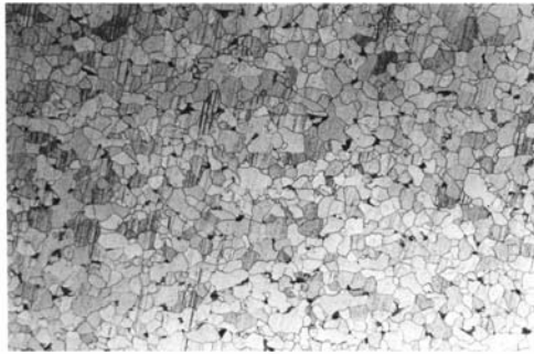
Figure 7.36 A microstructure photo (scaling \times 100 ) of the base material right under the cover. It is delightful that the changes due to welding are insignificant and the structure is mostly fine-grained perlite as desired.
