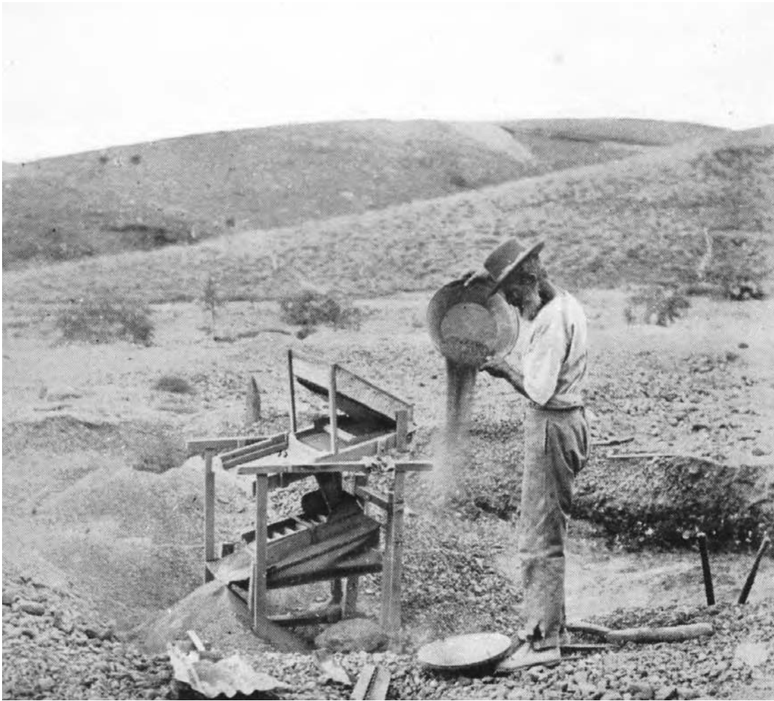
On the arid Western Australian goldfields there was often no water for washing pay dirt, so various dry-blowing systems were devised. (E. J. Brady, Australia Unlimited, Melbourne, 1918, p. 730)
