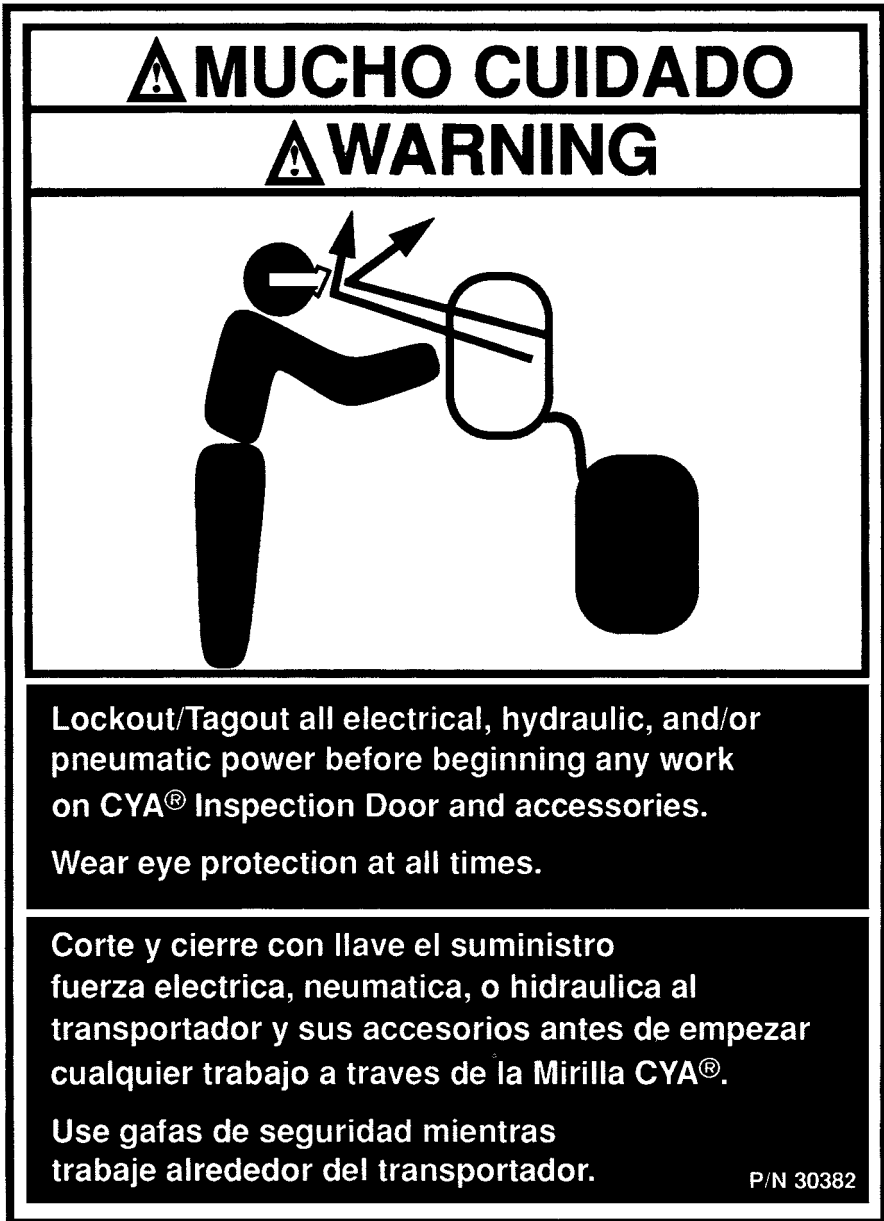
Figure 8.5 Bilingual warning label. The label uses orange for level hazard (Warning), a pictorial, and bilingual presentation of all prose text. (Courtesy of Holly A. Webster, Martin Engineering Company, Neponset, IL, 1990.)
