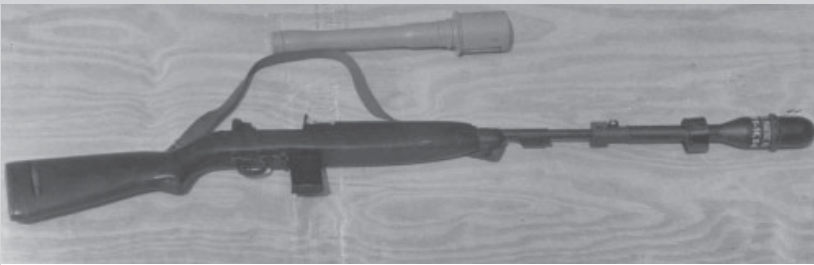
Two grenades. At top is a German "potato masher" hand grenade used in both World Wars. Below it is a rifle grenade fitted to a U.S. M 1 carbine.
