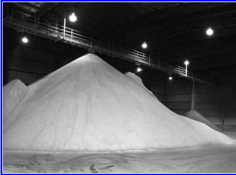
FIGURE 5.14 Distillers dried grains with solubles (DDGS) are most often piled into a flat storage building until cooled, at which time the DDGS will be transferred and loaded onto rail cars or semitrucks (photograph courtesy of USDA).
