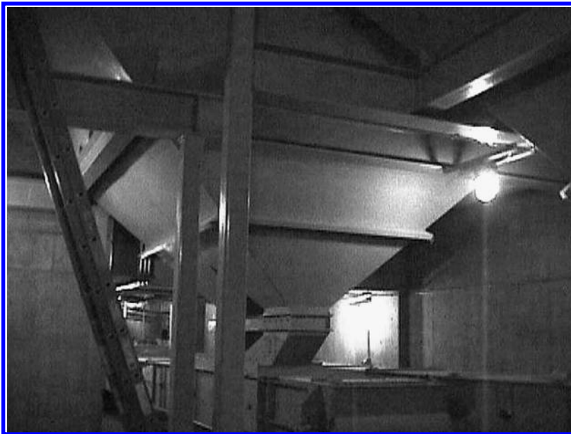
FIGURE 5.3 A below-ground grain receiving hopper accepts incoming corn by truck or rail, and then the corn is transferred to a bucket elevator by a drag conveyor (author's photograph).
