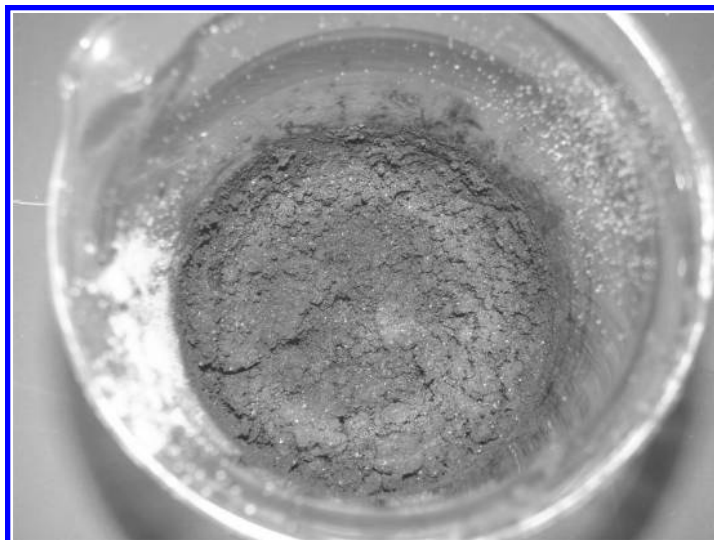
FIGURE 2.20 DDGS can be thermochemically converted into biochar, which can subsequently be used to produce energy, fertilizer, or as a precursor to other biobased materials (author's photograph).
