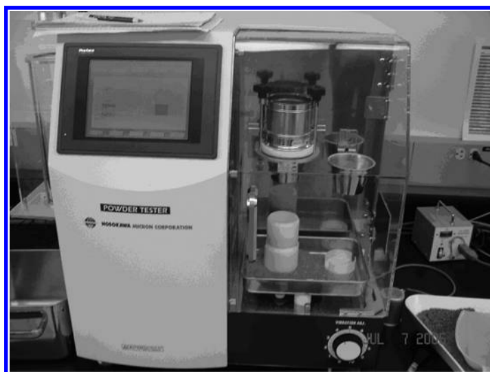
FIGURE 7.17 Typical semiautomated tester used to measure Carr indices (author's photograph).
