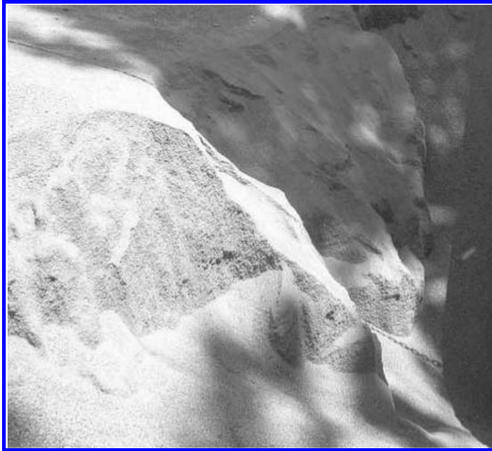
FIGURE 7.8 Flow of distillers grains is often problematic, due to caking and bridging between particles, which frequently occurs during storage and transport (author's photograph).
