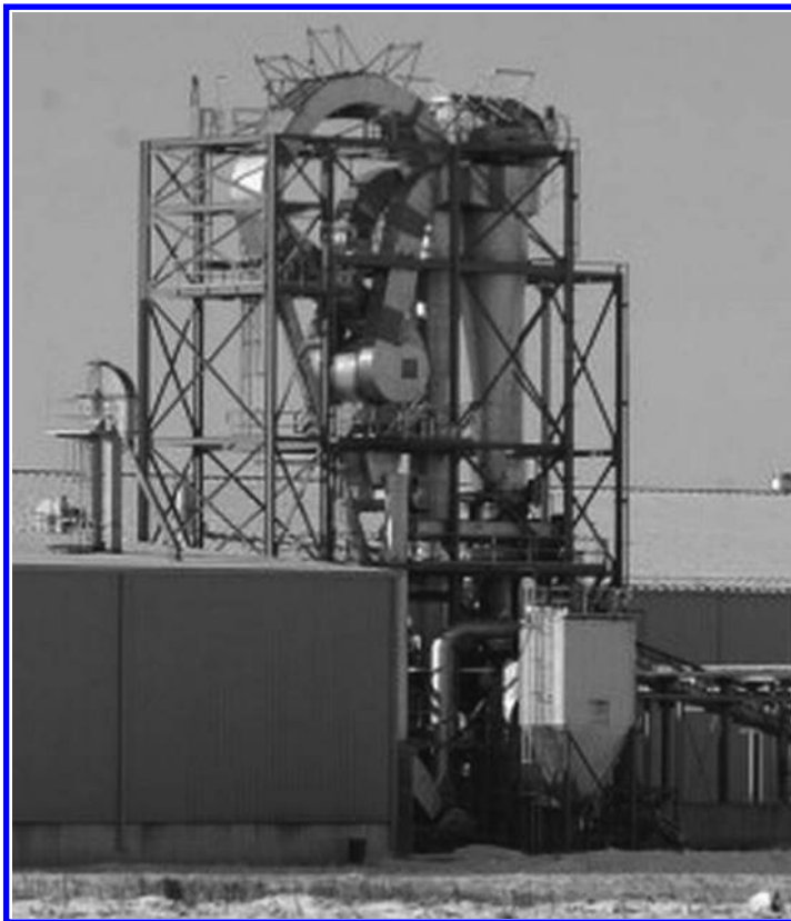
FIGURE 5.12 Ring dryers require a support tower, but encompass a smaller footprint than rotary dryers (author’s photograph).
