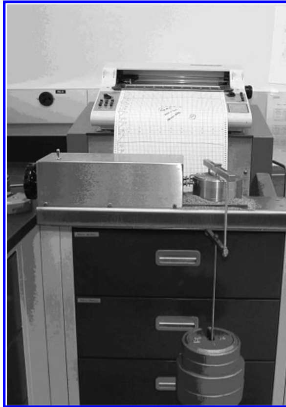
FIGURE 7.13 Typical Jenike shear tester setup (author's photograph).
