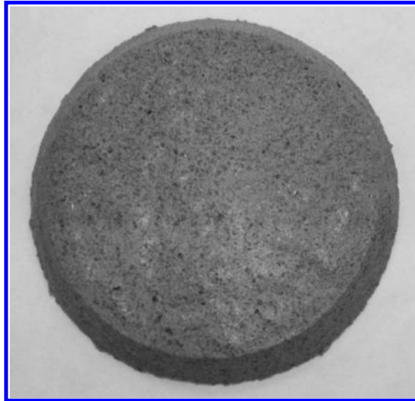
FIGURE 19.7 A 3 in (76 mm) diameter disk composed of 90% DDGS and 10% phenolic resin.
