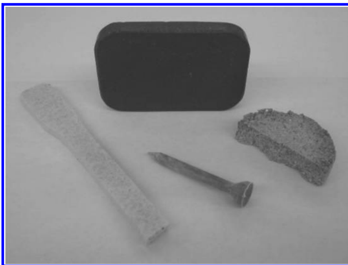
FIGURE 2.19 DDGS has been shown to be an effective filler in plastic products, replacing petroleum additives and increasing biodegradability (author's photograph).
