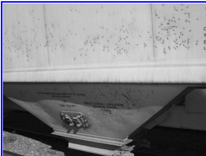
FIGURE 7.9 Transporting distillers grains can lead to substantial rail car damage due to flowability problems (when trying to unload product), because sledgehammers are often used to induce flow (author's photograph).
