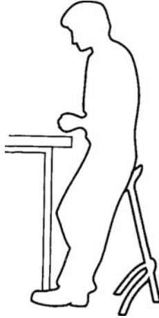
FIGURE 2.12 A pedestal stool can be used to change posture when standing for long periods.
