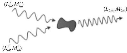
FIGURE 28.3 Scheme of SHG reporting the L and M quantum numbers that define the angular momentum and parity of the photons involved in the process.
