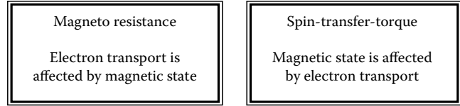
FIGURE 8.10 STT and GMR effects as dual mechanisms.
