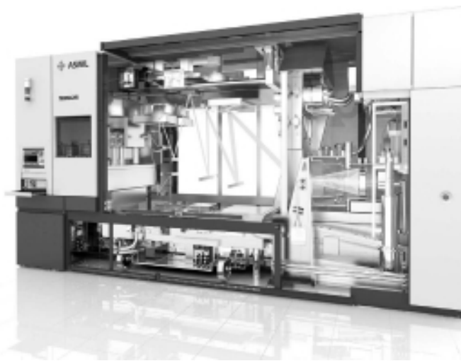
FIGURE 20.18 (See color insert following page 21-4.) Artist illustration of ASML NXE: 3100 preproduction EUV exposure tool showing the LPP EUV source on the right, the illuminator optics in the center, and the mask and the projection optics on the right. (Courtesy of ASML, Veldhoven, the Netherlands.)
