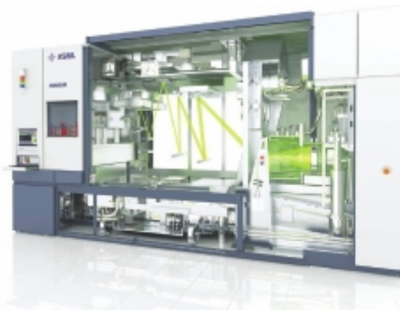
FIGURE 20.18 Artist illustration of ASML NXE: 3100 preproduction EUV exposure tool showing the LPP EUV source on the right, the illuminator optics in the center, and the mask and the projection optics on the right. (Courtesy of ASML, Veldhoven, the Netherlands.)
