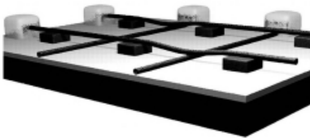
FIGURE 3.8 NRAM device made from a suspended nanotube device architecture with a three-dimensional view of a suspended crossbar array showing four junctions with two elements in the on state and two elements in the off state. The on state corresponds to nanotubes in contact and the off state to nanotubes separated. The substrate consists of a conducting layer (dark gray) that terminates in a thin dielectric layer (light gray). The lower nanotubes are supported directly on the dielectric film, whereas the upper nanotubes are suspended by periodic inorganic or organic supports (gray blocks). A metal electrode, represented by yellow blocks, contacts each nanotube. (Reprinted from Rueckes, T. et al., Science , 289(5476), 94, 2000. With permission.)
