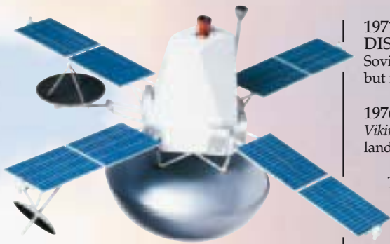
Viking spacecraft with solar panels and the metal capsule which contains the lander
