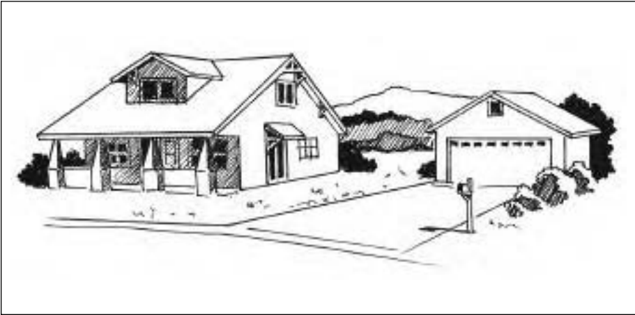
FIGURE 4.6—From an indoor air quality standpoint, a garage should be separate from the house; if that's not possible, the common walls must be extremely well-sealed.
