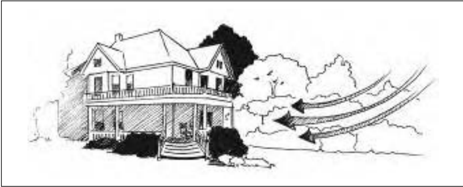
FIGURE 12.5— Well-planned landscaping can help to funnel summer breezes toward the house — allowing you to get by more of the time without air conditioning.
