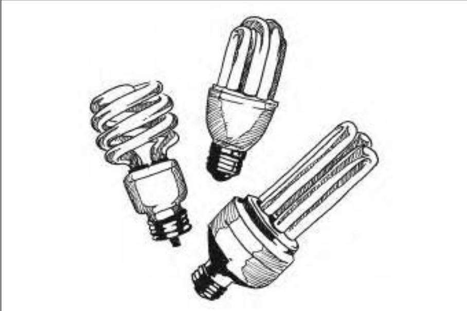
FIGURE 6.14—A wide range of compact fluorescent lamps is available, so there should be a product for most applications where incandescent lamps have been used. Products shown have integral ballasts and can be screwed into standard light bulb sockets.
