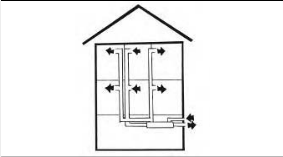
FIGURE 9.10—In a balanced ventilation system, incoming and outgoing airstreams balance one another. Heat in the outgoing airstream can be captured with an HRV or ERV.
