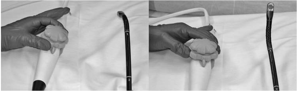
Figure 2 Anteflexion and retroflexion of the probe head is accomplished by rotation of the large knob on the TEE probe handle. Abbreviation: TEE, transesophageal echocardiography.
