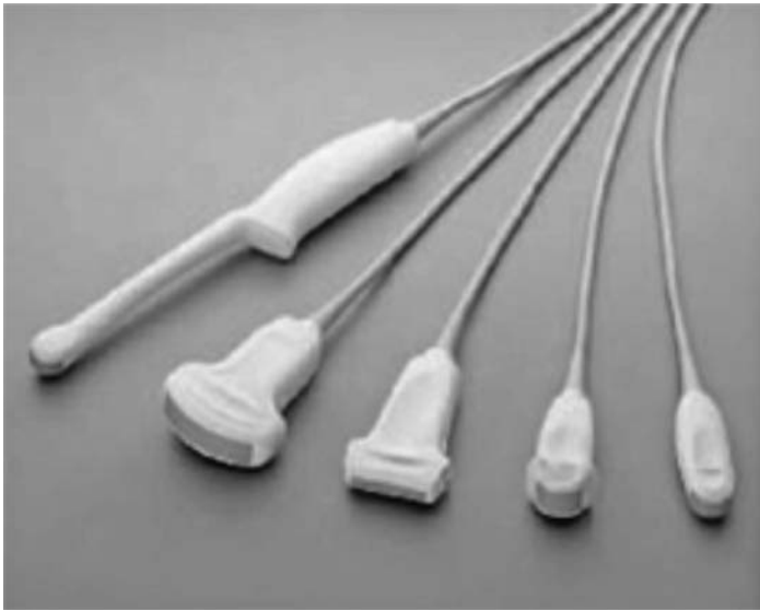
Figure 2 SonoSite probes; from left to right transvaginal, curved array larger footprint (abdominal/general), linear array (small parts/vascular), curved array small footprint (echocardiography), curved array small footprint (pediatric).
